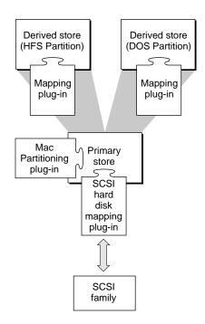
The bottom-most store in the figure is the primary store that maps to the SCSI hard disk. It has a SCSI hard disk mapping plug-in associated with it. The plug-in talks to the hard disk through the SCSI family. Because the store contains a Mac format partition map, the Apple-provided Mac partitioning plug-in is associated with it.
