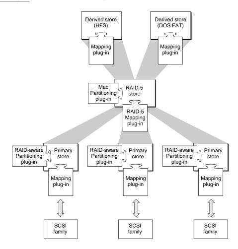
The RAID-5 driver is implemented as a mapping plug-in and is used at the derived store level. A RAID-aware partitioning plug-in stores the information needed by RAID-5 about its devices. The RAID-5 store is partitioned using the standard Mac partitioning format and contains an HFS and a DOS FAT partition, each of which results in a derived store.
