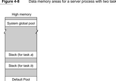
Figure 4-8 Data memory areas for a server process with two tasks
