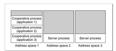
Figure 3-1 Copland processes and their address spaces
