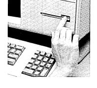
open the **Housekeeping** menu and choose **Eject "Diskette"**, or press simultaneously the Apple key and the letter *E*. To eject a micro diskette using other software, see the manual that comes with that software.
