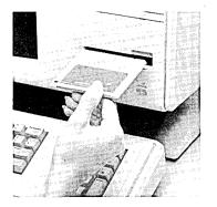
Push the diskette into the micro disk drive until it clicks into place. When the diskette is in place, you can hear the micro disk drive clamp onto the diskette. Once a diskette is in place and clamped, do not try to pull it out.
