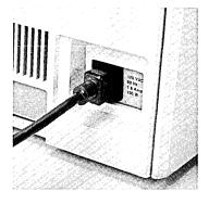
When you must unplug the Lisa, make sure the light in the on-off button is off before you pull the plug.
