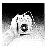
c. Pressing down on the ring, turn it clockwise 45 degrees until the marker lines up with the *L* (for *Locked*) on the mouse case.
