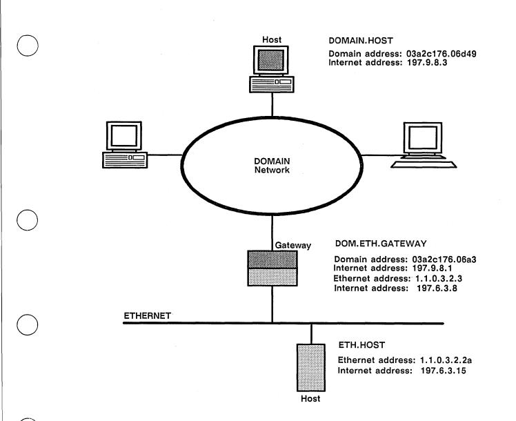
Figure A-2. Network Configuration that Illustrates Sending Packets
