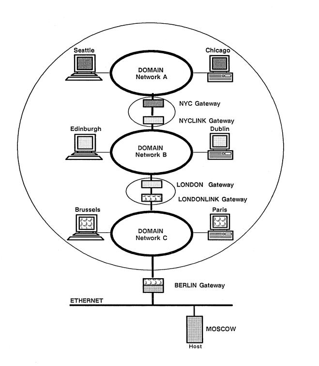
Figure 2-4. TCP/IP Configuration for DOMAIN Internet with Subnet Numbers
