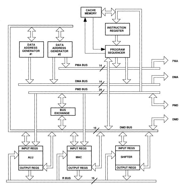
Figure 1.2 ADSP-2100 Internal Architecture
