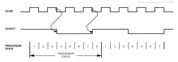
Figure 5.2 Clock Signals & Processor States
