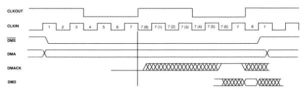
Figure 5.7 Data Memory Read Extended by DMACK
