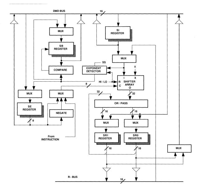
Figure 2.7 Shifter Block Diagram
