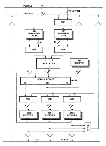
Figure 2.5 Multiplier/Accumulator Block Diagram
