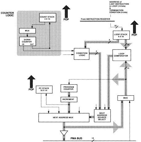
Figure 4.6E DO UNTIL: Final Iteration
