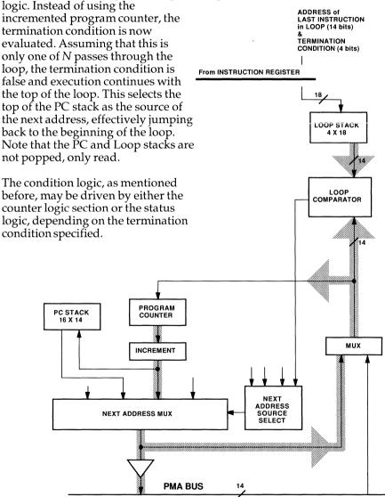
Figure 4.6D DO UNTIL: End of One Iteration
