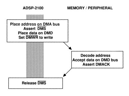
Figure 5.9 Data Memory Write Flowchart
