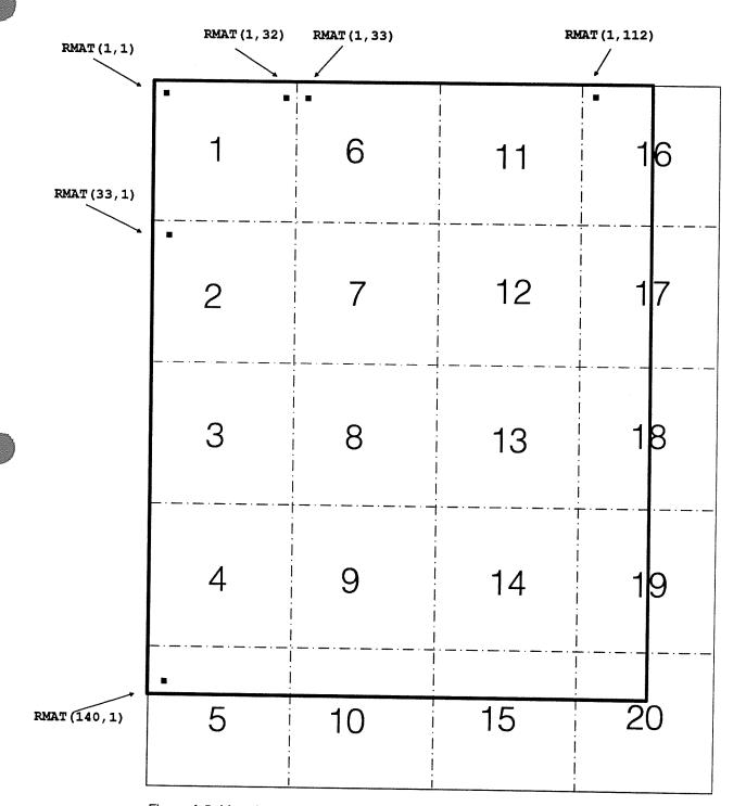
Figure A.5: Mapping of **REAL RMAT (\*140, \*112)** on a DAP 500(32 x 32 PEs)
