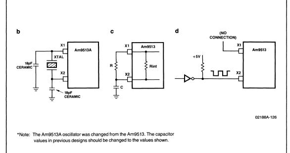
Figure 11-1.5b, c, d Driving the X1 and X2 Inputs
