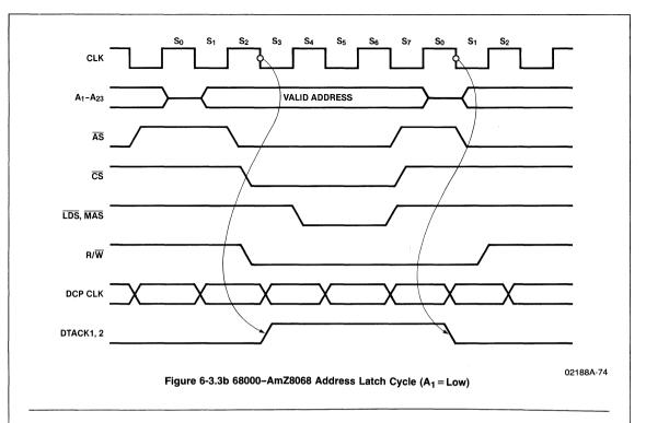
An address decoder generates the Chip Select for the DCP. The Address Strobe indicates a valid address. The PAL device is only activated if the Lower Data Strobe becomes active while the Upper Data Strobe stays inactive. This means that data is transferred in MOVE.B instructions with an odd peripheral address.
