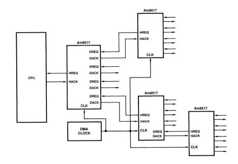
Note: All Am9517A devices must use common clock in Cascade mode.
