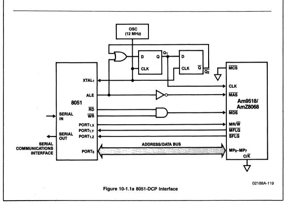
CPU is to execute "MOVX" instructions, every second ALE is left out and the divide factor is four. For both cases the minimum DCP clock High or Low width is two CPU clock periods, which guarantees that even a CPU clock of 12 MHz satisfies the minimum clock requirement for the Am9518 as well as the AmZ8068.
