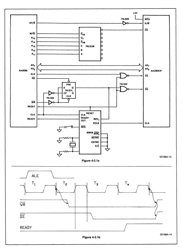
A 74LS74 is used to delay the falling edge of  $\overline{WR}$ ;  $\overline{RD}$  is ORed with  $\overline{WR}$  by the flip-flop which takes the advantage of the preset overriding clear. By using the asynchronous ready mode of the 8284A, one Wait State is inserted in both the read and write cycles. This stretches  $\overline{DS}$  to meet the minimum pulse width requirements.
