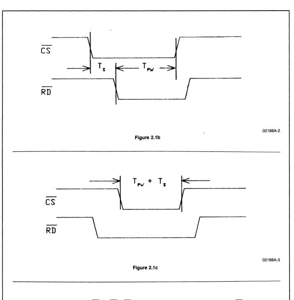
Note that it is often assumed that  $\overline{CS}$  and  $\overline{RD}$  or  $\overline{CS}$  and  $\overline{WR}$  are simply gated together. This is true for most peripherals but not in all cases. Check the manufacturer's specification. It is often possible to implement and simplify the design but manufacturers do not guarantee operation in these unusual modes.
