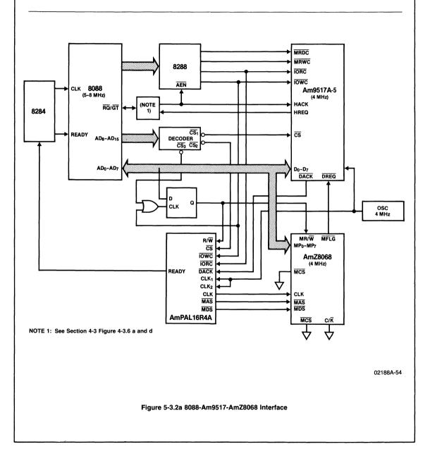
Before executing an access to the DCP, the CPU must latch the MR/ $\overline{W}$ . The transfer itself is evaluated in a two-cycle operation.
