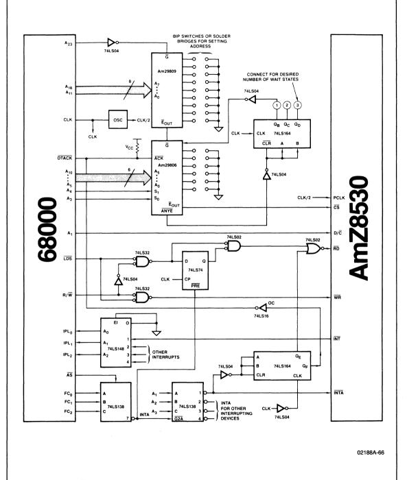
Figure 6-2.2a Am8530 to 68000 Connection with Interrupts Using SSI and MSI
