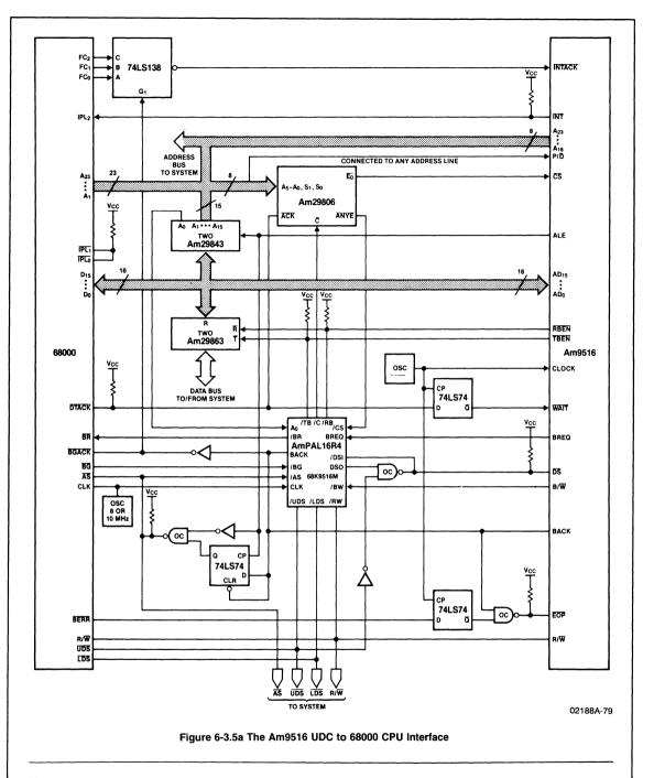
Note that the address latch and data transceiver, along with the address decode logic, are present in any case. The 68450 and 68440 also multiplex address and data, thus the PAL device is the only extra component required to make the 9516 a low cost alternative. Additionally, the 6 MHz 9516 has the same data throughput as the 8 MHz 68450.
