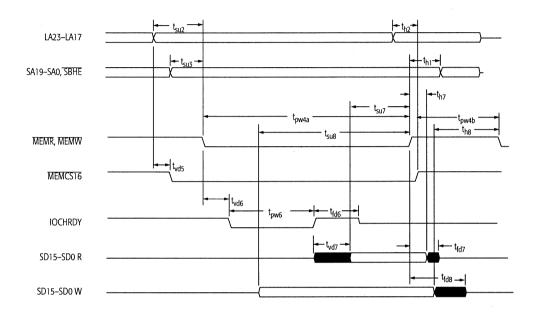
Figure 9-6. ISA Master-to-PCI Access Timing
