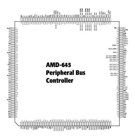
Figure 11-1. AMD-645 Peripheral Bus Controller Pin Diagram
