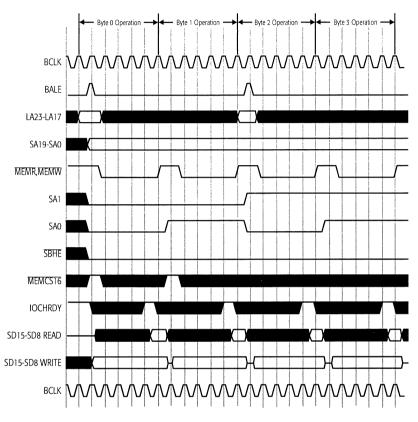
Figure 5-10. ROM Cycle 32-Bit to 8-Bit Conversion
