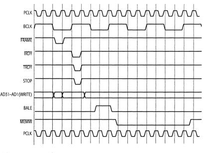
Figure 5-4. Posted PCI-to-Memory Write
