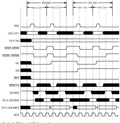
Figure 5-8. Memory Cycle 32-Bit to 16-Bit Conversion
