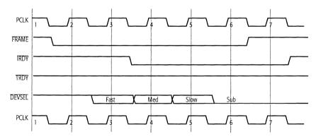
Figure 5-13. Subtractive Decode Timing
