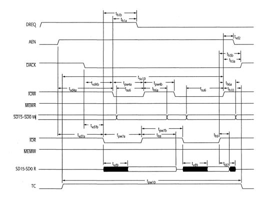
Figure 9-10. Type F DMA Interface Timing
