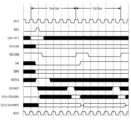
Figure 5-2. I/O Cycle 16-Bit to 8-Bit Conversion
