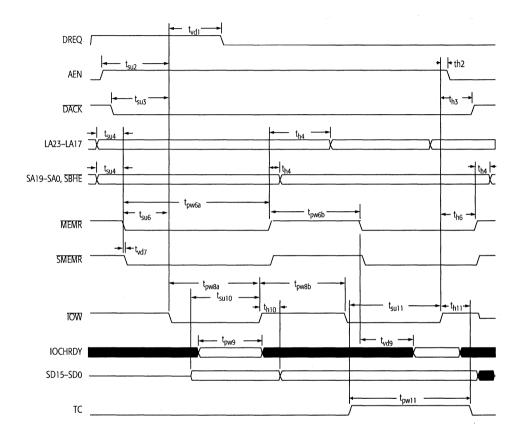
Figure 9-8. DMA Read Cycle Timing
