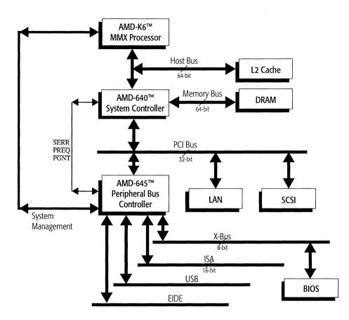
Figure 1-1. AMD-640 Chipset System Block Diagram
