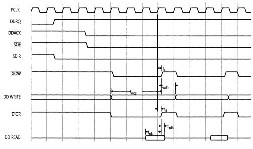
Figure 5-28. IDE Multiword DMA Cycle
