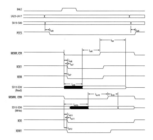
Figure 9-11. X-Bus Interface Timing
