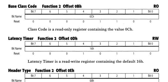
Header Type is a read-only register containing the value 00h.
