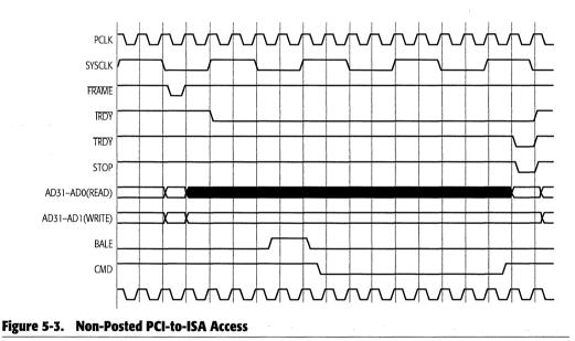
If the AMD-645 Peripheral Bus Controller is unable to complete the initial data phase within the required initial latency, it begins a delayed transaction and terminates with retry by asserting STOP without asserting TRDY at the end of the initial data phase. If the next data phase in a burst cannot be completed within the required incremental latency, the AMD-645 Peripheral Bus Controller disconnects by asserting TRDY and STOP at the end of the current data phase.
