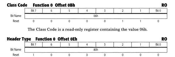
The Header Type is a read-only register containing the value 80h.
