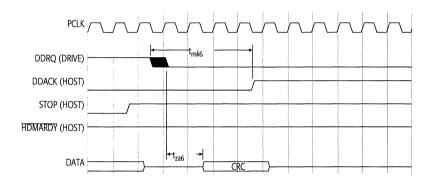
Figure 5-23. Host Terminating DMA Burst During Read Command
