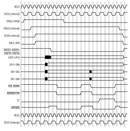
Figure 5-14. DMA Transfer Cycle
