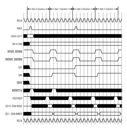
Figure 5-7. Memory Cycle 32-Bit to 8-Bit Conversion
