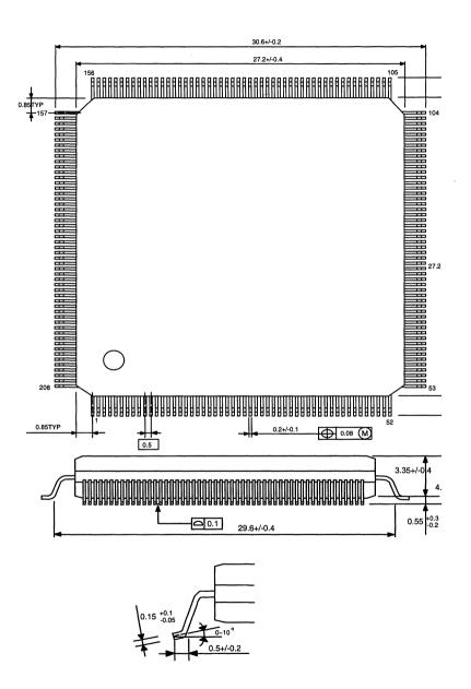
Figure 12-1. 208-Pin Plastic Quad Flat Pack Outline Drawing
