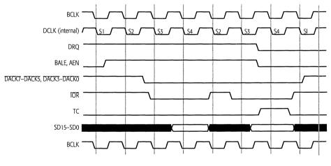
Figure 5-18. Type F DMA Timing
