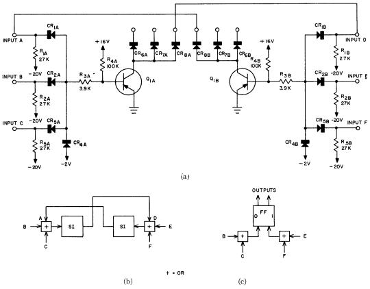
Fig. 12—(a) Basic flip-flop schematic diagram, (b) single inverters connected as flip-flop, (c) flip-flop block diagram.
