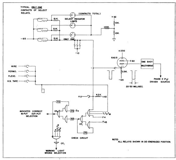
Fig. 3-Logical diagram-typical "only one" circuit.
