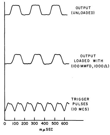
Fig. 9-Flip-flop waveforms.
