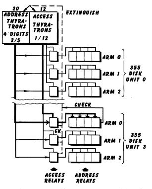
Fig. 11-Seek: Transfer address from 652 to 355 address relays.
