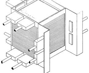
Fig. 4—"T" memory, 4096 words, 37 digits,  $4\frac{5}{8} \times 4\frac{5}{8} \times 5$  inches inside the brackets.
