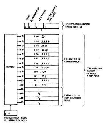
Fig. 7—TX-2 configuration selection. The cf digits select a configuration for the computer for use during the execution of the instruction.
