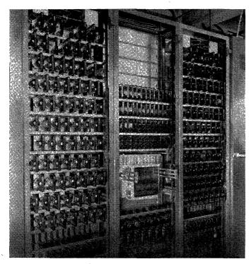
Fig. 7-Error matrix under test.
