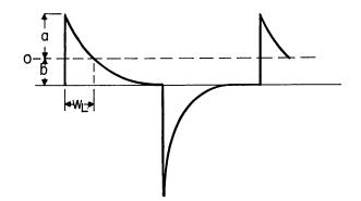
Fig. 8—Base current waveform of the main transistor switch in the logarithmic circuit.
