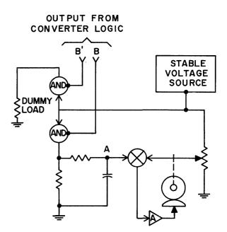
Fig. 9—Digit-to-voltage or shaft-position converter.
