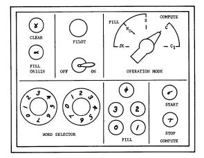
Fig. 5-Sketch of control panel.
