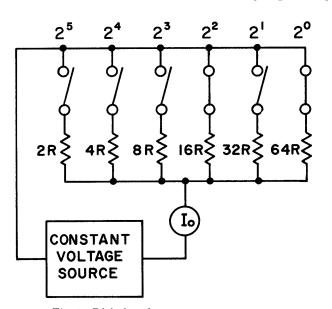
Fig. 1-Digital-analog current converter.
