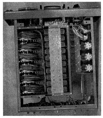
Fig. 3-Internal view of the A14 side control panel.
