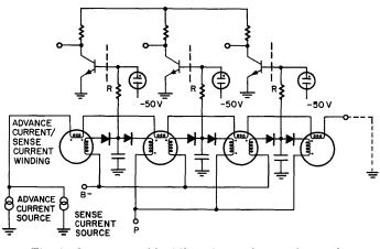
Fig. 6—One-core-per-bit shift register using nondestructive read-out to provide permanent output.
