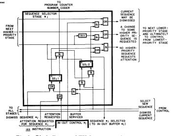
Fig. 2-Block diagram of TX-2 sequence selector stage.
