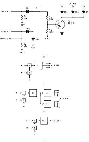
Fig. 11—(a) Basic single inverter circuit, (b) single inverter block diagram, (c) single inverter connected for double inversion, (d) double inverter diagram.
