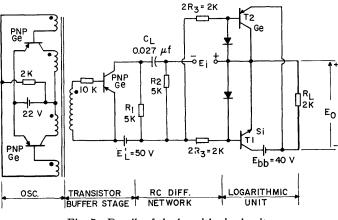
Fig. 7-Details of the logarithmic circuit.
