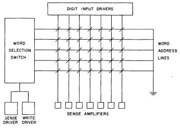
Fig. 7—Parallel-digit memory suited for magnetic inertia operation.
