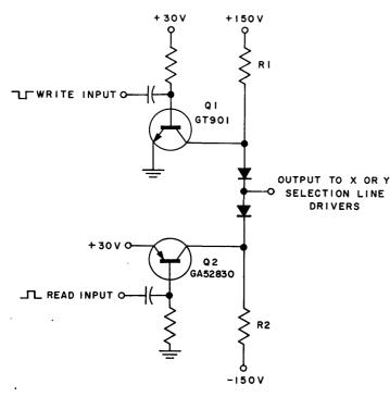
Fig. 8-Read-write driver (2 needed), "T" memory.
