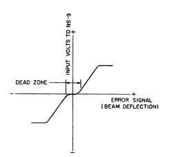
Fig. 5-Input to phase-detector amplifier.
