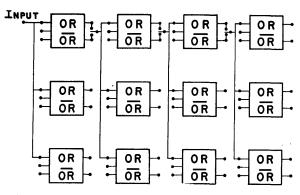
Fig. 9—Block diagram of four complemented OR circuits in sequence, with a cascading factor of three.
