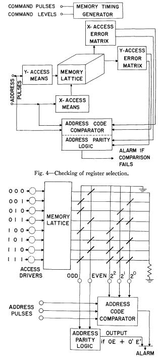
Fig. 5—Error-matrix and comparison logic for one access dimension.
