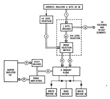
Fig. 15-Block diagram, "X" memory.
