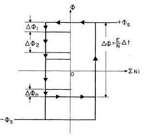
Fig. 5-Magnetic characteristic of rectangular hysteresis loop core material.
