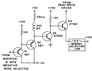
Fig. 7-One channel, selection line driver, "T" memory.
