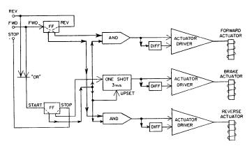
Fig. 8-Simplified tape-control logic.
