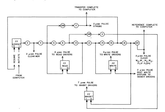
Fig. 8-Simplified block diagram of memory timing chain.
