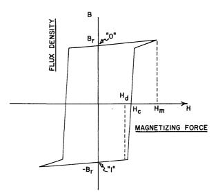
Fig. 1-Hysteresis characteristic of memory core.
