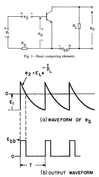
Fig. 2-Waveforms pertinent to logarithmic circuit.
