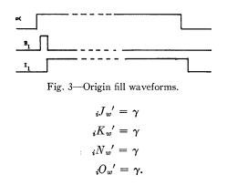
The origin is then indicated by four simultaneous ones in  $J_1$ ,  $K_1$ ,  $N_1$ , and  $O_1$ .
