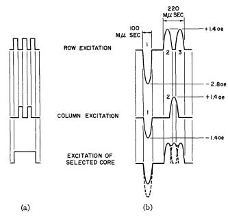
Fig. 8—Pulse interlace waveforms for writing into two-dimensional core matrices.(a) For use in serial digit arrays. (e.g., Fig. 9).
