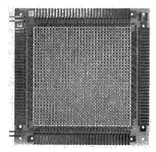
Fig. 2-Magnetic-core matrix.
