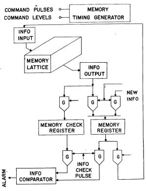
Fig. 10-Checking of information insertion.
