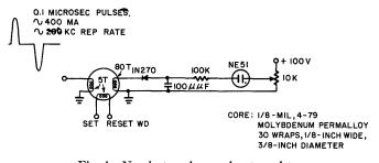
Fig. 4—Nondestructive read-out used to operate neon indicator.
