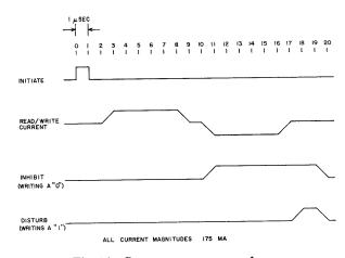
Fig. 16-Current generator waveforms.
