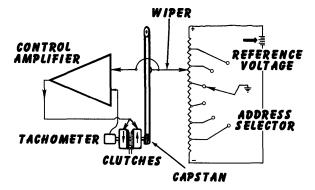
Fig. 13-Electrical portion of arm-servo (simplified).
