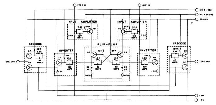
Fig. 8-TX-2 flip-flop.
