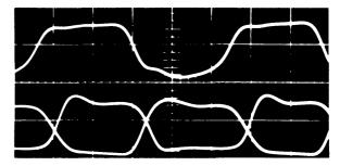
Fig. 6—Three-way complemented OR circuit. Two inputs are logical ZERO's, third input is the top waveform. Lower waveforms are outputs. (Hor.: 20 musec/cm, vert.: 1 volt/cm.)
