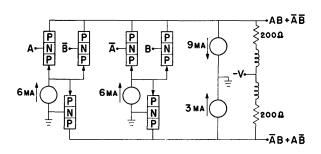
Fig. 11-Six-transistor, complemented, exclusive OR circuit.
