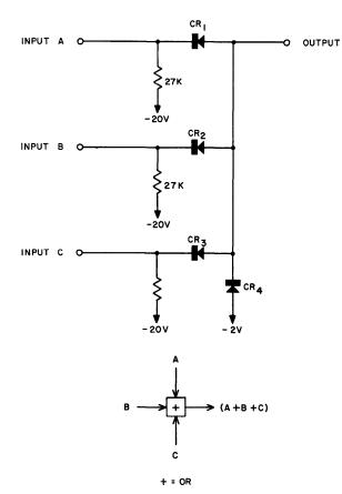
Fig. 10-Basic logical OR circuit and symbol.
