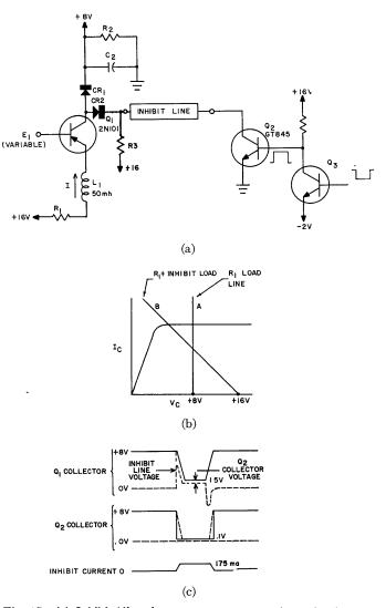
Fig. 17—(a) Inhibit/disturb current generator schematic diagram<sup>•</sup> (b) transistor Q, collector characteristics, (c) inhibit/disturb current generator voltage waveforms.
