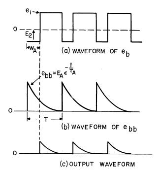
Fig. 3-Waveforms pertinent to antilogarithmic circuit.
