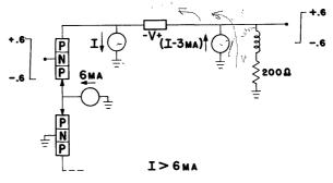
Fig. 4—Application of a voltage translating block as a means of coupling.
