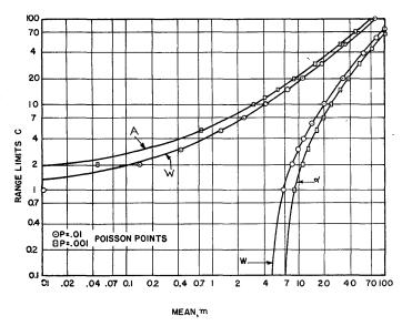
Fig. 3—Poisson cumulative curves of range limits, C, vs mean, m. The four curves represent the probability limits A = 1/1000, W = 1/100, w = -1/100, and  $\alpha = -1/1000$ .
