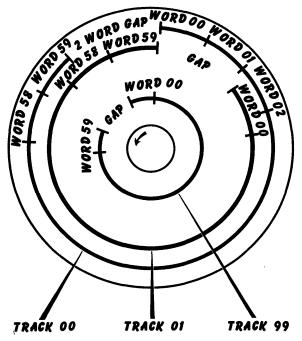
Fig. 6-Track and word arrangement on a disk face.
