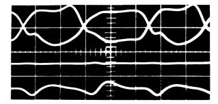
Fig. 7—Three-way complemented OR circuit. One input is a logical ZERO, top waveforms are two complementary inputs. Center waveform is AND output. Lower waveform is OR output. (Hor.: 20 musec/cm, vert.: 1 volt/cm.)
