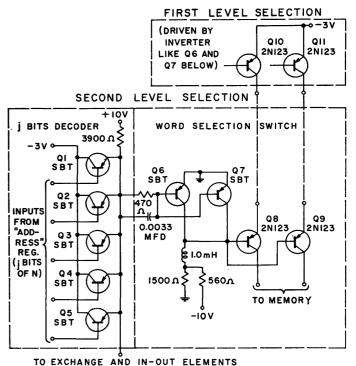
Fig. 16-Register selection circuit, "X" memory.
