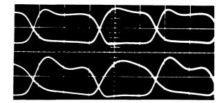
Fig. 8—Outputs of a ten-way complemented OR circuit, lower waveforms, compared with the outputs of a three-way complemented OR circuit, upper waveforms, driven by the same input signal. (Hor.: 20 musec/cm, vert.: 1 volt/cm.)
