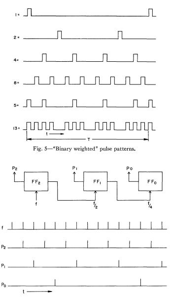
Fig. 6-Logic and timing diagram. Binary related pulse generation.
