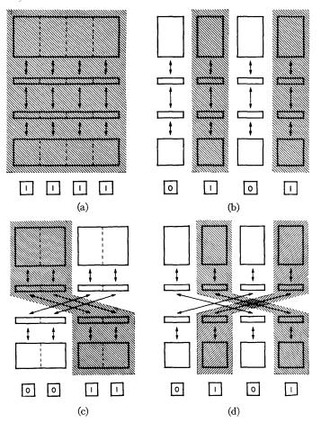
Fig. 10—Illustrative example of different configurations. Areas of activity during execution of instruction are shown shaded. Effects of AE coupling are shown by juxtaposition. (a) (P0, 36) configuration. (b) (P0, 9, 9, 9, 9) configuration. (c) (P2, 18, 18) configuration. (d) (P2, 9, 9, 9, 9) configuration.
