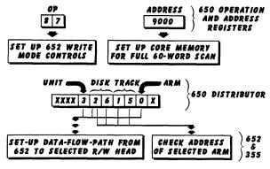
Fig. 15-Write flow path setup and address-check.
