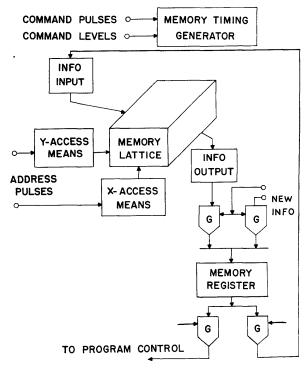
Fig. 3-Block diagram of core memory.
