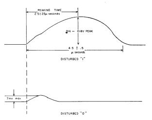
Fig. 3-Memory-core output signals.
