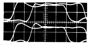
Fig. 10—Input and output waveforms of four sequential three-way complemented OR circuits with a cascading factor of three. Top waveforms are input and output of the system with blocks connected through inverted outputs. Lower waveforms are with the blocks connected through noninverted outputs. (Hor.: 20 musec/ cm, vert.: 1 volt/cm.)
