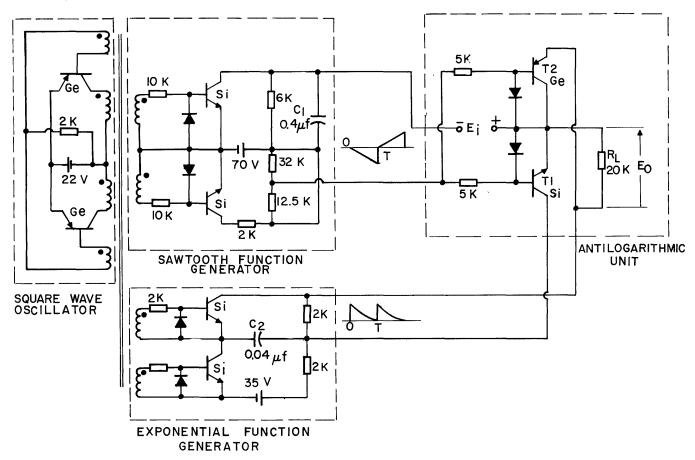
Fig. 10—Details of the antilogarithmic circuit.
