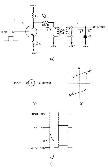
Fig. 6—(a) Magnetic-core timing-delay schematic diagram, (b) magnetic-core timing-delay block diagram, (c) magnetic-core hysteresis loop, (d) magnetic-core timing-delay voltage waveforms.
