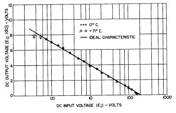
Fig. 9—Steady-state temperature characteristic of the logarithmic circuit.
