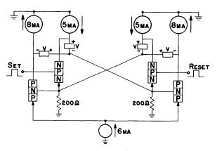
Fig. 14—A typical trigger circuit for use in set and reset operation using *n-p-n* emitter followers for pullover.
