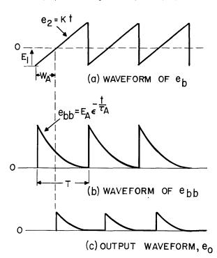
Fig. 4-Waveforms for an alternate antilogarithmic circuit.
