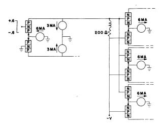
Fig. 3—A p-n-p block driving a number of remote n-p-n blocks.
