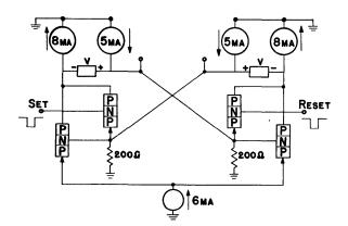
Fig. 13—A typical trigger circuit for use in set and reset operation using p-n-p emitter followers for pullover.
