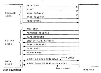
Fig. 4-Control lines for RCA Bizmac Tapefile.
