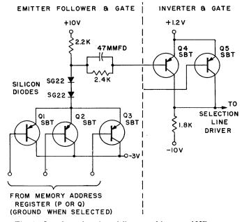
Fig. 6—One channel, emitter follower and inverter AND gates, "T" memory.
