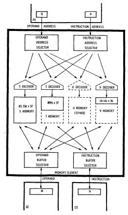
Fig. 2—TX-2 Memory Element. Two address and two buffer registers are used to permit simultaneous operation of any two of the four memories.
