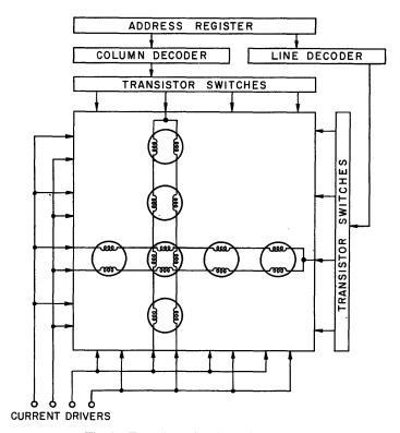
Fig. 9-Two-dimensional inertia memory.
