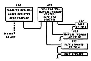
Fig. 3-650 RAMAC (basic 650 not shown).
