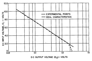
Fig. 11—Steady-state characteristic of the antilogarithmic circuit.
