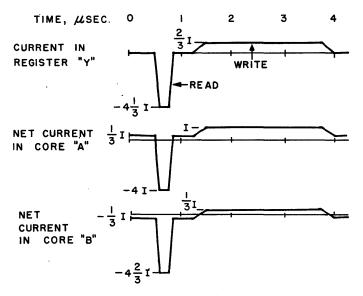
Fig. 12-Timing diagram, "X" memory.
