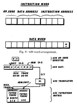
Fig. 10-Seek: transfer disk-memory address from 650 to 652.
