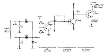
Fig. 15-Current diverter schematic diagram.
