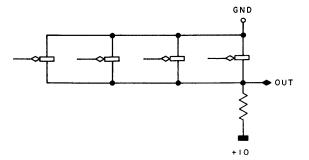
Fig. 4-Parallel inverters.
