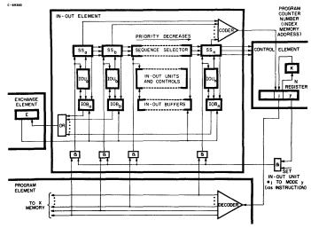
Fig. 1-Block diagram of TX-2 in-out element.
