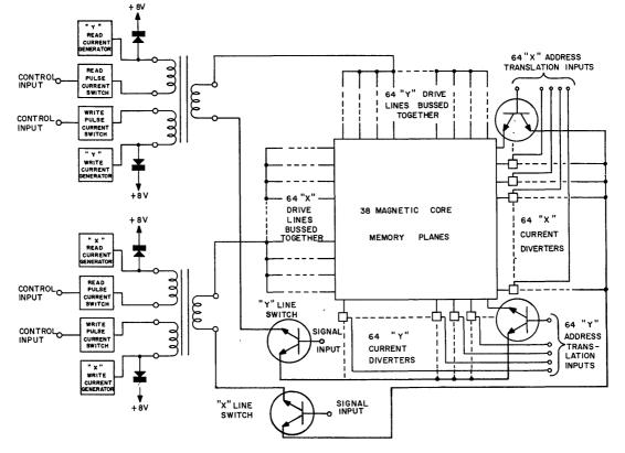
Fig. 18-Simplified diagram of "X" and "Y" drive line and current diverter system.
