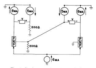
Fig. 12-Simple two-transistor trigger or flip-flop.
