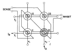
Fig. 2-Planar array of memory cores.
