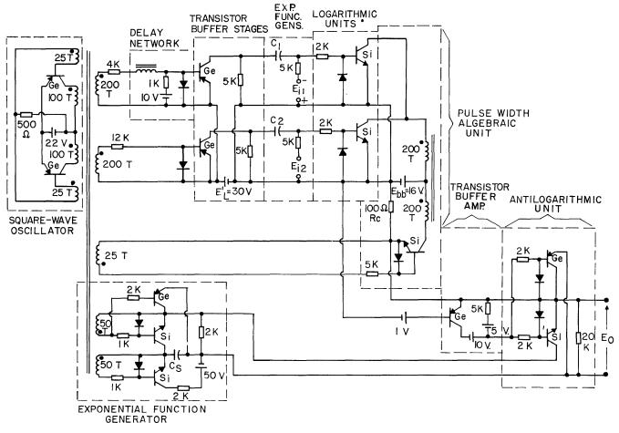
Fig. 12-Ensemble circuit.
