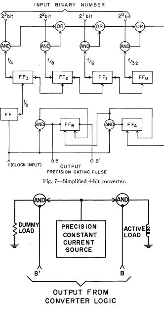
Fig. 8-Constant-current pulse generator.
