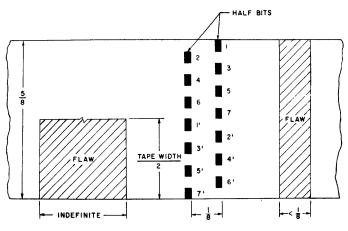
Fig. 5-Seven-bit dual-channel configuration.
