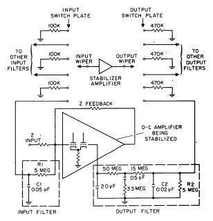
Fig. 2-Major parts of drift-stabilization system.
