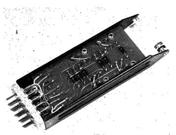
Fig. 17-TX-2 plug-in unit.
