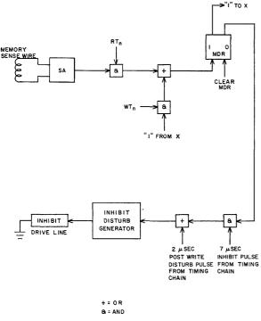
Fig. 13-Logical block diagram of restoration circuit.
