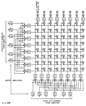
Fig. 14—Simplified block diagram of translator.
