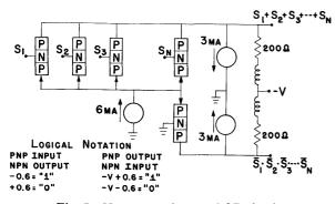
Fig. 5-N-way complemented OR circuit.
