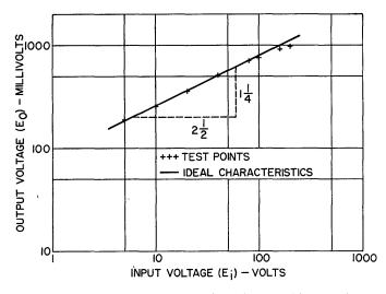
Fig. 14—Steady-state characteristic of the ensemble operating as a square-rooter.
