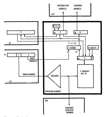
Fig. 4—TX-2 Program Element, determining the instruction and operand memory addresses, performing X memory operations.
