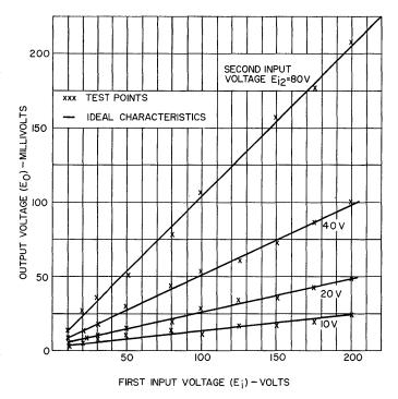
Fig. 13—Steady-state characteristic of the ensemble operating as a multiplier.
