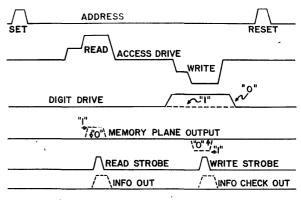
Fig. 9-Memory-timing diagram.
