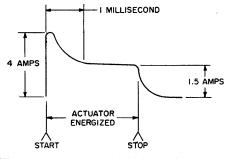
Fig. 9-Input current for high-speed actuators.
