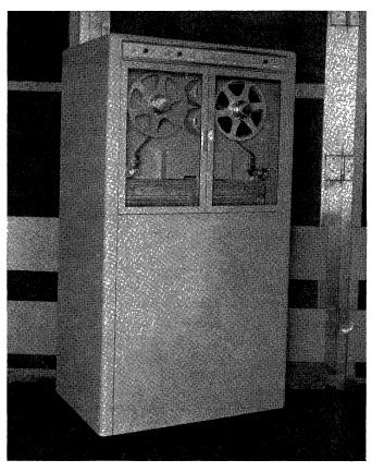
Fig. 1-Tape Transport equipment.
