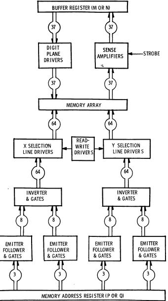
Fig. 5-Block diagram, "T" memory.
