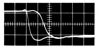
Fig. 16—Input and output waveforms of three sequential triggers using alternate p-n-p and n-p-n emitter followers as pull-over transistors. The inverted output signals were used for coupling. (Hor.: 20 musec/cm, vert.: 0.5 volt/cm.)
