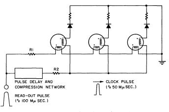
Fig. 5—Application of nondestructive read-out to current steering switch.
