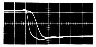
Fig. 15—Input and output waveforms of three sequential triggers
