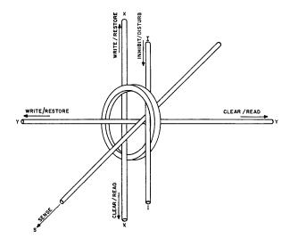
Fig. 4—Magnetic-core control wires. Arrows indicate direction current flow during reading or writing.
