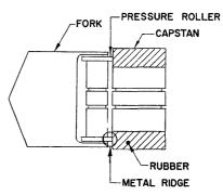
Fig. 3-Plan view of pressure roller and capstan.
