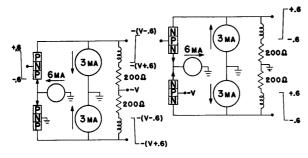
Fig. 2-N-P-N and p-n-p basic transistor blocks with input and output levels shown to illustrate compatibility.
