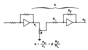
Fig. 1—Elements involved in determining the over-all gain of a computer amplifier.
