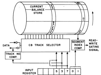
Fig. 3. Addressing method for "current balance" section of drum
