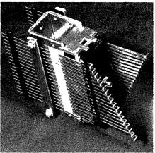
Fig. 7. Wire spring relay
