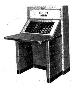
Fig. 10. Operator-verifier console
