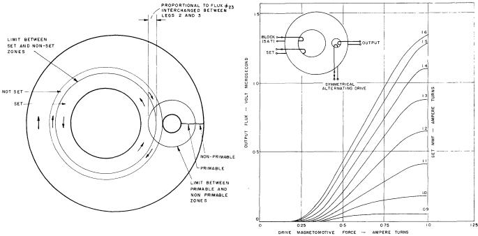
Fig. 8. Zones of setting and primability in the transfluxor
