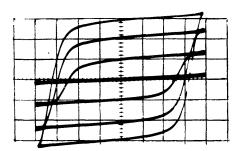
Fig. 10. Hysteresis loops of the output magnetic circuit for various settings
