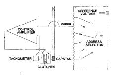
Fig. 4. Electrical functional schematic
