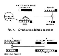
Fig. 5. The computation of y = ax + binvolving decimal points
