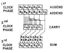
Fig. 7. 5-bit parallel binary adder
