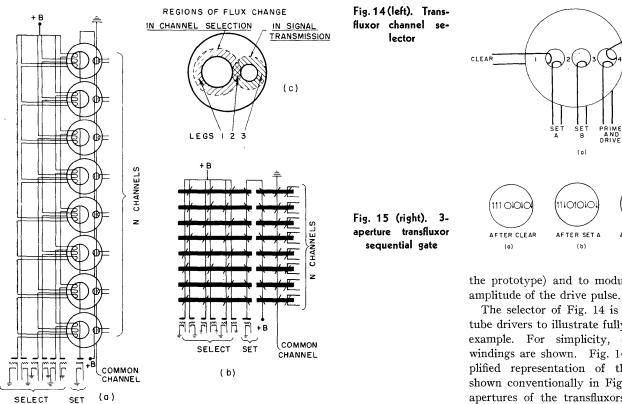
number of selectable channels is controlled by a transfluxor. All transfluxors are blocked except one which is set and which determines the selected channel.
