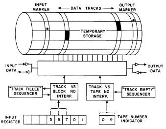
Fig. 4. Addressing method for "temporary storage" section of drum
