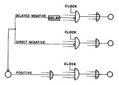
Fig. 5. Use of negative signals for inhibiting
