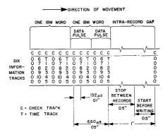
Fig. 3. Output tape format. This figure illustrates format for two channels of data. "1" is the most significant digit of a number; "10" is the least significant. The third row except for check track contains zeros in all cases
