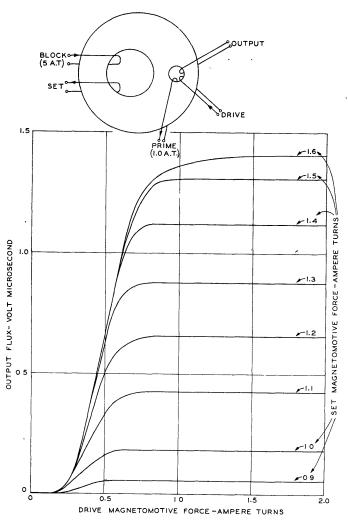
Fig. 6. Driving characteristic—asymmetrical energization
