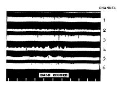
Fig. 3. Dash record. Vertical lines along bottom edge are time marks
