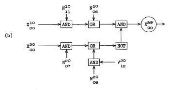
Fig. 1. Typical logical equation with diagrammatic representation
