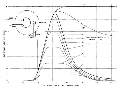
Fig. 5. Setting characteristic—asymmetrical energization
