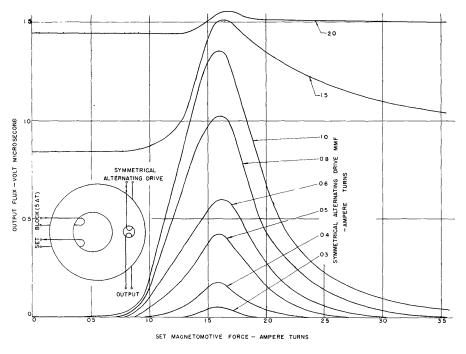
Fig. 7. Setting characteristic—symmetrical energization
