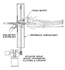
Fig. 3. Mechanical functional schematic
