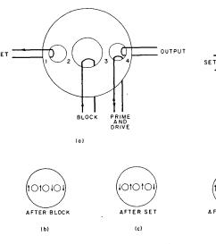
Fig. 17. Elimination of oversetting with an additional aperture
