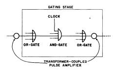
Fig. 1. One stage of SEAC-type circuitry
