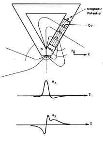
Fig. 3. Field plot showing influence of coil location on  $H_x$  and  $H_y$
