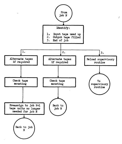
Fig. 2. Supervisory routine: between-tape operations
