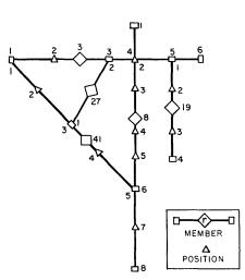
Fig. 3. Example of representation of a closed structure
