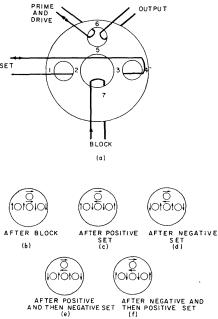
Fig. 18. Setting with a pulse of either polarity
