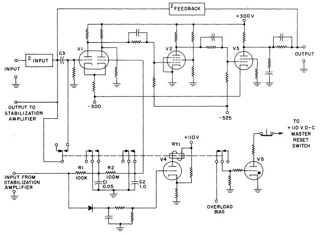
Fig. 4. Computing-amplifier unit
