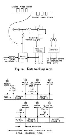
Fig. 6. Data arrangement on intermediate tapes. Note: Numbers in circles indicate sequence of events in time
