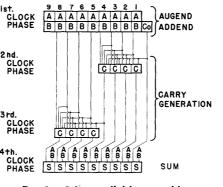
Fig. 8. 9-bit parallel binary adder
