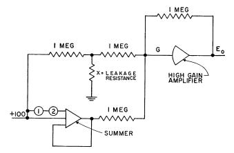
Fig. 4—Circuit for measuring interconsole leakage resistance.
