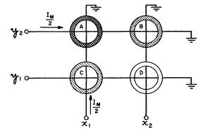
Fig. 2-Two-co ordinate array.
