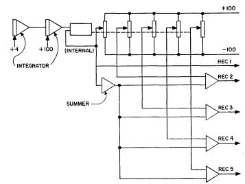
Fig. 3—Circuit used for checking servo-multiplying potentiometers with followup potentiometer as standard.
