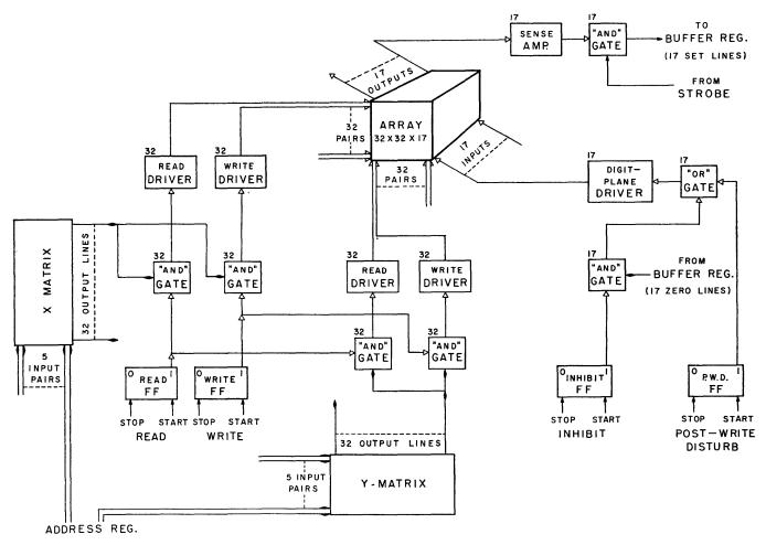
Fig. 5-Memory block schematic.
