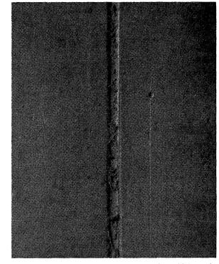
Fig. 2—Showing a streak in the magnetic coating which results in a deficiency of magnetic oxide along the streak (magnified 50 times).
