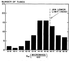
Fig.  $3-G_m$  distribution of 6SK7 removals from land-based communications receivers.
