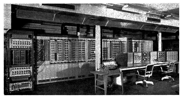
Fig. 10-Memory installation in MTC.
