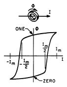
Fig. 1-Flux-current characteristic of ferrite toroid.
