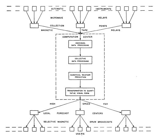
Fig. 4—A flow diagram of meteorological information in a possible system for data processing. The role of small-scale forecasting, extended-range forecasting, and climatological uses is not included.
