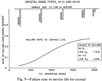
Fig. 9—Failure rate vs service life for crysta diode types 1N111 and 1N112.
