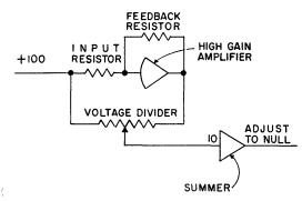
Fig. 2-Amplifier gain calibration circuit.
