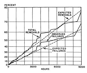
Fig. 11-Tube mortality with time, shipborne equipments.
