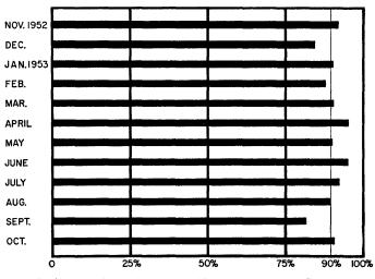
Fig. 7—Monthly reliability coefficients for Project Cyclone Simulation Laboratory (average for first year 90.6 per cent).
