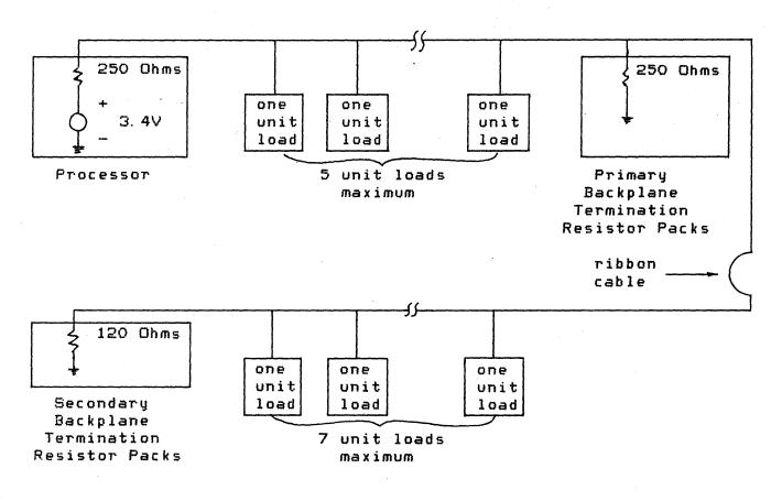
Figure 5.8.2 Bus Terminations for System with Primary and Secondary Backplanes
