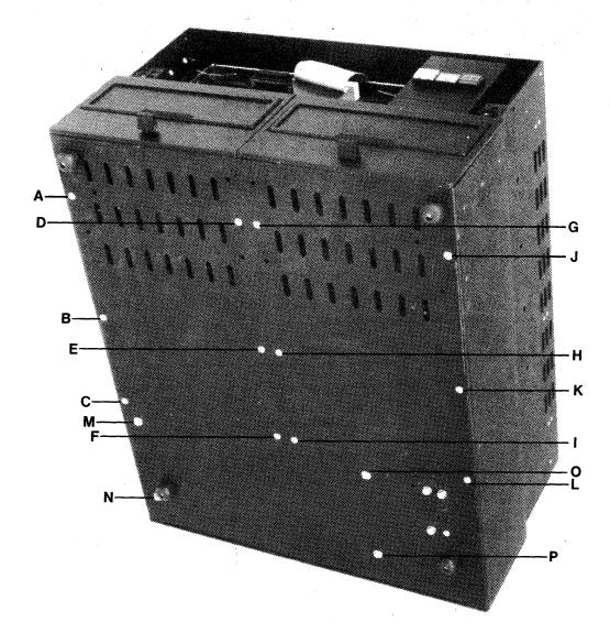
A-F) Screws for Floppy Drive Unit #0 G-L) Screws for Floppy Drive Unit #1 M-P) Screws for Primary Power Supply
