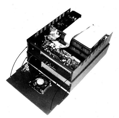
Figure 3.3.1 Removing the Rear Panel
