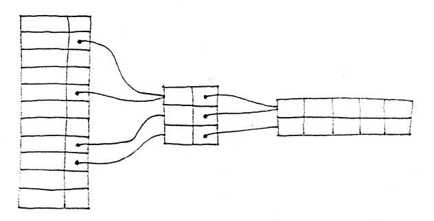
host2dli: host number to data link instance dli2dlty: data link instance to data link type dlty2dlsw: data link type to data link switch
