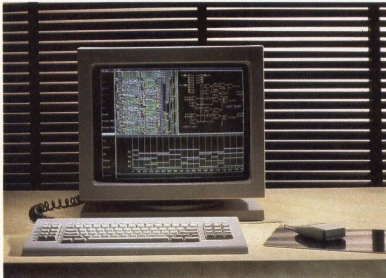
Sun Microsystems' Sun-4/200 workstation, based on Sun's SPARC microprocessor, delivers performance comparable to DEC's VAX 8700.
