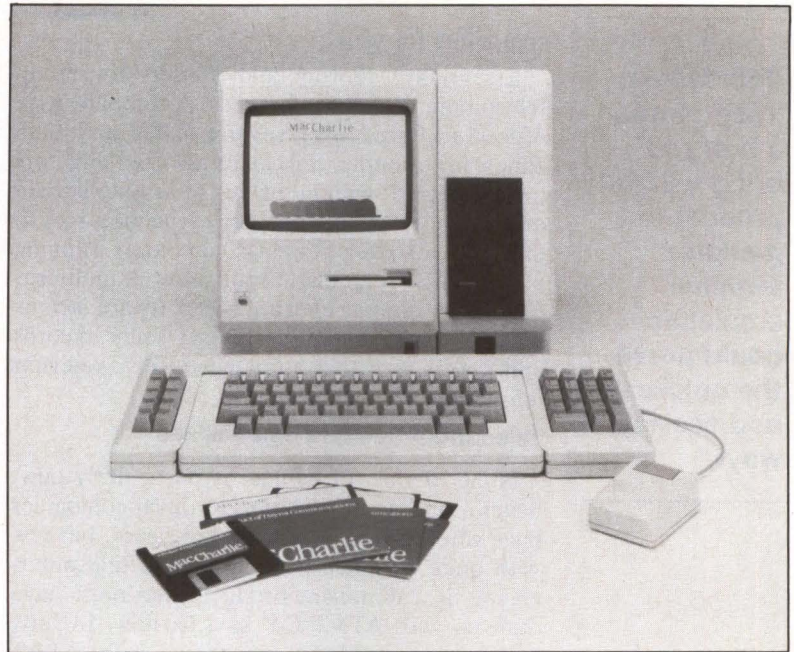
A novel use of ASCII, Dayna's MacCharlie links the Apple Macintosh to an IBM PC-compatible microcomputer. The bridge between the two systems is Dayna's communications software.
