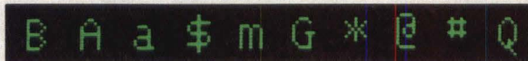
The sharp 8 x 16 character matrix helps make for easier reading and fewer operator errors.
