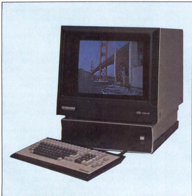
Supporting 1,024-by-780-pixel displays with six planes of colors, Intecolor's series has 250K bytes of display list plus DMA interface for $4,995.
