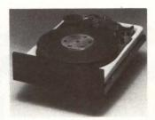
closed-loop servo positioning system. With a track density of 720 tpi, the drive stores 20M bytes. With a recording density of 9,036 bpi, the drive achieves an 85-msec average access time and a 5M-bps transfer rate. The printed circuit board includes four LSI devices and two 8-bit microprocessors. The read/write head is positioned with a stepper motor/band actuator system. \$500, OEM quantities. Shugart Corp., 475 Oakmead Pkwy.Sunnyvale, Calif. 94086 (408) 733-0100. Circle No 308
