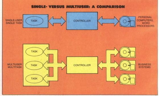
A main feature of Adaptec's SCSI is its ability to support multiple hosts and devices and thus multiple tasks. In a typical single-user environment, the relationship is one-to-one; as tasks are added, so are the number of disk accesses threatening a major I/O bottleneck. SCSI allows multiple tasks to address any of several storage devices. I/O channel bottlenecks are avoided by arbitrating bus data transfers with disconnect/reconnect capability within the SCSI bus controller.
