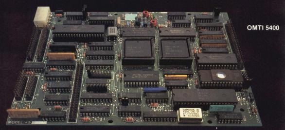
Our OMTI 5400 SCSI (SASI) controller offers Winchester, floppy and tape support all on a single 5¼" footprint PC board. By using our proprietary VLSI chip technology, we were able to squeeze all these functions onto a board size that most controller companies are still using for single function controllers. This means increased capability and improved cost-effectiveness in your application.
