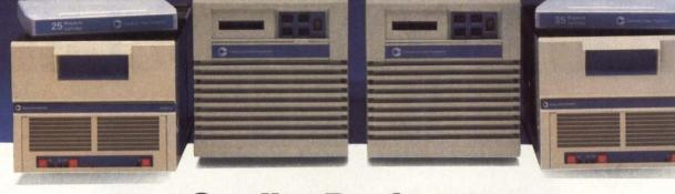
This new family of high performance, 8-inch disk memories uses advanced technology and provides compact, reliable mass storage. For example, our new 8-inch Winchester, the C2476, is the ideal choice for computer systems utilizing disk memories in multiuser and multi-task environments which require fast access to large files of data. The C2476 stores 476 megabytes in significantly less cabinet space than previously available models and has an average positioning time of 15 milliseconds.
