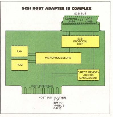
**An SMS/OMTI implementation of SCSI** combines microprocessor, cache memory, ROM firmware and a host adapter, that matches the controller to virtually any system bus configuration.
