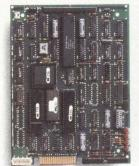
With Champion, you can interface two serial-mode ESDI 5¼" Winchester drives to the SCSI bus. These large capacity drives support up to 10 MBits-persecond disk transfer rates, higher bit densities per track and range from 110 to 380 megabytes. The Champion also features hard and soft sectoring capability. **CIRCLE NO. 22 ON INQUIRY CARD**
