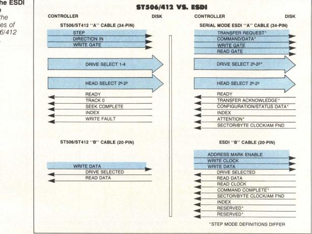
Fig. 1. The ESDI interface extends the capabilities of the ST506/412 interface.
