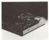
YD-380-1714 51/4-inch disk drive's dual-speed feature allows operation with either the current standard format for 51/4-inch media or the new high-capacity 51/4-inch media. The drive reads and writes on either the standard 1M-byte, double-density, double-track format or the new high-capacity 1.6M-byte unformatted/ 1.2M-byte formatted disk. Data transfer rates are 500K and 250K bps; track density is 96 tpi. As many as four drives can be daisy chained. A read and write head design, steel
