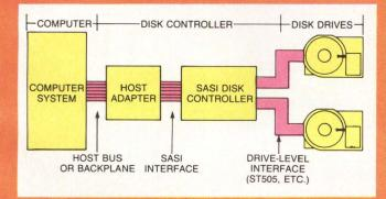
A typical SASI interface configuration consists of a host system with adapter, controller and devices. This is still the most common SASI implementation and established the methodology for interfacing devices with differing host systems
