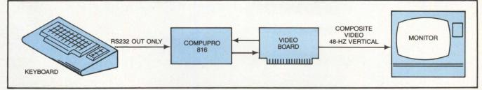
Echo-replacement software automatically displayed a predetermined message on the monitor, one character at a time, no matter what key the actor hit. Software also replaced the input signal with a predetermined output signal and sent it to the monitor through the video board.
