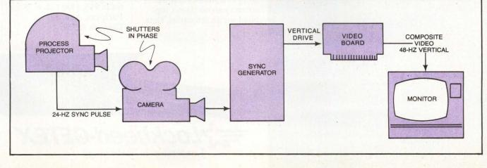
Modified video boards scanned CRTs at the same 24-frame-persecond rate the movie cameras used to shoot. This method solved the synchronization problem that results in flickering horizontal bars that continually roll up the screens of monitors in low-budget films.
