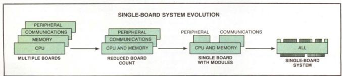
Fig. 1. Thanks to LSI and VLSI circuitry, the number of computer system functions that can be placed on a single board has been growing. Single-board computer manufacturers will soon be offering
