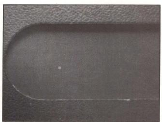
A barely visible fingerprint, seen here as a dot on a diskette's surface, contains information that allows encrypting and decrypting of programs stored on the diskette. Vault Corp. has applied for a patent on the process that creates the fingerprint.
