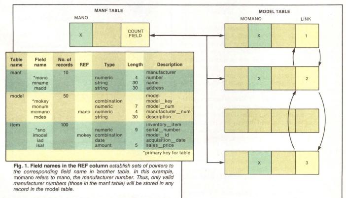
Fig. 2. Doubly-linked lists of records speed data-access searches. Pointers connect each record in the model table with manufacturer number "X" to the record in the manf table with that manufacturer number and vice-versa. In addition, each manf record stores a count of the records in model to which it is linked, and each associated
