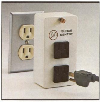
The "SurgeSentry" three-stage surge suppressor uses a gastube, silicon avalanche suppressor and metal-oxide variator to detect a spike in less than 5 psec. The device is tested to the IEEE 587 and UL 1449 standards.
