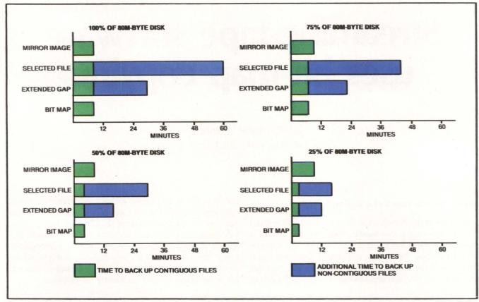
Fig. 2. The backup time for the four approaches to streaming tape is approximately equal, as long as the disk is full and files are contiguous. The time needed by the selected-file and extended-tapegap methods for non-contiguous files is much greater than the
