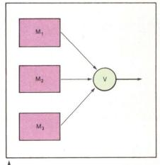
Fig. 2. Triple-modular redundancy (TMR) provides three identical modules and a "voting" circuit. The voting circuit (V), presents a majority vote of the three modules' outputs, thus masking a faulty module.
