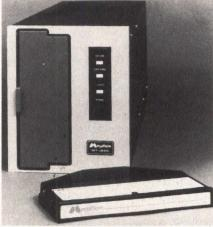
back up a 300M-byte disk in 24 minutes. Information is stored using a 24-track serpentine format with a 9,600-bpi density. An integral formatter that is transparent to the controller encodes data in a 4/5 GCR bit-serial format. A two-track read/write head assembly steps 12 times to create the 24 tracks. This arrangement permits recovery of stored files within an average of 30 seconds. \$4,950. MegaTape Corp., 1041 Hamilton Rd., P.O. Box 317, Duarte, Calif. 91010, (213) 357-9921.
