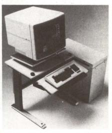
virtual-address system affords pixel-bypixel access to the memory-mapped display, and the system can simultaneously display as many as 16 softwareselectable colors from a palette of 4,096. The electronics are contained in a 25-by-12-by-36-inch tower unit that includes an ANSI-compatible, lockable, ergonomic keyboard with 16 program-
