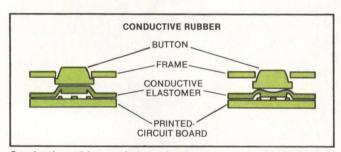
Conductive-rubber switch technolgy uses a molded sheet of rubber that forms a dome beneath each key. When a key is depressed, the dome collapses and makes contact with the circuit below it. The dome then pops up again.
