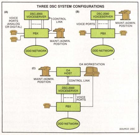
Compatibility with these peripherals puts the DSC-2000 to work in office-automation environments. Subscribers can access the Voice-Server from workstations and terminals as well as from telephones. The terminal display and keyboard can be used to control mailboxes, message attributes and messaging functions.
