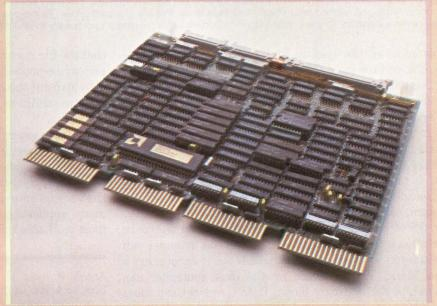
Two controllers in one. Spectra Logic Corp.'s Spectra 25 is a single-board disk/tape controller for Digital Equipment Corp.'s LSI-11 and PDP-11/23 computers.
