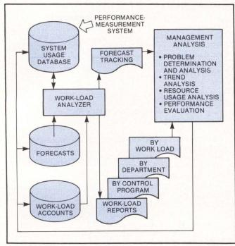
Fig. 2. A work-load analyzer provides plots of work-load patterns over time, reporting the capacity usage by equipment class, and enhances trend and forecasting capabilities. Reports are produced daily, weekly or monthly and indicate work-load activity levels. Report analysis helps modify system usage and forecasts.
