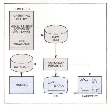
software should impose little burden on a system for economic reasons and should avoid disturbing the observed system. To avoid burdening the system, the collector stores raw data on disk or tape for later reduction, analysis and reporting (Fig. 1).
