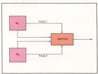
Fig. 4. An alternate fault-tolerant approach features module self-checking. Surrounding modules can query to determine when a module has failed and then can disconnect the faulty module from the system and use a spare module. Alternatively, the remaining modules can assume the processing tasks of the failed module.
