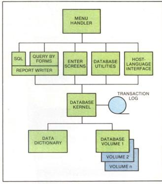
Fig. 5. User interaction with Unify takes place via the menu handler. The database kernel manages data access for the non-procedural and host-program interfaces. The data dictionary maintains menu hierarchies and user passwords.
