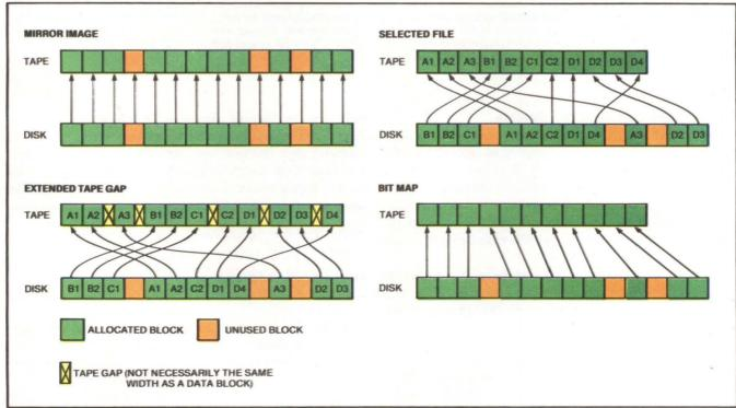
Fig. 1. There are four techniques for disk-to-tape copying. The mirror-image approach copies disk to tape sequentially, transferring both allocated and unused disk blocks. In the selected-file approach, sequential blocks of tape represent sequential logical file blocks rather than sequential physical blocks. Therefore, unused blocks need not be transferred. The tape drive stops and starts while waiting
