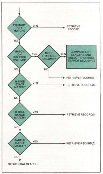
Fig. 3. Selecting an access method involves a hierarchy of options from a primary-key match to a sequential search. In general, Unify chooses the access method on its own according to the algorithm shown. However, application developers can bypass the usual procedure by specifying any of the access methods shown in the figure.
