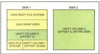
Fig. 4. Unify's disk space can be organized as a file managed by UNIX (yellow) or as a logical or physical disk that is separate from UNIX (green).
