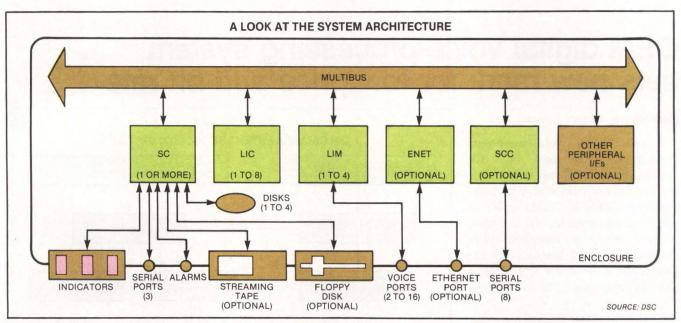
The system architecture is open-ended on the Multibus and contains system controller (SC) cards, a line interface controller (LIC), a line interface module (LIM) and optional off-the-shelf boards such as Ethernet (ENET) and serial communication cards (SCC).
