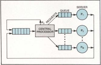
Fig. 3. Central server models portray tasks in queues awaiting servers. Such analytical queuing models aid in performance measurement of a system that cannot be evaluated directly.
