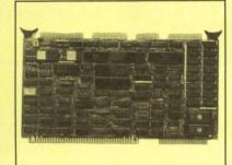
THE SBC90A designed for multiprocessor/ slave or I/O processor, has on card Z80A (4MHZ); DMA; 128K dual ported RAM, no wait state, byte/word accessible; MEMORY MAP RAM; EPROM sockets up to 32K; 2 RS232; 2 parallel ports; 3 counter/timers; floppy disk controller; hard disk interface; math chip AM9511; 20-bit address; 21 vectored interrupts. Multibus compatible.
