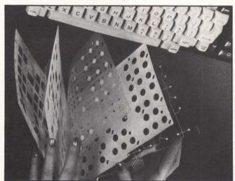
Membrane-switch technology uses a plastic sandwich that contains a spacer sheet with holes for the contact areas. Although many membrane keyboards are flat panels, they can also be actuated by full-travel keys. (Courtesy of Micro Switch)
