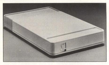
modes for initiating and receiving telephone calls and a diagnostics program that displays modem status characteristics on-screen. The units also incorporate tone- and pulse-dialing options and an internal speaker to monitor data transfer.
