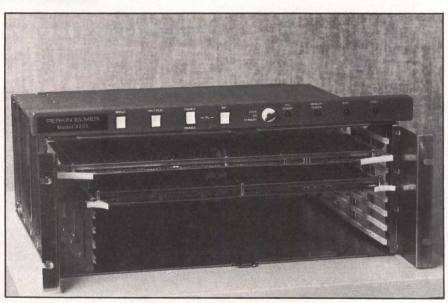
P-E's 3205, an OEM version of the company's 32-bit superminis, includes the CPU, 1M byte of RAM and a peripheral controller for less than \$10,000 and runs UNIX or P-E's real-time OS/32.
