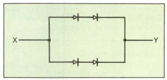
Fig. 1. Diode masking prevents either an open or a short between nodes X and Y as a result of any diode's failure. The implementation uses four diodes instead of the usual one.
