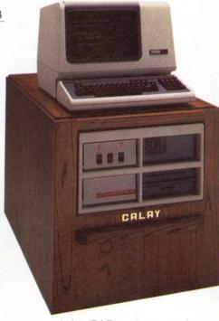
your existing CAD environment the Calay RPR-300 Router and feed it the data from your REDAC or APPLICON. After a short time of the fully automatic routing process, you get the complete data of a routed PC board, which is fed back to your original CAD system for output documentation purposes.
