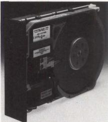
shock. It is configured with an oxide-coated disk and four read/write heads-two per surface-each of which addresses 306 cylinders. The drive operates at an average access time of 65 msec. using a stepper-motor-driven actuator. A proprietary off-track compensation system permits operation at track densities of 550 tpi. The drive has 612 tracks per surface, divided into two 306-cylinder bands. \$690 (1,000 units). Seagate Technology, 920 Disc Dr., Scotts Valley, Calif. 95066, (408) 438-6550.
