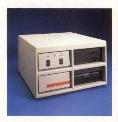
For large configurations, choose the DSX80000 foundation system with eight Multibus slots, 10, 20, 40 or 80Mb of Winchester storage plus an 8" IBM compatible floppy.
