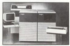
The Auragen System 4000 32-bit superminicomputer has UNIX, programmerinvisible fault tolerance and an easy-to-use collection of software-development tools.
