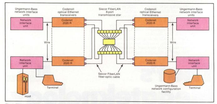
Fig. 2. Fiber-optic-based network from Codenoll Technology, Ungermann-Bass and Siecor FiberLAN connects nodes via Ethernet plugs to optical transceivers. The node hardware and software regard the network as standard Ethernet equipment, requiring no modification.
