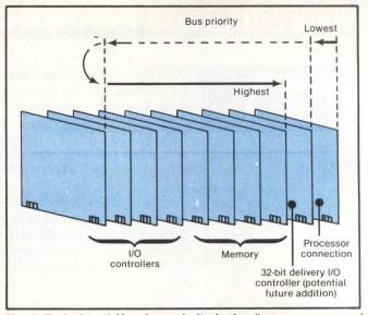
Fig. 7. Redesigned Megabus priority logic allows processor and 32-bit I/O to be closer to memory without changing priority. Priority signals are driven "backward" across processor and 32-bit I/O.
