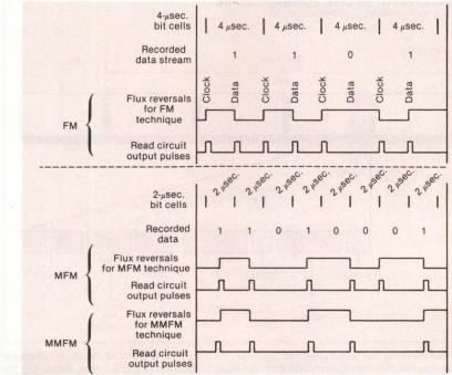
The intent of MMFM was to improve the read margins for still more density, but the use of MMFM became a moot point when IBM Corp. adopted MFM and established it as a de facto standard. MMFM's additional data capacity and lower error rate were not cost-justified.
