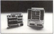
The SBX-FDIO can control up to four single or double sided, single or double density 5¼ inch or 8 inch floppy disk drives. A software toggle allows both 5¼ inch and 8 inch drives to be intermixed on the same cable!
