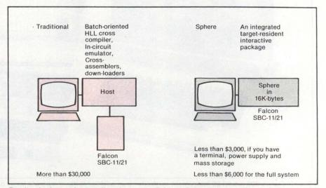
By developing software directly on the Falcon, Sphere users can save both time and money compared to developing programs first in a host.
