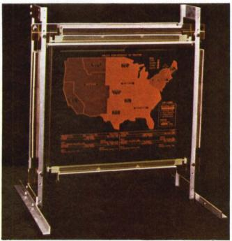
**The OEM version of IBM's plasma display** measures  $17\frac{1}{4} \times 10 \times 3$  inches and weighs 27 lbs. While IBM is targeting its end-user system for desk-top applications in the company's 3270 terminal series environment, the 581 can be integrated into systems operating in any environment. Prices start at \$3400.
