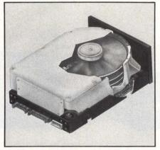
Applied Information Memories' fourplatter "Dart" drive has 1,000-tpi track density and 19,220-bpi bit density and uses standard MFM recording code. Capacity is 140M bytes.
