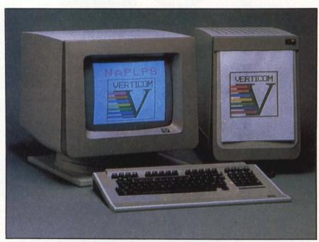
Verticom Inc.'s terminals are both ASCII and NAPLPS compatible and emulate the DEC VT100 and Tektronix 4010. Resolution is 640-by-480 at 30 Hz interlaced. The low-profile keyboard has 105 keys and a palm rest.
