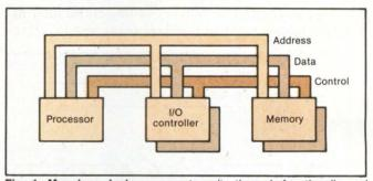
Fig. 1. Megabus design connects units through functionally and electrically identical contacts. Address, data and control signals are accessed in the same way by all units.
