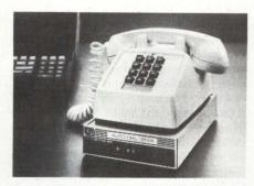
The modem's self-test system and multiple DIP switches permit any user to install and adapt the Auto Dial 212A to virtually any computer or terminal. The Auto Dial 212A also features a low parts count for low cost and high reliability. Three vendor-developed microprocessors compress the entire range of modem functions within 12 ICs, all contained on one PC board. Price is less than \$600 in single-unit quantities. U.S. **Robotics Inc.**, 1123 W. Washington Blvd., Chicago, Ill. 60607.
