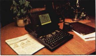
**Grid Systems' portable microcomputer** incorporates a Sharp electroluminescent display. Emulating DEC VT100 or IBM 3270 systems, the Compass can be used as an intelligent terminal in the office or as a portable computer on the road. The Sharp display provides users with graphics and alphanumerics capability and enables the Compass to fold into a 2- $\times$  11<sup>1</sup>/<sub>2</sub>- $\times$  15-inch package.
