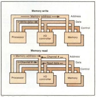
Fig. 2. Megabus memory transfers occur over address and data leads. During a memory read, the address and data leads carry different information on the request and response cycles. The processor identifies itself by channel number on the data leads during the request, and recognizes its channel number on the address leads during the response. During a memory write, the address and data leads are used to specify an address and carry data.
