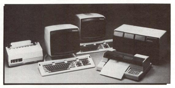
**DG's microEclipse-based Desktop Generation** is available in a variety of configurations ranging from a \$3,165 single-user system that includes an Intel 8086 co-processor for running MS-DOS and CP/M-86 packages. Multiuser configurations supporting as many as 12 terminals are possible. With the system, DG is introducing a new Mannesmann Tally printer (left) and a Hewlett-Packard plotter.
