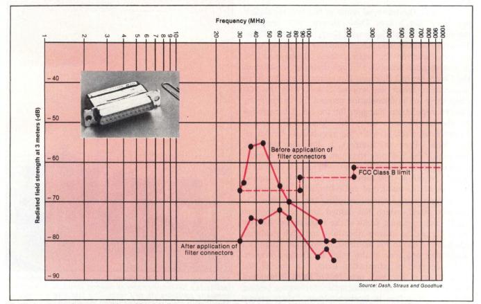
Emitted radiation from a graphics tablet, initially more than 10 decibels above the FCC's limits for Class B mass-market devices, complies with the regulation after the addition of three ITT Cannon filter connectors (inset). The filter connectors are placed on the tablet's two I/O ports and on its power-supply connection.
