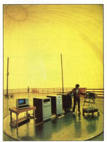
"The Bubble," Digital Equipment Corp.'s corporate verification facility, is a 100-foot-diameter air-support structure, in which the company performs its RFI tests. The test site includes an 18-inch-diameter turntable, on which the equipment under test can be rotated to determine the worst-case RFI configuration, and a large ground plane, on which the entire test station rests.
