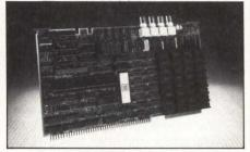
**MLZ-VDC** intelligent 640 x 480 x 4 color graphic controller based on the NEC 7220 controller chip with on-board Z-80 CPU, DMA controller, and user definable FIFO interface to Multibus<sup>TM</sup> Users may display up to 16 colors from a 4K palette. Up to 1024 x 1024 x 3 interlaced also available.
