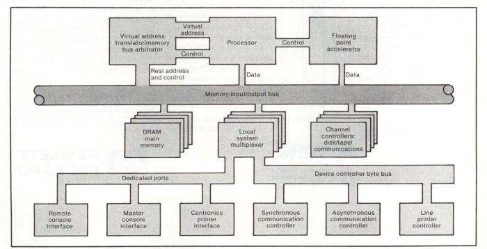
A 27M-byte-per-second bus links the A.B. Dick MC-30 CPU, memory and I/O processors. The company claims that its first minicomputer product offers twice the performance of a DEC VAX-11/780 and is positioned for UNIX OEM suppliers.
