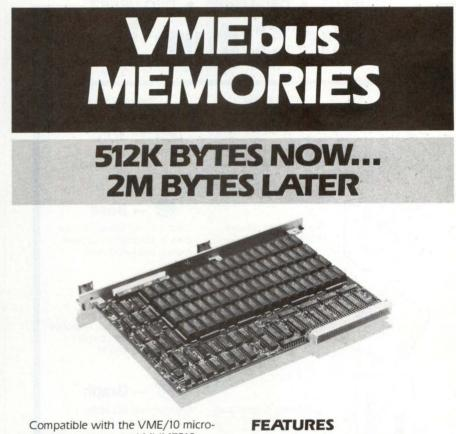
Compatible with the VME/10 microcomputer system and MVME210 memory board, the MM-6000D is a high density memory that can employ either 64K or 256K DRAMs. A jumper option selects either 64K or 256K DRAM operation.
