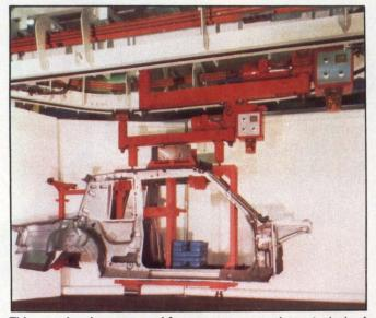
This overhead, power-and-free conveyor system, typical of material-handling systems installed in factories, could be used with manual or automated assembly lines. Most assembly includes some manual work, says George Ramsden, of Jervis B. Webb Co. "Although the assembling of some rather sophisticated office equipment is now being done without any human hands, it requires a lot of robots—and a lot of volume to justify a lot of robots," he adds.
