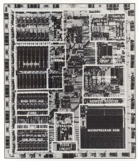
Harris Corp.'s version of the 80C86 CMOS replacement for the Intel 8086 uses 2.5-micrometer geometries to pack 38,000 transistors onto a ¼-square-inch die. A 5-MHz part will initially be offered, but it will be followed by an 8-MHz version and a family of peripherals as well as a CMOS version of the 8088.
