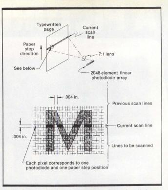
Fig. 3. Optical scanning. A 2048-element linear photodiode array detects light from a line one pixel high, with each pixel representing an area on the page of 0.000016 sq. in. Each text character occupies a 24  $\times$  32 pixel frame.
