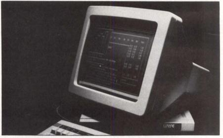
The WY-50 from Wyse Technology is the company's lowest priced offering featuring a 14-inch diagonal screen and 80 or 132 columns.
