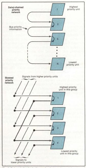
Fig. 5. Daisy-chained priority mechanism produces delays as each unit receives and passes on the priority information. Skewed priority network resolves priority in groups of 10 (four units are depicted here for simplicity). Unit 1's "service not requested" signal (boldface line) is passed directly to unit 4 without passing through units 2 and 3.
