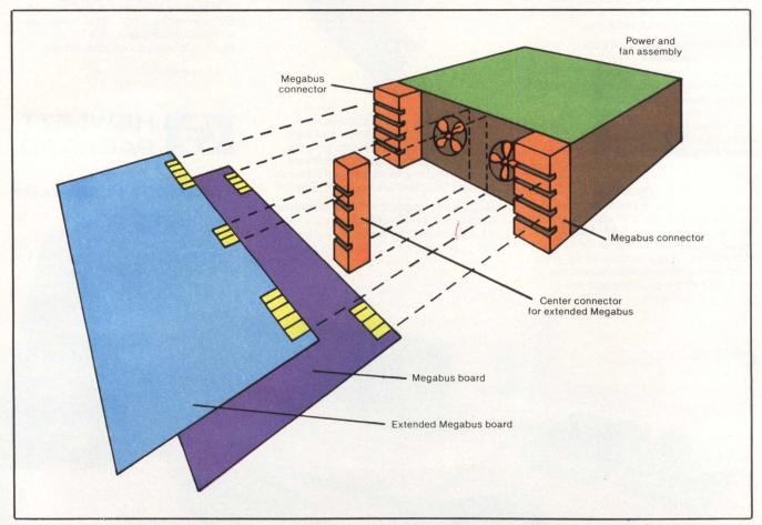
Fig. 6. Extended Megabus connections are implemented through an added center connector carrying additional data and control leads. The center connector is configurable on a single-bus-slot basis.
