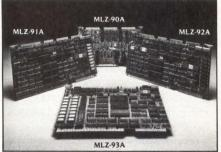
**MLZ-90A** single board microcomputer with nine byte-wide memory sockets for use with RAM or ROM (AM9511 and floppy disk drive controller optional).
