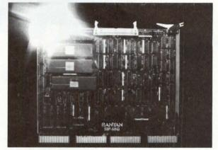
Q-Bus. And Quest memory is available in static RAM (90 nsec cycle—no need for cache) or dynamic RAM; both on quad boards for up to a maximum of 16 MB.
