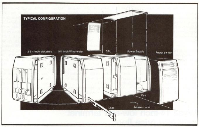
DG has adopted a modular packaging system for the Desktop Generation microcomputer series. It uses 4½-inch-wide components that snap together to form a rigid unit. As many as six modules can be linked and installed horizontally on or near a desk. A floor mount-option is available.
