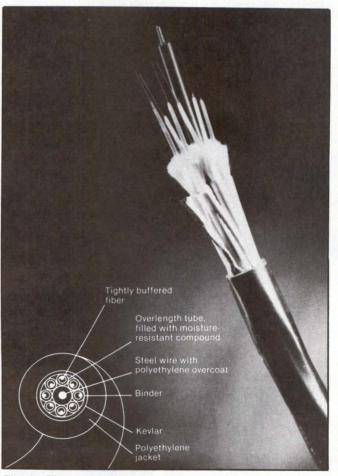
Fig. 1. Fiber-optic cable from Siecor Corp. consists of fused bundles of glass rods that transmit light from end to end. The cable pictured comprises eight fiber bundles with a central steel wire for stiffness.
