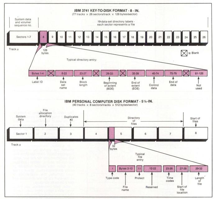
Formats vary widely, even within IBM. The above figures illustrate the disk formats of the IBM 3741 (8 in.) and the IBM Personal Computer (5¼ in.). The TM-500 resolves the different formats by reading file-directory information from the source, locating occupied files, formatting the destination disk and transferring the source records to the destination disk.
