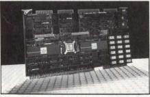
**HK68**<sup>™</sup> powerful and versatile single board UNIX<sup>™</sup> or CP/M-68K<sup>™</sup> system with MC68000 CPU, MMU, quad channel DMA, four serial ports, 128K or 256K bytes of onboard RAM with parity (expandable to 1M byte on-board!), and two iSBX<sup>™</sup> connectors for I/O expansion.
