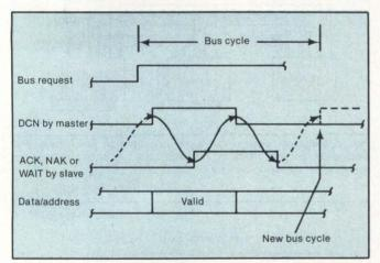
Fig. 3. Bus-cycle timing is performed by the master and slave involved, without a central bus controller. Priority resolution to select the next master is accomplished during the current bus cycle if another unit wants the bus.
