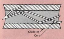
**Optical fiber** consists of a core surrounded by a cladding of lower optical density. Light entering the core at a sufficiently shallow angle with respect to the core axis will be reflected back into the core, traveling through the core until it emerges at the other end. If the light enters at too sharp an angle, it will escape the core into the cladding.
