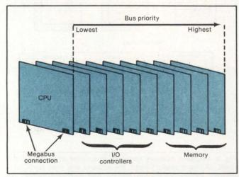
Fig. 4. Bus service priority is linear from processor to farthest memory controller. Memories are assigned high priority to allow completion of memory read responses as quickly as possible, freeing the memory for further requests.
