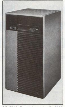
A.B. Dick's first minicomputer, the 32-bit MC-30, comes in a 23.8-inch-by-44.75-inch cabinet that houses a two-board CPU and 25-slot card cage. A matching peripheral cabinet accommodates SMD interface disks and start/stop tape drives.
