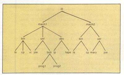
Fig. 1. The @ directory is ALTOS-NET II's extension to XENIX's hierarchical file system. Traditionally, XENIX files on separate machines are linked by utilities that confine network functions to file transfer and remote log-on. But the @ directory establishes a new root on the tree, enabling all utilities and applications to function throughout the network.
