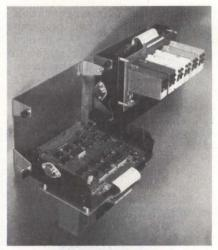
each for address, data and control. The SRP24's communications port is compatible with the 24-line PIO ports of most common microcomputers including Multibus, Microbus, STD bus, DEC and others. Price is \$350 in single-unit quantities. Adatek, P.O. Box 1339, Sandpoint, Idaho 83864.
