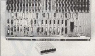
Wang's 64K-byte dynamic RAM module, shown in the foreground against a VS computer system board, houses 1M byte, as does the board, but would take up 3 square inches (shown). The VS board includes error checking, while the SIMM would require four extra modules to perform error checking, adding 1 inch to the module's size.
