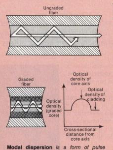
spreading caused by the different path lengths of light rays entering a core of uniform optical density at different angles. A ray traveling straight through such an ungraded core will arrive before a ray that reflects off the sides. A graded core fiber has a varying optical density, so rays travel faster as they approach the cladding, reducing the difference in arrival times. Rays entering graded cores at an angle follow a curved path resulting from the continuously varying refraction.
