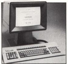
A dark-on-light display, such as the one (shown) on TEC's ET80, is favored by Deutsche Institut für Normung standards. A 70-Hz refresh rate is employed to reduce flicker on the ET80.
