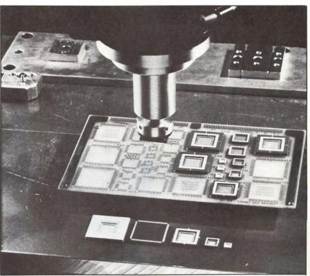
Control Automation's Mini-Sembler robot can be controlled by any computer and programmed in any language. It is targeted to precision-assembly applications.
