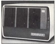
Computer Automation's Naked Mini division is addressing the shifting computational performance range with a 186-based system multi-user system called OMNIX 186. The basic configuration includes 384K bytes of RAM, four serial ports, a 5M-byte, 51/4-in. Winchester disk drive and a 1M-byte floppy drive for a single-unit list price of \$8990.
