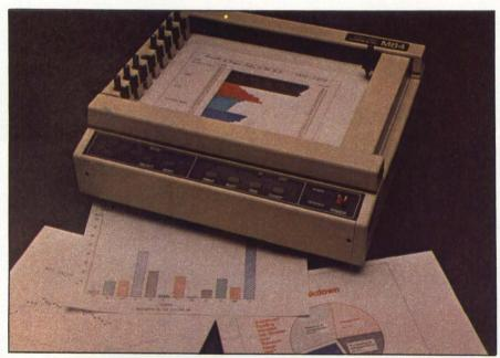
CalComp is entering the low-end pen-plotter market with the Model-84, an eight-pen unit with an end-user price of less than \$2000.
