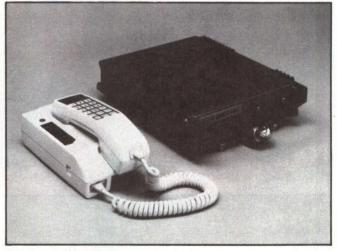
Mobile phone unit from Oki includes a handset, usually mounted within reach of a driver, and a box mounted in the trunk handling transceive and control functions. Most mobile units are used with two antennas for optimum reception.
