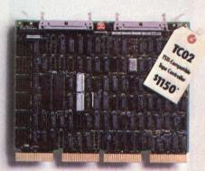
Coupler works with all NRZI, PE, GCR formatters at speeds from 12.5 to 125 ips.
