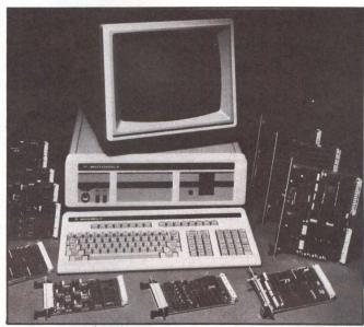
VME/10 expansion modules available from Motorola and other suppliers provide flexibility for many OEM industrial and scientific applications. The basic system includes an MC68010 microprocessor, 384K bytes of RAM, a 15-in. display and 20M bytes of unformatted mass storage.
