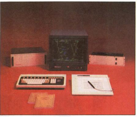
**Genisco's new 6210 high-end graphics terminal** features  $1392 \times 1024$  interlaced resolution and can display as many as 4096 colors out of a possible 16 million on a 19-in. monitor. Maximum display list memory is 1M byte.
