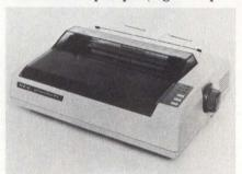
NEC Information Systems Inc.'s Pinwriter series of low-cost, dot-matrix printers features 18 printing pins to form high-density characters.
