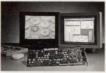
Better effective resolution can be applied to signal data that's taken in under low light or low contrast conditions with the DT2867-LC precision frame grabber. These conditions are more prevalent in microscopy and astronomy work. The device contains a continuously adjustable analog-to-digital offset and reference, and a separate programmable gain amplifier. These functions fine-tune the board's input range to allow over 16,000 selectable ranges. Consequently, the board makes it possible
