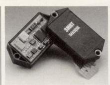
ment format. Operating from a 5-V power supply, the sensors are packaged in a thermoplastic housing with with a standard single in-line package connector and barbed ports for plastic hose hook-up. SMRT sensors are available now at prices starting from \$115 each in 100-piece quantities.
