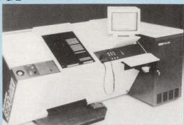
1792 universal pins at data rates to 40 MHz. S790VXI prices start at \$275,000, and delivery is within 120 days.
