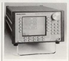
analog output stages. This technique yields nearly ideal sine, haversine, square, triangle, ramp, and pulse waveforms. Linear and log sweeps are phase continuous. White noise can be added to any waveform. Because the chosen modulation signals are merely a part of the waveshape calculation, they have virtually no distortion or frequency limits.
