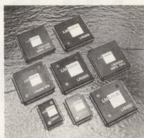
LR3208 video-frame controller drives a 1024 by 768 by 8 terminal consistent with the ARC specification
