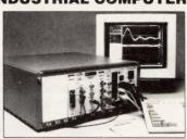
EISA and AT bus, rackmount industrial computers. Modular, interchangeable, multi-vendor industrial PCs. Noise, emissions, power, ground, airflow & cooling are specified & verifiable. All PC functions, from CPU (286/386/486) to power supplies, are enclosed & protected in metal-shielded modules, with front panel
