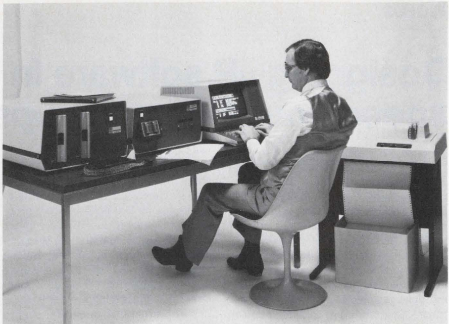
Write, edit, and debug a microprocessor program, then transfer it to PROM, with a development system like this one, from Tektronix.
