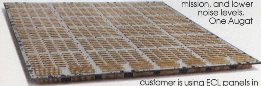
Large scale ECL wire-wrap panel with 660 SIP/DIP patterns.
