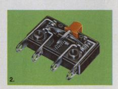
2. Coil spring snap-action mechanism extends life of switch. (Outlasts stressed blades in terms of metal fatigue.) Overcenter and compression springs are not stressed to their limits even under full overtravel as are stressed blades. Coil springs retain characteristics longer under usage than stressed blades.
