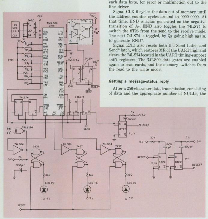
6. Data parity is tested again as information leaves the memory and enters the UART. The CPU acknowledges or
