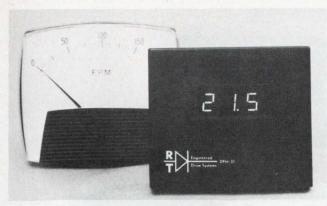
Replacing analog meters is another long-sought goal of DPM makers. This unit, from R.T. Engineering Service Inc. (Mansfield, MA) incorporates an Analog Devices DPM in a package designed to fit analog-meter slots.
