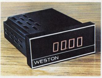
**Zero means zero** on Weston's 4 1/2-digit Model 2470. The unit has  $\pm 1$ -count stability at zero over a 0 to 50 C operating range, and no dead band at zero.
