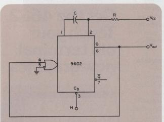
1. This retriggerable multivibrator generates a single pulse whenever  $\rm V_{cc}$  comes on. The pulse can be made long enough to reset storage elements in digital circuits.
