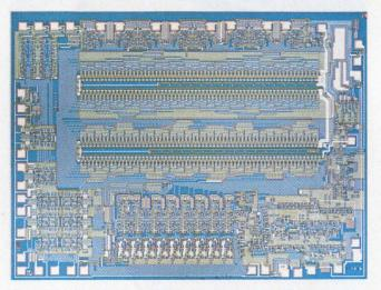
The first single-chip monolithic data-acquisition system, the ADC0816 by National Semiconductor, has an 8-bit a/d, a 16-channel multiplexer and microprocessor-interface logic. It performs a conversion in 50  $\mu$ s.
