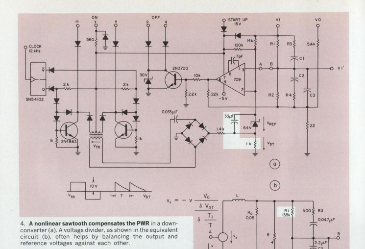
The equivalent circuit for the down-converter is shown in Fig. 1b, for the up-converter, in Fig. 2b. Both these equivalent circuits assume that the components are ideal: lossless transformers with no leakage inductance, plus transistors and diodes with no voltage
