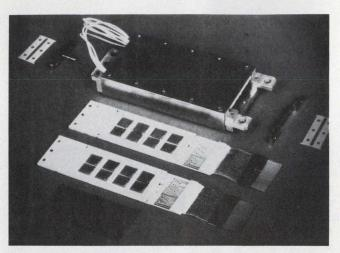
Four PPS-8  $\mu$ Ps control four independent bubble-memory channels in this NASA 102.4-Mbit solid-state recorder, which replaces tape machines. One of the channels is shown here. Total rate for all channels is 2.4 MHz.
