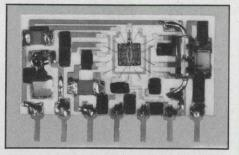
ULTRA SMALL ACTIVE BAND PASS FILTER fabricated using OP Amp incorporated Hybrids Circuit. Operating Voltage 1-2.5V/4-15V, Frequency Range 288.5-2800Hz, Q 180+20, 35+5 and etc. .788" × .138" × .433". By adding Feed Back Circuit of extra Diode and Capacitor, it does the job of small but reliable Oscillator. Active Filters can be tailor-made to customer's specifications. IWATA ELECTRIC CO., LTD. Mansei Bldg., 1-1-16 Sotokanda, Chiyodaku, Tokyo, Japan.
