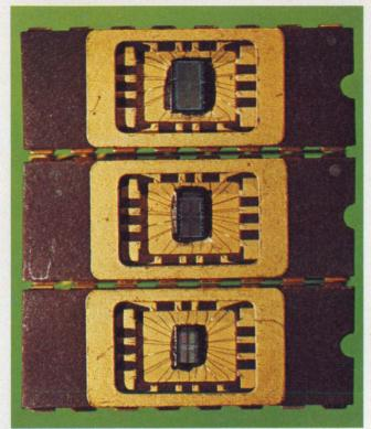
VMOS shrinks static RAMs. These three AMI 1-k static devices went from 100 to 83 to 66 mils on a side, while access times dropped from 45 ns to 35 to 25.
