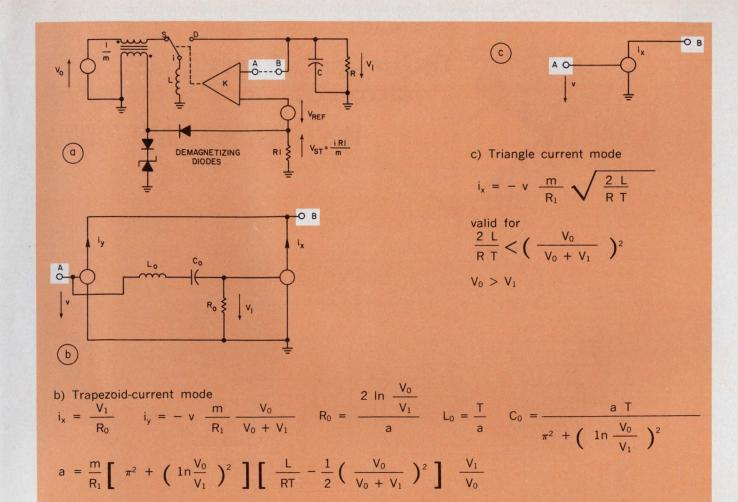
9. An up-converter with current-proportional-sawtooth (a) works in the trapezoidal-current mode (b), so the
