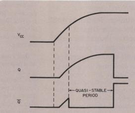
2. A single pulse from the multi's Q output rises with the applied supply voltage. The  $\overline{\mathbb{Q}}$  output also begins to rise, but reaches only 2.3 V before going low.
