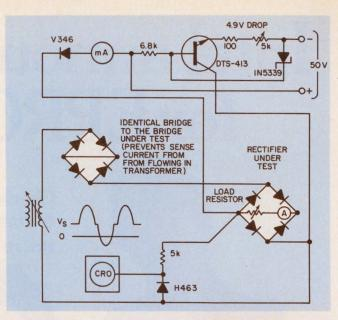
Acting like a full-wave bridge rectifier, this test circuit treats the diode as if it were in actual use in its intended circuit and applies sensing current as well.
