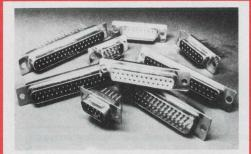
SOURIAU Sub "D" Series 8634 NORMAN-D connectors are low cost, crimp type, w/ stamped & reeled contacts for lower install. costs; intermateable w/ all "D" connectors. SOURIAU has "D" connectors in 1-piece thermoset, 2-piece thermoplastic insulator, non-removable solder contacts, rigid & float mount shells, crimp, rear release contacts, operating temp of -55°C to +125°C qualified to MIL-C-24308. SOURIAU, INC., 7740 Lemona Ave., Van Nuys, CA 91405 (213) 787-5341.
