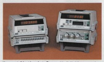
You can tell just how hot  $\mu$ Ps are with digital thermometers like Fluke's processor-controlled units. Microprocessors here control, and are part of, the a/d converter. They also handle I/O and massage data.
