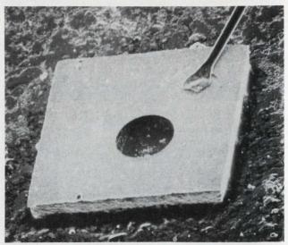
The best emitters for optical communication systems up to 50-Mbits/s are Burrus-type diodes, like this General Telephone and Electronics diode chip.
