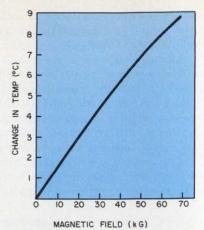
1. Applying a strong magnetic field changes the temperature of gadolinium. The variation of temperature with field shown above was obtained in NASA experiments.
