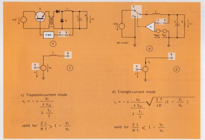
1. A down-converter switching supply (a) relies on constant-frequency switching. Varying the switching-pulse width regulates the output. The equivalent circuit for the entire supply (b) shows that the PWR responds
