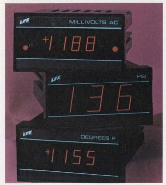
For process-control applications, DPMs like these LFE units include signal-conditioning and direct readout in engineering units. Meter relay-like setpoints are available.
