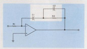
3. An integrator/filter circuit can be built with a wideband op amp and RC feedback network.
