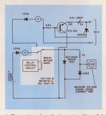
4. When sensing and operational currents can't be applied together, a relay arrangement switches to a sensing mode for 1% of the operating period.
