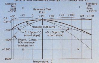
Designed to meet or exceed Mil-R-39035 Char. H requirements. Settability of 0.01% typical, 0.05% max.
