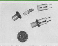
New subminiature replaceable-lamp incandescent lights. 50% cheaper than conventional submini flange-base or bi-pan because lamp base formed for bulb's glass and lead wires permits high-speed production. Socket-and-assembly design for one-hole mounting. Flat, dome, seven colors, 2 to 28 V. Samples and specs: Industrial Devices, Inc., Edgewater, N.J. 07020.
