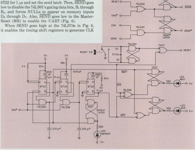
5. After all cards have been read, the send pushbutton shuts down the feed motor and read lamp, and sets up
