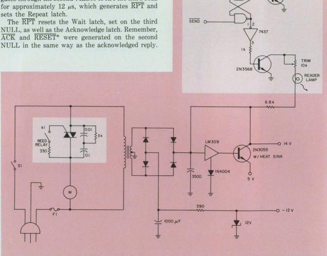
7. Power-supply and motor-control circuits are straightforward. The R-C across the triac suppresses noise.
