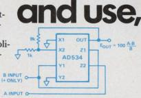
computes the percentage deviation between its two inputs. The scale factor in this arrangement is 1% per volt although other scale factors are obtainable by altering the resistor ratios.
