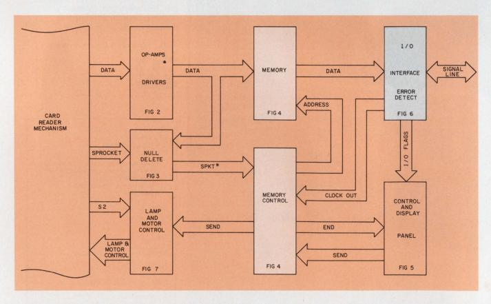
1. Internal memory in a card reader accepts parallel input data, delivers serial data, and simplifies the I/O design.
