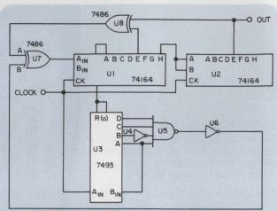
**Stop pseudorandom generator interruptions** with a binary counter that feeds a logic ONE into the shift register when too many zeros occur.
