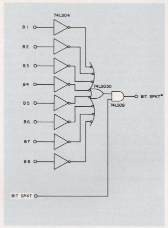
3. A simple "delete" circuit keeps the NULL signal from reaching the memory.
