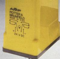
CMOS controlled CG time delay. Standard delays range from 0.1-1 sec. to 10-100 min. Delays to one year or more available. Repeatability is typically .05% for DC units, 0.1% for AC, including the first cycle! DPDT contacts rated 10 amps at 120V AC. Delay on operate, interval on or delay on release models.
