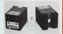
RUBIDIUM OSCILLATORS Series FRK are ultra stable, reliable, light (2.9 lb) small (4x4x4.5") and ideal for navigation/posi-(4x4x4.5") and ideal for lavigation/position location and communication systems. The unit provides 10 MHz; 5 and 1 MHz optional. Long-term stability 1x10<sup>-11</sup>/month, short term 1x10<sup>-12</sup>/100 sec. avg times and extremely low noise. Available commercial and MIL (radiation hardened) EFRATOM CALIFORNIA, INC., 18851 Bardeen Ave., Irvine, CA 92715 - (714) 752-2891
