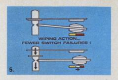
5. Wiping action helps clean away surface contamination in low level circuits, where contact resistance must be kept low. Breaks through minor contact welds that cause switch failure under high current conditions.
