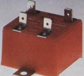
New low-cost ECT hybrid AC relay. Reed-triggered triac switches 2 to 32 amps. Now with AC or DC input. Life to 10 million operations. Has built-in snubber for loads of .40 P.F. or greater. UL-CSA rated.
