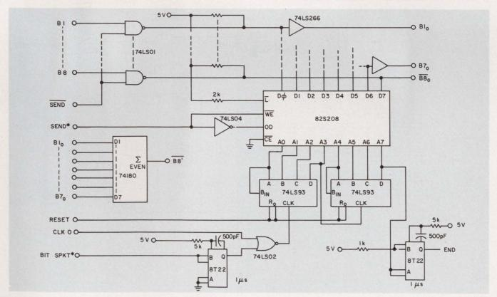
4. Data are checked for parity errors by an exclusive-NOR gate during memory loading. If the parity bit, as read in
