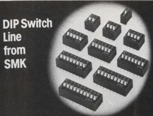
The JS-8722 Series is a complete line of DIP Switches, from 1 to 10 positions, featuring sealed construction to prevent flux contamination during wave soldering. A clip-type wiper design assures positive 2-sided contact to provide excellent shock and vibration characteristics.
