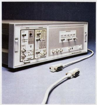
It takes more than one  $\mu P$  to digitize a transient. In Tektronix' 7912, there's a processor in each plug-in and two more in the mainframe.
