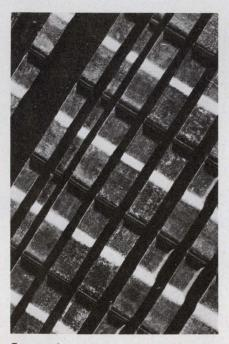
Formed strips of aluminummagnesium foil, bonded to the platelets and activated after assembly by oxidation, form a layer of magnesium oxide, which is a good secondary emitter.
