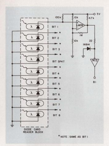
Cards are read by a standard diode-block assembly.IC comparators form the necessary TTL-level signals.
