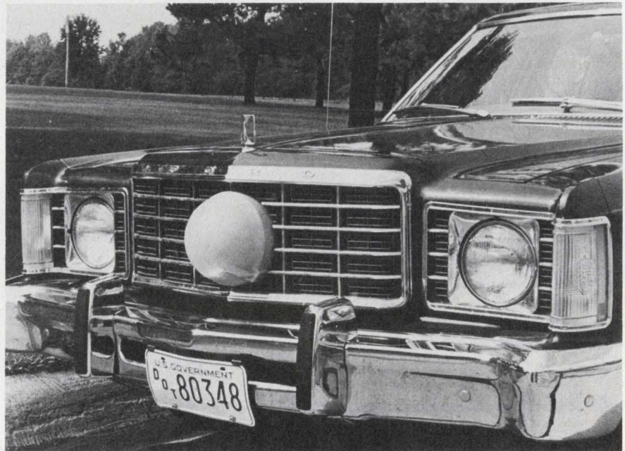
This radome for an experimental radar braking system protects radar elements from the weather. Small antenna beam width and range gating minimize false alarms that have plagued similar systems.
