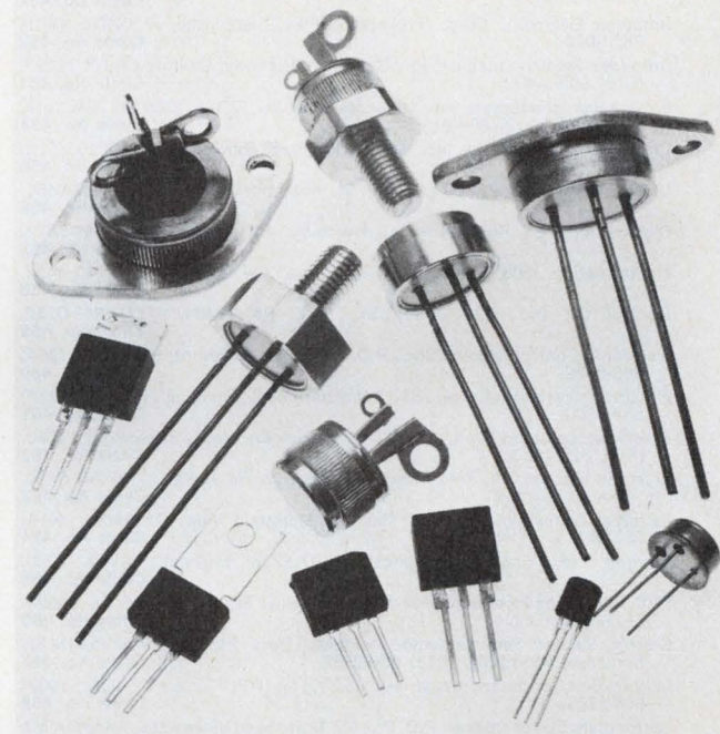
Thyristors and SCRs from Teccor are in the low and medium-power range. They are appliance-grade units, some with lugs, others with push-on terminals and ruggedly packaged in TO-3 cases.
