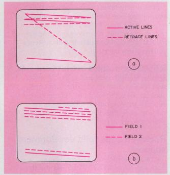
1. Both a non-interlaced video display (a) and an interlaced display (b) generate images on a CRT screen. But, the interlaced display effectively provides double the resolution of the non-interlaced version.
