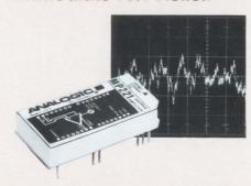
Check that scope photo. It's the output of our MP221 ultra-low-noise, ultra-low-drift chopper amplifier, the best in its class by at least an order of magnitude. What's really impressive about that photo is that it was taken at a gain of 1000, and with a 10 kHz bandwidth... a "tell-it-all" test that other amplifiers costing far more will flunk miserably!
