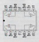
Compensated with LM324 pinout.
