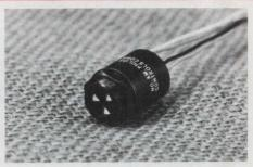
ELECTRIC RESET "BITE" INDICATOR Meets M83827/02. Monitors systems or components. Pinpoints malfunctions by providing automatic and permanent (until reset) warning of fault condition. Miniature size. Can be compactly grouped. 3 to 28V dc. 40 ms response. Wire leads or turret terminals. North American Philips Controls Corp., Cheshire, Conn. 06410.
