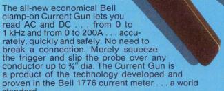
The Bell Current Gun has two ranges, 0 to 10A and 0 to 100A. Both have 100% overrange. Accuracy is ±2%. **Only three controls:** zero, range selector and press-to-read button for extra long battery life (batteries rated for 30 hours full-time use).
