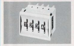
OMRON ECONOMY THUMBWHEEL SWITCHES. Cuts cost and assembly time with standard-size, snap-together, modular construction, plus snap-in mounting. Black or beige housings. Decimal or binary codes, with or without repeating terminals. Service life exceeds 100,000 mechanical operations. Continuous current of 1A at 28 VDC. Typical 4 digit assembly units measures 1.7" width  $\times$  1.3" high  $\times$  1.6" depth. OMRON ELECTRONICS, INC., 233 S Wacker Dr., Chicago, IL 60606. (312) 876-0800.
