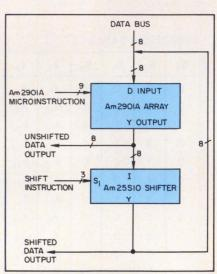
7. Connecting an 8-bit barrel shifter to a 2900-based processor requires that the input lines of the scalers be connected to the output port of the 2901A, and that the output lines of the 25S10 be connected to the data bus/input port of the 2901A.
