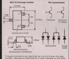
R joggle transistors are identified by a suffix R after the type number. Devices are identified by a code stamped on the body of the device.
