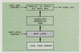
6. With pipelined memory organization, the total access time for the ROM and RAM combination is simply the longest of either rather than the sum of the two.
