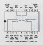
Compensated with offset control. Pin equivalents:  $\mu$ A747
