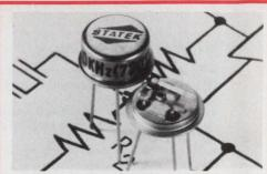
CMOS Crystal Oscillators in Low profile TO-5. Frequency range is 10 kHz to 300 kHz (divided outputs to 1 kHz, low as one cycle per month available). Low milliamp current consumption. Accuracy ±0.01%. Shock 1000 g. Hybrid thick and thin film chip and wire design is rugged and ideally suited for portable equipment. Details in Gold Book & EEM \* STATEK CORP \* 512 N. Main, Orange, Ca. 92668 \* (714) 639-7810 \* Telex 67-8394.
