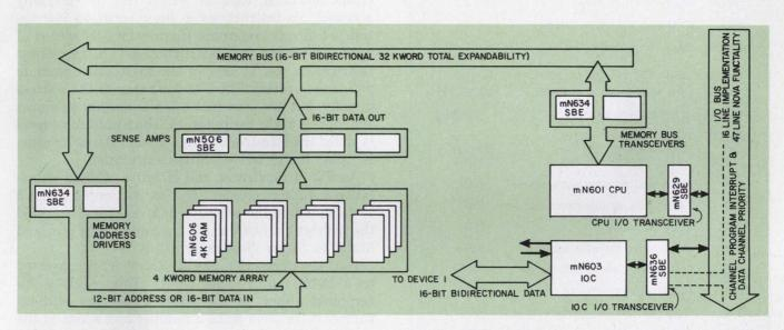
2. There are three major buses on the processor—the memory bus, the serial I/O bus and the control bus. And
