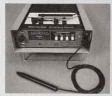
Tracking shorts and opens is simplified by sensing the phase of magnetic fields. This Model 2220 Bug Hound from GenRad has LED-lamp and audible indicators, as well as a microvoltmeter.
