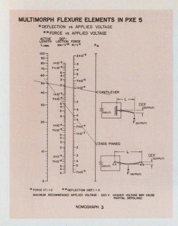
for an active length of 50 mm with a cantilevered configuration, you can obtain a deflection of  $1.8 \times 10^{-3}$  mm/V. With a supply voltage of 20 V applied to the outer electrodes a deflection of 0.04 mm (0.0015 in.) can be obtained. Higher drive levels can produce larger displacements, and nonlinear effects tend to increase the displacement.
