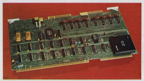
Compatible with Intel's SBC 80 microcomputers, Burr-Brown's MP8600 analog I/O board costs as little as \$198 (in quantities of 100) for a 16-channel input-only configuration.
