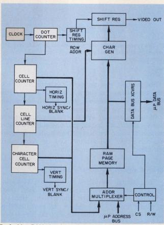
5. A video RAM circuit combines the sync generator with all the counting circuits, the character generator and the necessary memory pages to form an almost complete video display system.
