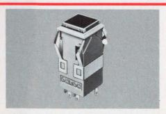
OMRON LIGHTED PUSHBUTTONS. Mechanical contacts or solid state Hall-effect outputs, choice of momentary or alternate action, SPDT or DPDT, for direct power switching or input to solid state switching. Available in solid state, gold alloy and silver alloy contacts. Standard T-1 3/4 incandescent bulb replaces with power on, no tools needed. Snap-in mounting, long life of 5 million mechanical operations. OMRON ELECTRONICS, INC. 233 South Wacker Drive, Chicago, III. 60606. Phone (312) 876-0800.
