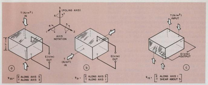
1. The piezoelectric constants and the stress and voltage axes are directionally dependent. Therefore they are indexed relative to the poling axis, which is by convention
