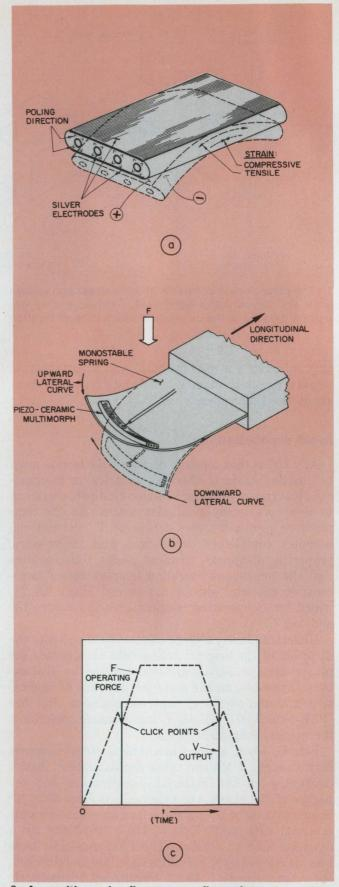
3. A multimorph flexure configuration, for piezo ceramics (a), is simpler to fabricate than a bimorph. Such a piezo element can be used to build a snap-action switch, when bonded to a cantilevered spring of special design (b). The spring's snap action provides a step-voltage output (c) and also a tactile feel.
