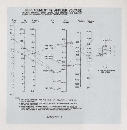
ever, since you must take care to prevent flashover along the ceramic's exposed surface areas, the applicable field is limited to approximately 900 V/mm. For an applied field opposite the poled direction, the maximum field is about 450 V/mm for PXE-5 to prevent depolarization.
