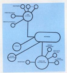
There's more than one way to distribute processing power through an organization. A hierarchically distributed structure (top) is simplest and easiest to visualize and expand. But some computer users, like oil companies, have systems so complex they can be represented graphically by only the most over-simplified diagram (center). Just one node of the oil company's processing system—distribution, for example—has a complex representation (bottom).
