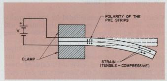
2. The flexure mode, as in this bimorph configuration, is used where larger deflections and smaller forces are involved than are possible with rings or discs.
