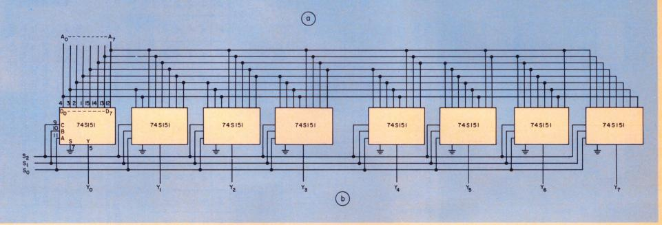
4. An end-around barrel shifter built from four scalers can handle an 8-bit data word and shift it 0, 1, 2, 3, 4,
