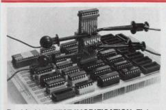
**Dual-In-Line TEST/MODIFICATION Fixture** Simplifies testing and provides a means for nondestructive circuit modification. DIP switches provide a means of isolating each circuit lead, test points are provided on both sides of the switches for testing or circuit modification. High rel components are used through out. 14 pin \$21.95, 16 pin \$22.95, 24 pin \$28.95, 40 pin \$40.95. Other sizes quoted on request. EMD Co., 7891 Camp Chaffee Rd., Ventura, CA 93001. 805-649-1513.
