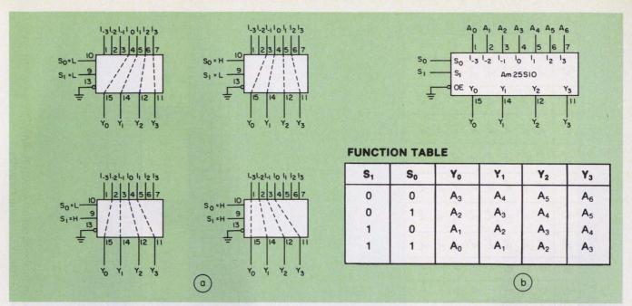
2. The four shift positions of the 25\$10 depend on just the  $S_0$  and  $S_1$  control lines (a). By representing the 7-bit
