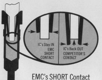
Many newer IC's have shorter or highly tapered leads. If plugged into longer standard terminal contacts, lateral pressure caused by the angle of the contacts vector into a constant potential ejection force. Add a
