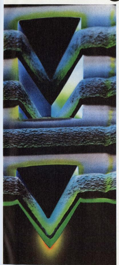
**AMI creates VMOS.** This revolutionary idea revolves around a three-dimensional transistor, etched into the silicon substrate.
