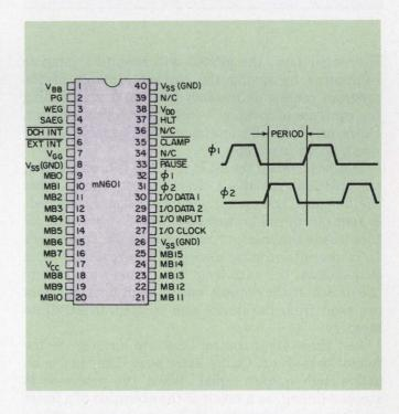
3. Of the 40 pins on the microNova, 16 are required by the memory bus, four are used for the serial I/O, eight for control, seven for power, two for the clock and three more are not connected (a). The two-phase nonoverlapping clock (b) controls all system timing.
