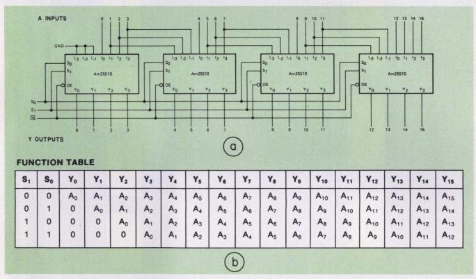
3. Shifting a 16-bit word up to four places, the scalers can be cascaded for almost any word length. When the
