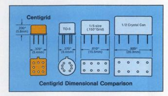
Out of Teledyne's TO-5 relay technology has evolved the Centigrid® - the ultimate subminiature relay. It combines the proven TO-5 relay design concept and internal construction into an even more compact package. Low profile height - just .230" (5.84mm) with terminals spaced on a .100" (2.54mm) grid permitting direct pc board mounting without the need for lead spreading.
