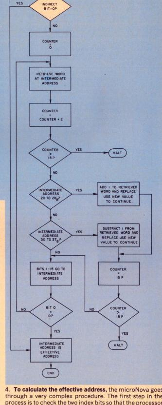
4. To calculate the effective address, the microNova goes through a very complex procedure. The first step in the process is to check the two index bits so that the processor knows what to do with the displacement bits in the instruction before performing the calculation.
