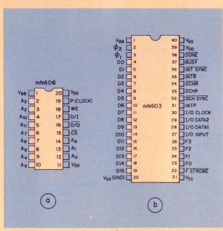
5. Housed in a 20-pin package, the 4-k dynamic RAM developed by Data General keeps the memory-support circuits needed by the processor to a minimum (a). The I/O controller circuit, housed in a 40-pin DIP, is almost as complex as the processor (b). One controller must be used with every peripheral device connected to the  $\mu P$ .
