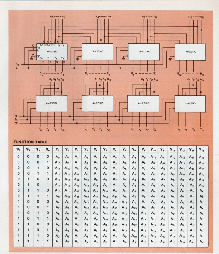
5. **Performing a 16-bit, two-level barrel shift** requires just eight 25S10s. By using a two-level approach, four control
