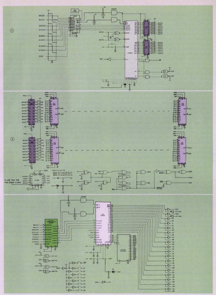
8. By combining a processor chip, two mN634 buffers, an mN640 clock driver and an mN629 transceiver, you
