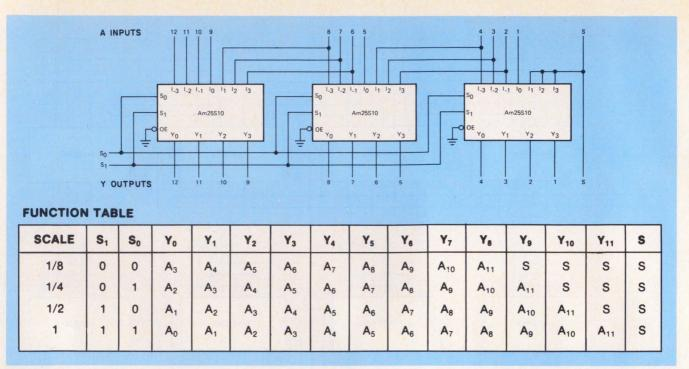
6. To do 2's complement arithmetic, a 13-bit scaler can be built from three shifters. Scale factors of  $\frac{1}{8}$ ,  $\frac{1}{4}$ ,  $\frac{1}{2}$  and
