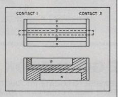
p-n junction diffusion potential of 0.52 eV. The capacitance/voltage curves of the Osaka diode (with a linear doping profile and gold contacts) reveals that the sensitivity of the capacitance to bias voltage variations ( $\lambda$ ) lies between 0.4 and 0.6. In the curves the capacitance was normalized to its zero bias value.
