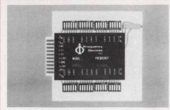
PROGRAMMABLE ACTIVE FILTERS provide a convenient breadboarding tool for designers. Series 744/FC102 are 4 pole lowpass filters with cutoff frequency (F<sub>o</sub>) that can be varied over a 500:1 tuning range in 0.2% increments via self contained programming switches. Ten models cover the frequency range from 0.1 Hz to 50 kHz with Butterworth and Bessel transfer functions. Frequency Devices, Inc., 25 Locust Street, Haverhill, MA 01830. (617) 374-0761.
