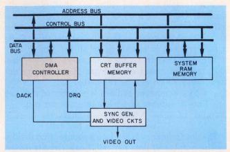
9. By using a DMA interface between the processor and the video display, the main system memory can be constantly updated then transferred to the display's buffer in one operation every time the display wants an update.
