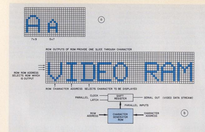
3. Standard 7×9 and 5×7-dot matrix displays can be generated from ROM-based data (a). To actually form the
