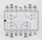
Compensated with RC4136 pinout.
