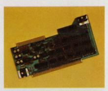
A low-cost analog I/O system from Cromemco has seven a/d channels and seven d/a channels. Compatible with the S-100 bus, it costs \$145 in kit form and \$245 assembled.
