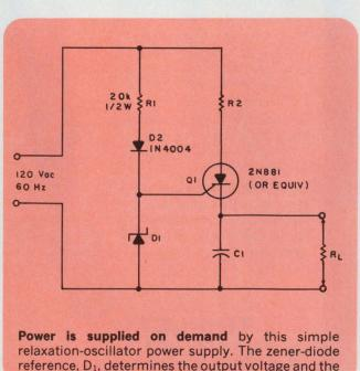
time constant of R<sub>2</sub>C<sub>1</sub> controls the amount of ripple.
