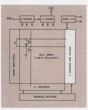
An Intel 2104A-style RAM with folded bit lines. These lines allow easy Y-access to both halves of a divided bit line.
