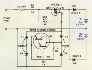
Battery-charger circuit charges two series-connected batteries independently with only one voltage-level adjustment, R<sub>4</sub>. Moreover, the circuit's temperature coefficient automatically adjusts for proper charging as the temperature changes.
