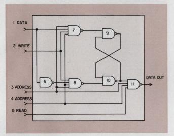
3. In the D-Lasar, the memory cells are interconnected by data (in and out), address, read and write lines.
