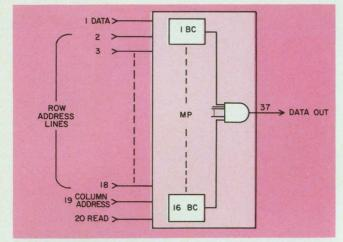
5. A memory-plane model reserves 16 lines for the row address, one for the column address, one for data output, and three for control.
