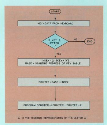
8. A more complex keyboard can also be handled by the processor. Just expand the table of look-up functions and allow enough space in memory.
