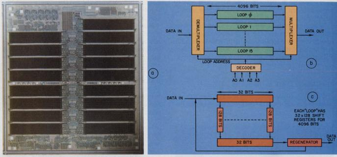
The advantage of CCD memories over dynamic RAMs is that about 70% of the chip area is used for storage, while dynamic RAMs use less than half. TI's CCD, the TMS-3064 (a), is organized as an array of 16 shift-register loops, each
