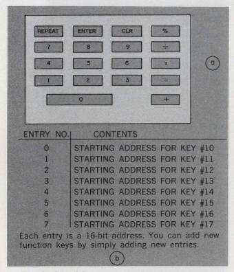
6. Even keyboard inputs can be handled by a table (a) since each key closure can be made to generate an index, which directs the processor to a particular subroutine.
