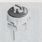
MINIATURE CERAMIC TRIMMER CAPACI-TORS 9371 series of ceramic trimmer capacitors are compact, economical and rugged. They are 50% smaller than other trimmers of this type yet provide high capacitance values. Available in 4 capacitance ranges, 1.5 to 4, 3.0 to 10, 3.5 to 18 and 5.0 to 25 pf with Q's > 300 at 10 MHz. They have an overall diameter of .225" with .215" above board height. JOHANSON MANUFACTURING CORPORA-TION, Rockaway Valley Road, Boonton, N.J. 07005 201-334-2676
