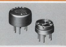
FIGARO GAS SENSOR TGS is a gas sensitive semiconductor. When combustible gas is absorbed on the sensor surface, a marked decrease of electrical resistance occurs. Major features of the sensor include high sensitivity, long term reliability and low cost. The applications are: GAS-LEAK ALARM, AUTOMATIC FAN CON-TROL, FIRE ALARM, ALCOHOL DETEC-TOR, etc. Figaro Engineering Inc., North America Office-3303 Habor Boulevard, Suite D-8, Costa Mesa, Calif. 92626 Tel: (714) 751-4103 Telex: 678396
