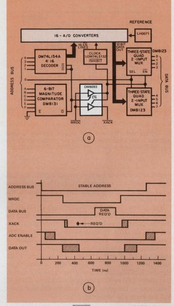
4. A data-ready signal MDRC returns to the 8080  $\mu$ P from the 16-channel parallel-conversion system (a) to prevent extending the Memory Access cycle. MDRC goes out on the XACK line at least 300 ns before it is needed (b).
