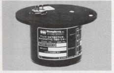
MAGNETIC FLUX DETECTOR . . . Provides continuous north reference. Has sensing element that uses standard flux gate windings suspended in a pendulous position. For use with directional gyros or servocompass systems. TSO C6c for use in autopilots. Model No. FD01-020-1 recommended for guidance and control systems on RPV's target drones, reconnaissance vehicles, oceanographic applications. 2.28" diameter x 1.91" high. Humphrey Inc., 9212 Balboa Ave., San Diego, CA 92123 Telephone (714) 565-6631.
