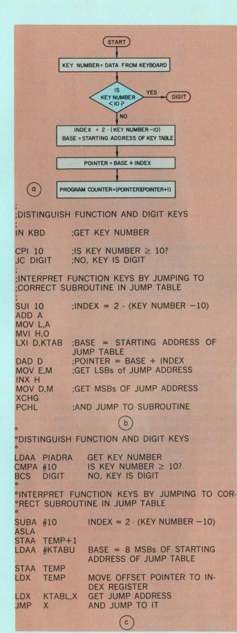
7. **To handle keyboard inputs**, the processor must make a decision and determine whether the key pressed is a number or a function (a). Both the 8080 (b) and the 6800 (c) can handle the task, as shown by these simple programs. An example, using one of the table entries, is also shown.
