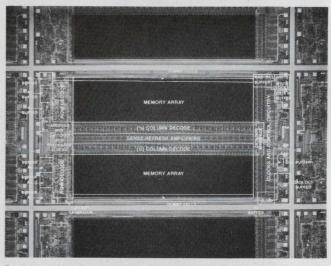
**1.** A combination of high speed and low power in this 16k Mostek MK 4116 dynamic RAM results from new approaches in the design of on-chip peripheral circuits and sense amplifiers.
