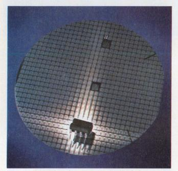
Nonvolatile semiconductor memories don't forget after the power is off. Nitron's 256-bit electrically alterable, read-only memory (EAROM) retains data for a year. Serial data input and output keep pin count low.
