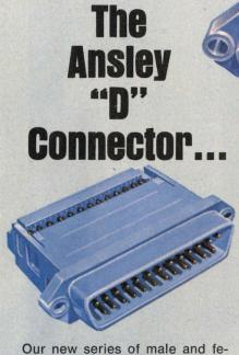
male "D" connectors offer you a cost effective external mass termination cable and connector system second to none. Its uniqueness begins with a one-piece "D" connector package that meets industry standards for size, pin spacing, and contact reliability. With no loose parts to match up, positive cable-to-contact alignment is assured. Conductors are mass terminated in seconds with our standard BLUE MACS™ hand or bench tools. The results? Faster installation, higher reliability.
