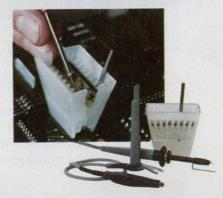
And here's something NEW for scopes. HP's **Easy-IC Probes.** A new idea for probing high-density IC circuits that eliminates shorting hazards, simplifies probe connection to DIPs and gen-
