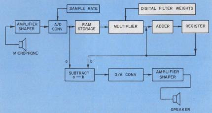
This digital audio processor is the first to operate in real time. Since it eliminates the conventional recording step required in other digital audio processors, it can be used in real-time communications systems.
