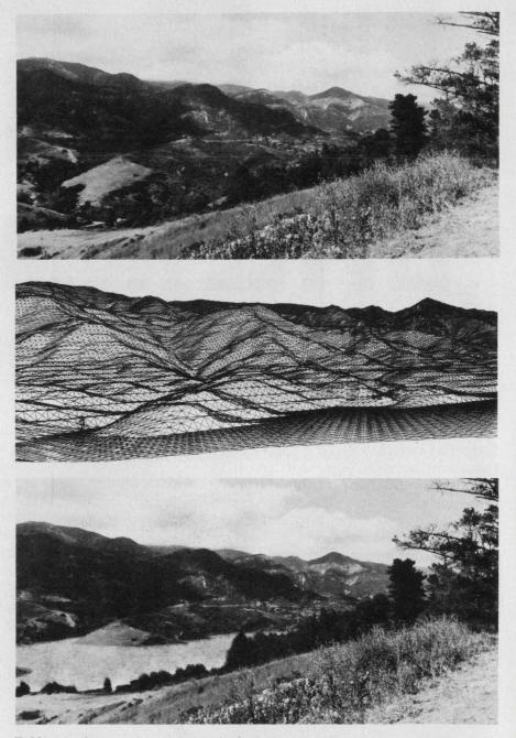
**Taking a picture of a lake that isn't there yet** is less costly than surveying, more accurate than an artist's concept and quicker than building a model. Photograph of actual site (top) is matched to a survey map of the area. The map is digitized along its contour lines, software-rotated to the camera's vantage point and outputted to a pen plotter (middle). A photographic process super-imposes the two into a montage; an artist adds color and texture (bottom).
