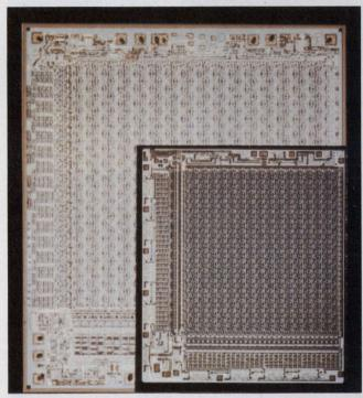
The size of the die directly affects the cost of a semi memory. The original design of this 1024-bit memory from Signetics is shown in the background; it requires 25,000 sq mil of silicon. The present design, shown in the foreground, is only 14,500 sq mil. Data sheets often indicate the die size.
