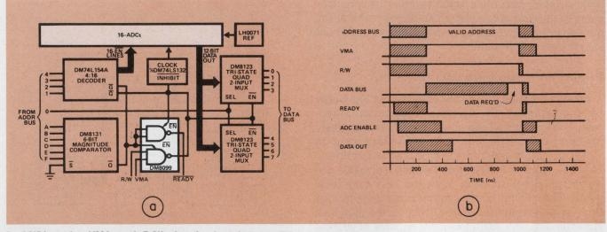
5. ANDing the VMA and R/W signals decodes a valid address in the 16-channel parallel-conversion system for the 6800 microprocessor (a). Address information, the
