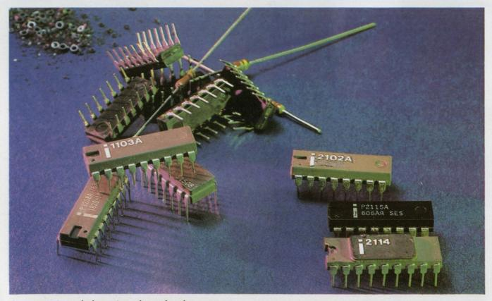
**Memory-systems design gets easier and easier,** as you go from core to dynamic then static semiconductor RAMs. Dynamic MOS-memory design is no cinch, however—it takes TTL-to-MOS level shifters, output sense amplifiers and a handful of parts to refresh the RAM. Static RAMs at right are the easy way out (Intel).
