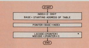
\*The Intel 8080 generally stores 16-bit numbers or addresses with the LSBs first while the Motorola 6800 stores them with the MSBs first. LSCODE and MSCODE are thus reversed in 6800 memory.
