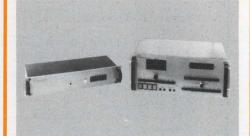
**COMPUTER PROGRAMMABLE MAGNETIC FIELD CONTROLLER.** Model FFC-4DP can interface with most regulated power supplies and virtually any computer with 6 decades of BCD output. Offers 1 part in  $10^6$  full range setting of field amplitude of an electromagnet. Manual input also provided. Features stray field compensation and elimination of hysteresis effects and temperature gradient effects. Many applications. Write: Walker Scientific, Inc., Rockdale Street, Worcester, MA 01606
