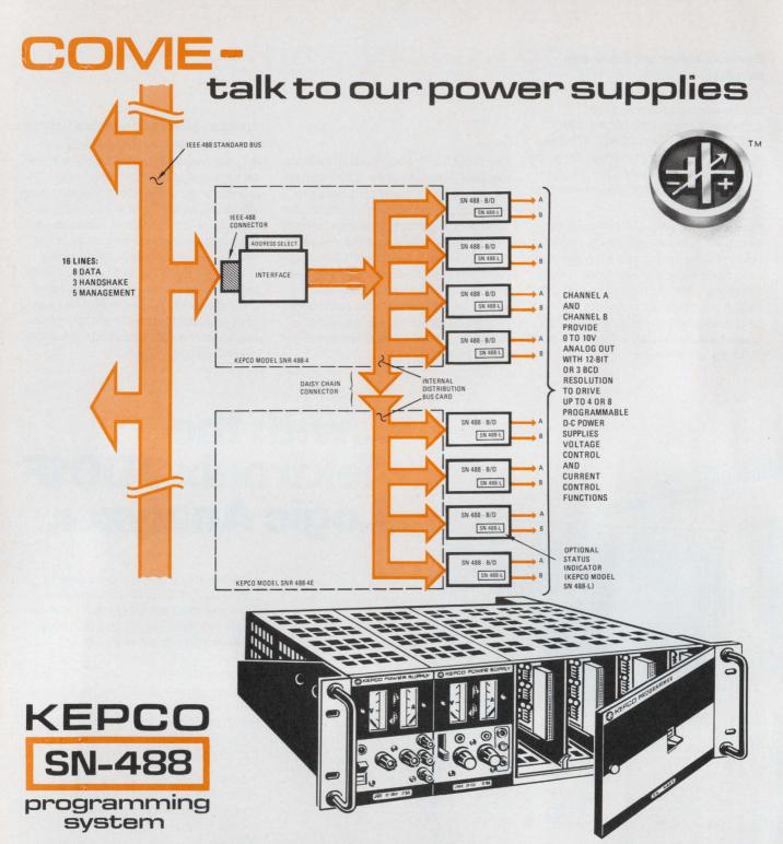
Kepco's new SN-488 digital interface provides you with a convenient way to put our programmable power supplies on your General Purpose Interface bus. The model SN-488 responds to the "listen" instruction, provides the "handshake" interaction and gives you two addressable channels on each card. Up to eight cards can be addressed through a single bus connector.
