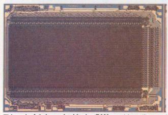
**This colorful dynamic, bipolar RAM** combines the good attributes of bipolar technology (5 V, 280-ns t<sub>cy</sub>, 120-ns t<sub>acc</sub>) with low MOS power (350 mW active), and high density (4096  $\times$  1 bits). Fairchild makes this memory with isoplanar integrated injection logic.
