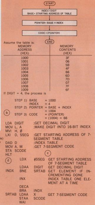
language programs for the 8080 (c) and the 6800 (d and e) require less than 10 lines of code. Note that # indicates "immediate" and X means "indexed" on the 6800 assembler. Also, 0, X can be abbreviated to just X.
