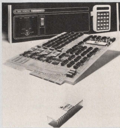
The microNova family consists of chip set, board computer and fully packaged minicomputer.
