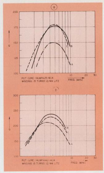
9. Q curves measured on two 1408 pot core sets in 4C4 nickel zinc material with  $A_{\rm L}$  of 25 (a) and  $A_{\rm L}$  of 40 (b).
