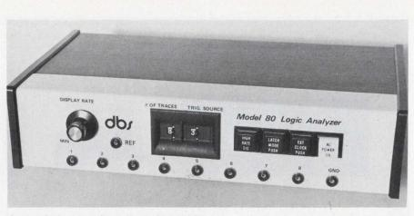
A stand-alone analyzer from Digital Broadcast Systems delivers a multiplexed signal to an external scope.
