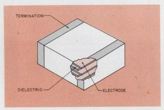
2. Multilayer ceramic capacitors are fabricated by stacking and co-firing thin sheets of metalized green dielectric.
