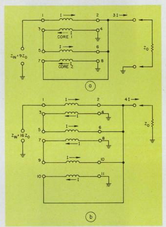
2. Two cores are required in a transmission-line transformer to achieve a 9:1 impedance ratio (a). Three cores are required for a 16:1 ratio (b).
