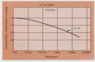
5. Electrical characteristics for Class II capacitors vary widely with temperature, offered voltage and frequency.
