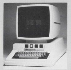
The M-8 Educator development system, designed by Technical Communications Inc. (P.O. Box 306, Olathe, KS 66061. 913-764-0243), provides a CRT communications terminal and  $\mu$ P controller in one unit. The system is built around the Fairchild F-8 microprocessor and includes a 53-key (Hall-Effect) keyboard, 64-character-by-31-line CRT display, 110-baud TTY-compatible serial I/O, 300 or 600-baud TTL serial I/O, composite video output signal for remote CRT and 2-k of RAM, expandable to 32-k.
