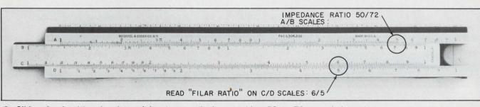
8. Slide-rule algorithm for determining turns ratio for matching 50 to 72  $\Omega$ , unbalanced.
