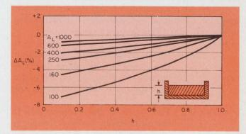
4. If less than the total bobbin height is used, the actual inductance will be lower than the calculated value. The larger the air gap, the greater the deviation.
