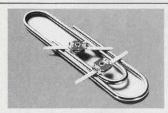
Thin-Trim variable capacitors provide a reliable means of adjusting capacitance without abrasive trimming or interchange of fixed capacitors, Series 9401 has high Q's and a range of capacitance values from 0.2-0.6 pf to 3.0-12.0 pf and 250 WVDC working voltage. Johanson Manufacturing Corporation, Boonton, New Jersey (201) 334-2676.
