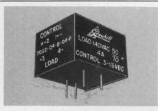
SPACE-SAVING 4 AMP SOLID STATE RE-LAY occupies only 1 cubic inch, is logic compatible, with switching capability from 0.1 to 4 amps, rated @25°C. Optically coupled; zero voltage turn-on. Offers inductive load switching, excellent transient protection. PC mountable. Prototype quantities from stock. Grayhill, Inc., (312) 354-1040.
