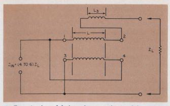
3. To extend a 4:1 impedance ratio to 6:1, a third winding,  $L_3$ , is wound over the original winding, L.
