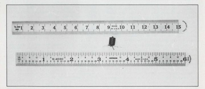
15. The compact 5.5- $\Omega$  to 50- $\Omega$  transformer uses a trifilar winding, with the strands connected series-aiding.
