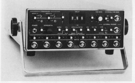
**Glitch detectors,** such as the one found in the BP Instruments 20-D, bring some of the analog scope's capabilities to the analyzer.
