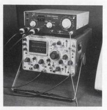
**Testing in the field** is the forte of the Digital Laboratories DSR 505, a twochannel analyzer.
