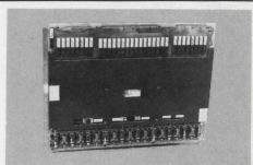
**16K/32K Memory Systems.** Model 696: 16K, 18-bits; to 256K X 9, 128K X 18, 64K X 36. Model 698: 32K, 18 bits; to 512K X 9, 256K X 18, 128K X 36. Cycle 650 nsec, access 250 nsec. Dir. rplcmnts for Micro 3000. Fabri-Tek, Inc., 5901 S. Cnty. Rd. 18, MpIs, MN 55436 (612) 935-8811
