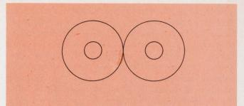
13. Two toroidal cores placed side by side offer a better form factor than a simple toroid.
