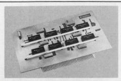
EASIER ECL VOLTAGE AND GROUND DIS-TRIBUTION SYSTEMS—Reduced system noise, high packaging density and less design time for PC boards with ECL circuits are yours with Mini/Bus®, the Rogers way to eliminate the cost of multi-layer boards by off-board voltage and ground distribution. Rogers Corp., Chandler, AZ 85224 (602) 963-4584.
