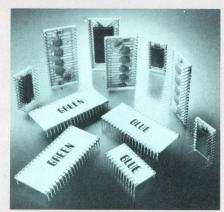
data I/O. Another Blue chip (the IPC-16A/502) generates system timing. Gold-chip memories include  $256 \times 4$ -bit static RAM (IPC-16A/504), 16-k bit ROM (IPC-16A/505), 4-k bit electrically programmable PROM (IPC-16A/506) and 4-k bit ROM (IPC-16A/507). Interface latch elements—Green chips—consist of eight (ILE/8) or 16 (ILE/16) dual port flip-flops in a single package.
