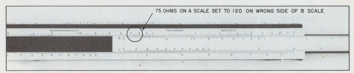
12. An incorrect turns ratio will appear if the wrong half of the A or B is used.
