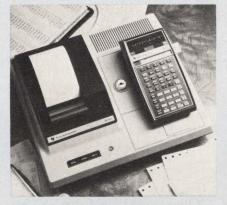
**Texas Instruments SR-52** programmable calculator is converted into a desktop printing unit.
