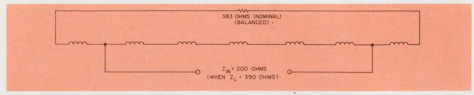
11. A seven-winding autotransformer is needed to match 383 to 200  $\Omega$ , both balanced to ground.
