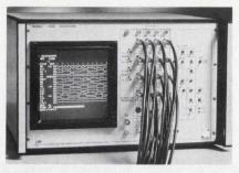
**Alphanumeric readout** plus a timing diagram are characteristics of the AMC 1320 Digiscope, from E-H Research Laboratories.
