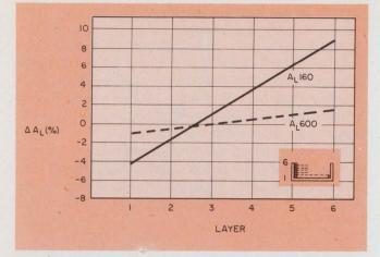
5. The position of layers of turns on a pot core introduces still another deviation between actual and calculated values. Layers 1 and 2 have less than average inductance, while layers 3 to 6 have more than average inductance per turn.
