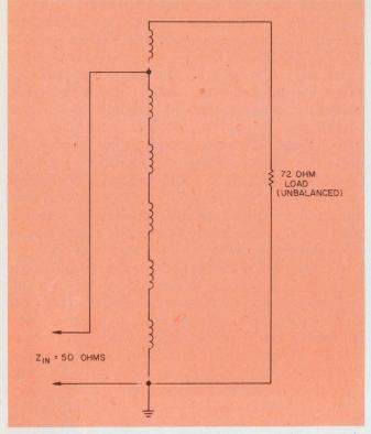
9. A hexafilar winding is used in this example to match a 72- $\Omega$  load to a 50- $\Omega$  cable.
