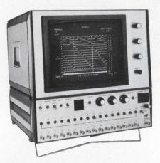
Taking aim at  $\mu$ Ps is the Model 16. from Vector Associates, a 16-channel unit with a microproceseor I/O.
