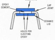
Various types of DIP packaging are utilized of which the molded and "sandwich" types seem most common. One problem that frequently occurs with the sandwich types is delaminating. This happens when air in tiny voids remaining in the epoxy filler (bonds the substrate to the sandwich "lid") expands in hot operating environments to the extent that the package comes apart and fails.
