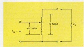
1. In a basic autotransformer used for impedance stepdown,  $Z_{in} = k^2 Z_{out}$  where k is the location of the tap.
