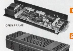
**FOR THE OEM,** PCX are available as an open frame module with a massive heat sink that requires no other cold plate for non-derated operation to +71°C.
