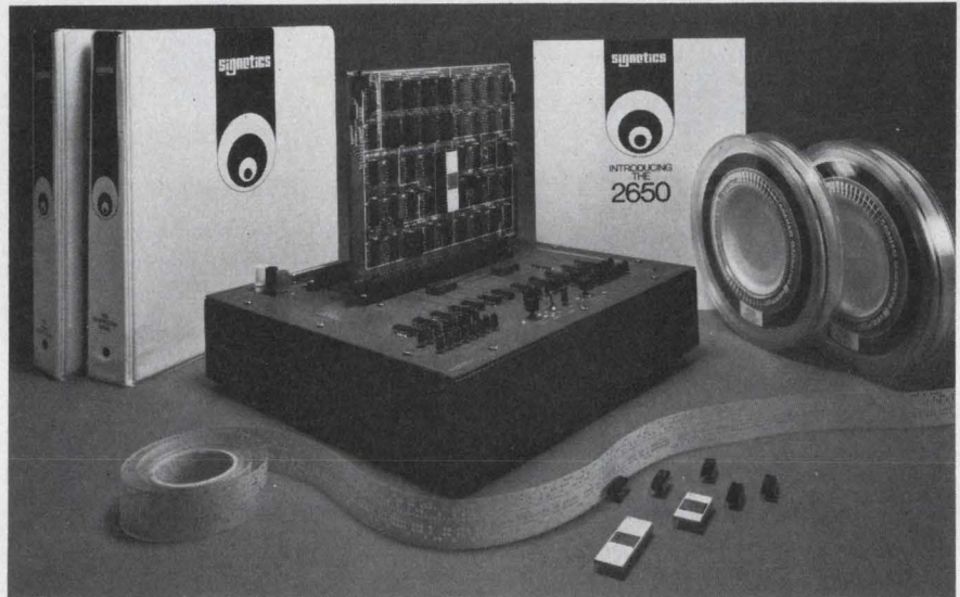
A $155 kit for the 2650 microprocessor includes the CPU, PROMs, interface circuits and a board. Signetics offers the kit along with other design aids (some are shown) for the company's 8-bit NMOS micro.
