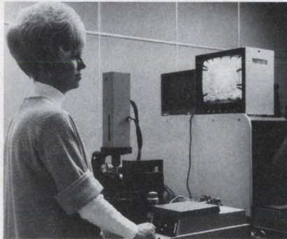
Motorola laser trims diffused resistors to adjust the ladder network of the MC3510 10-bit d/a converter. The operator follows a bright spot on the TV display to position the laser beam on the chip. The resulting IC converter has a maximum linearity of \pm 0.05\% .
