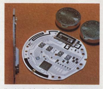
**Use of tuning-fork crystals in electronic watches** is on the rise. On this chip a Statek crystal is sealed under a glass cover through which the crystal is laser-trimmed.
