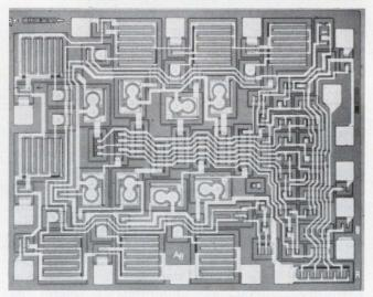
**By combining bipolar drivers and JFET switches** on the same monolithic chip, National Semiconductor achieves vastly improved resistance characteristics. The LF 11305, an 8-channel multiplexer, specifies resistance variation as a mere 1% over the input-voltage range.
