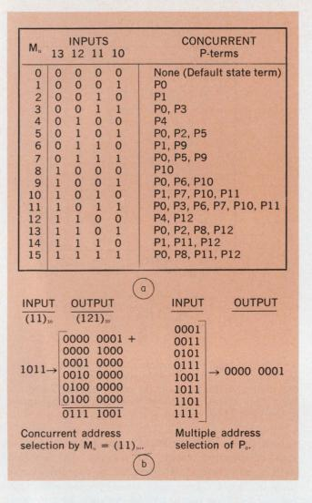
5. The simultaneous selection of P-terms with a minterm generator (a) reveals an FPLA's concurrent and multiple addressing-mode capabilities. In concurrent addressing, a single input selects several words (a). Multiple addressing leads to the selection of a single word by several input combinations (b).
