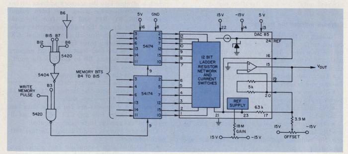
5. D/a converters can be interfaced easier than a/d's. All you need are several gates to enable two hex D flip-
