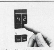
Solid-State Digital Advance Switch-The thumbwheel switch you activate with only a TOUCH! No rotating of cumbersome ratchet wheels. Simply touch the "touch plate" and the switch advances, step-by-step, until you remove your finger. Stepping rate 0.3 seconds/digit. Master Specialties, 1640 Monrovia, Costa Mesa, Calif. 92627. 618
