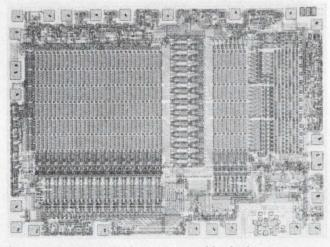
**One of the first field programmable logic arrays** was this IM 5200 from Intersil. It can accommodate as many as 14 inputs and eight outputs. Fusible links are used.
