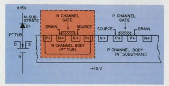
By not tying the n-channel body to the negative supply, Intersil achieves an overvoltage tolerance of up to 10 V in excess of either supply. The body voltage comes from a diode structure that connects to the positive supply. Called floating body, the technique is used in the company's line of CMOS switches such as the IH 5040, a single-pole, single-throw circuit. Intersil also offers a series of floating-body multiplexers.
