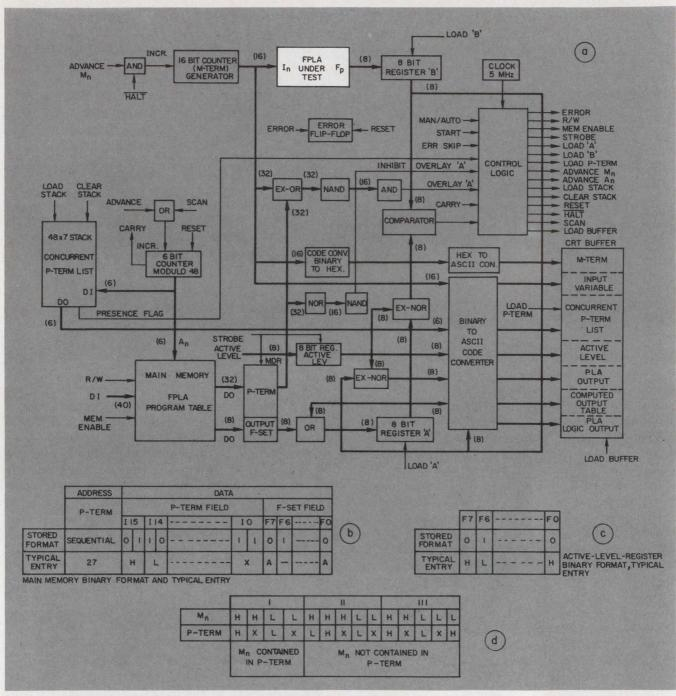
11. A hardwired algorithm (a) performs the logic-verify test sequence. The algorithm manipulates program-table data stored in both main memory (b) and the active-level
