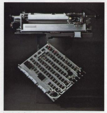
Interdata's Carousel printer is the first microprocessorcontrolled serial printer. It prints at 30 cps.
