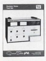
The Model 315B is designed to make resistor NOISE INDEX measurements in accordance with the recom-mendations of the National Bureau of Standards. (Method 308 of MIL-STD-202B). NOISE INDEX is defined as the measured ratio of microvolts of noise per volt of ap-
