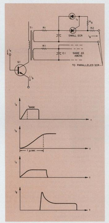
**3. A pulse-sharpener circuit** helps reduce the mismatching effects of differences in SCR turn-on delays when the thyristors are operated in parallel.
