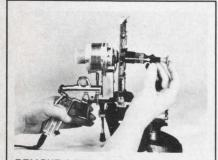
REMOVE-A-DIP, 14/16 pin IC desolder, remove and self contained vacuum system for cleaning solder out of the plated through holes. Works from solder side of PCB so high density is no problem. MICRO ELECTRONIC SYSTEMS, INC. Danbury, Ct.
