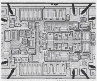
A dual single-pole single-throw CMOS switch—the HI-200 from Harris Semiconductor—features ON resistances of less than 100  $\Omega$ .
