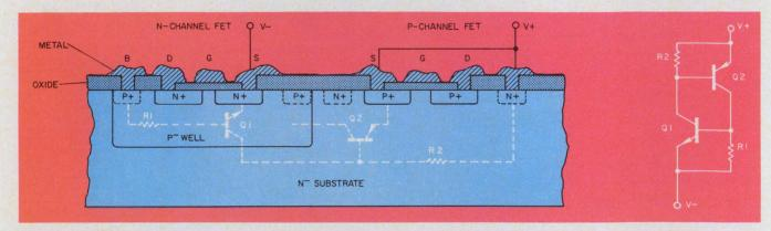
**Parasitic pnp and npn devices form an SCR,** or pnpn diode, in conventional CMOS structures. One or more forward-biased pn junctions trigger the SCR, which then
