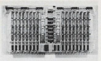
A CCD memory system capable of storing 128 kilobytes of data has been constructed by Intel from 64 of their 16-k serial memory chips. The 16-k CCD memory chips are designated 2416 and are available.
