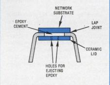
Various types of DIP packaging are utilized of which the molded and "sandwich" types seem most common. One problem that frequently occurs with the sandwich types is delaminating. This happens when air in tiny voids remaining in the epoxy filler (bonds the substrate to the sandwich "lid") expands in hot operating environments to the extent that the package comes apart and fails.
