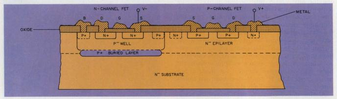
With the addition of a buried layer beneath the n-channel body, the product of npn and pnp-device betas can be slashed to less than unity, the minimum needed for
