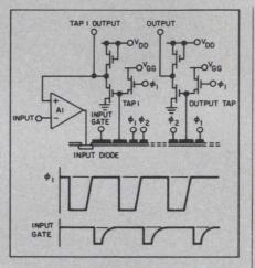
appears to be a disadvantage, in applications such as recursive filtering a differential amplifier is essential. Consequently when the amplifier is introduced with a CCD, it allows other signal-processing functions to be performed, such as signal summation and multiplication. The differential amplifier should preferably be produced so that it can be integrated monolithically with the CCD.
