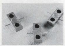
Hermetic stripline packages from Hewlett-Packard allow broadband performance to 18 GHz. They can be matched to 50  $\Omega$  at both input and output.
