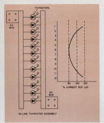
6. An in-line bus assembly for paralleling SCRs provides a  $\pm 20\%$  current mismatch.
