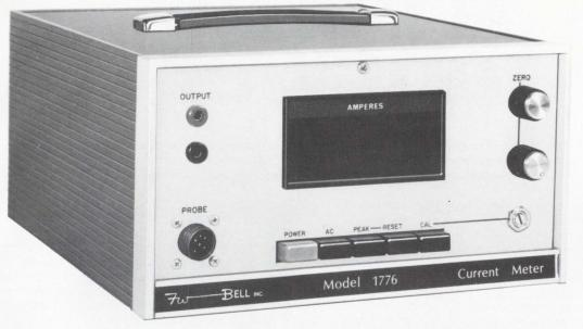
The Bell Model 1776 digital current meter provides features never before available. For example, its ability to measure ac, dc, (and ac on dc) currents with a non-contact clamp-on probe. No longer is it necessary to break the circuit to make a current measurement! This time-saving feature alone is extremely useful in the troubleshooting, repair and design fields. Now, it is possible to obtain current measurements more easily and safely than voltage measurements. And that's not all!
