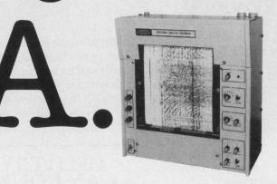
The new 19" rack-mounting SPECTRUM ANALYSIS RECORDER from Raytheon. It's the first dry paper line scanning recorder specifically developed for direct plug-in operation with commercially available spectrum analyzers.
