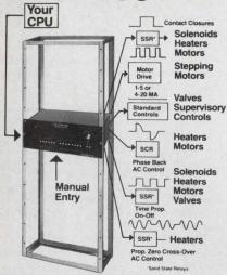
UNI-DRIVER, the one standalone interface between your computer and all commonly used final control elements. It maintains process control at the last command level, even with the computer shut down, and provides "back up" manual control.
