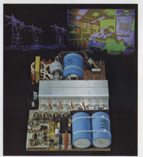
**Fast-switching transistors,** power Darlingtons and Schottky diodes are key components in high-efficiency power supplies, like this 1000-W off-line unit designed by TRW Power Semiconductors. Efficiency is better than 80%.
