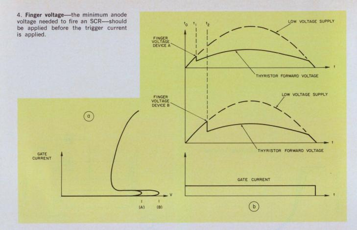
The effects of turn-on delay can also be reduced by use of input trigger pulses that have steep leading edges. This ensures that the SCR's trigger gate current rises above the trigger point of the least sensitive SCR before the SCR's builtin delay period ends. Note that if the squaring, or pulse-generating, circuit is directly coupled to the SCR, input isolation transformers don't have to pass the high frequencies required to generate the steeply rising pulses (Fig 3).
