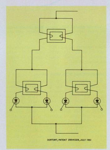
5. Equal current flow in the SCRs is forced by this arrangement of balancing reactors.
