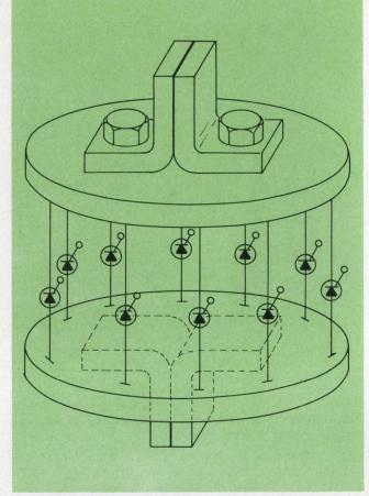
8. A cylindrical assembly should theoretically provide the most uniform current distribution among paralleled SCRs because of the configuration's symmetry.
