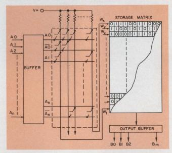
2. An internal programmable address matrix is the source of an FPLA's logic-compression capability. The matrix can choose a small fraction of a large number of input states.
