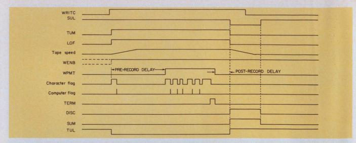
2. Write One Record—a typical command—begins with the tape initially at rest (tape torque is low). The first set of raised signals causes the tape to be moved forward and erased. This pre-record delay allows the tape to come up to speed and generates an interrecord gap. With the raising of Computer Flag, the first data character transfers from the computer to the controller, where it is held temporarily in a buffer register.
