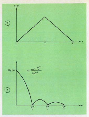
2. The over-all delay line has a triangular impulse response (a). The corresponding spectrum exhibits the characteristic of a matched filter with a 1/T bit rate.
