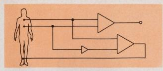
10. To cut common-mode noise, you can detect the unwanted signal, then vary a reference signal—usually derived from the right leg—at the same rate as the noise. The differential amplifier thus "sees" no common mode at its front end.
