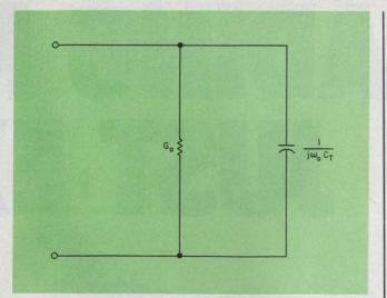
4. A surface-wave transducer can be represented by this equivalent circuit.
