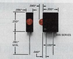
LED logic state fault indicators available in 14 models with voltage ratings from 1.7 to 14. Suitable for dense packaging on printed circuit boards—up to 10 units to the inch-IC compatible. With built-in series resistor. Polarity identified. Low power consumption.
