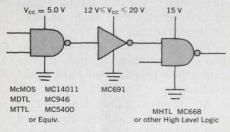
The MC696 Dual Interface Unit, Line Driver/Receiver offers flexible hysterisis capability for design variety. And has low output impedance of  $\approx 20$  ohms in LOW state.
