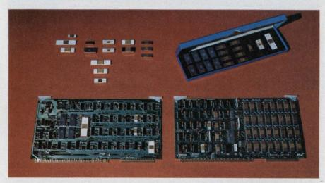
**Intel's popular 8080, 8-bit n-channel MOS microprocessor** can also be bought at many levels of integration. The chips are available to designers who choose to assemble their own boards. Or a small prototyping kit can be purchased. In addition larger boards are sold, with all the associated circuitry to make a complete CPU or add-on memory boards.
