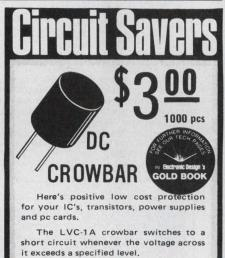
Any trip voltage level between 4.7V and  $200V \stackrel{+}{-} 10\%$  can be selected. The unit will handle a peak current of 50 Amps (8ms) and 3A continuously. MIL Temperature range, Call Mike Coyle for applications assistance.
