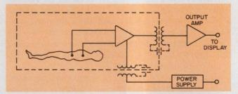
9. Present practice aims to isolate as much as possible the patient and instrument front-end from all external electrical sources. Thus input power and output signals are coupled with high-isolation devices.
