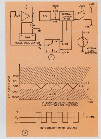
2. Code centers can be determined by use of a digital comparator and feedback to an integrator (a). The integrator's output ramps up or down, depending on where the comparator sets the solid-state switch (b). The manual switch is set by the user to an arbitrary code.
