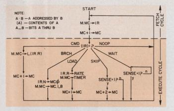
4. In the execution of an instruction, the contents of memory location M, addressed by counter MC, are loaded into instruction register IR. Then the register's contents are decoded, and the diagram branches according to instruction. All instructions are fetched in one clock time, and all except WAIT are executed in the next clock time.
