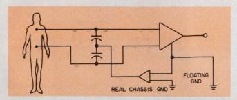
11. Still another way to discard a common-mode signal: Drive the junction of two capacitors with a signal 180degrees out of phase with the noise.
