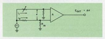
4. Unbalanced impedances in the two input legs of the amplifier cause unequal currents to flow into each leg. As a result, a portion of the common-mode noise is converted to a differential signal, which is then amplified and delivered at the output.
