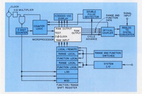
In the first LSI microprocessor-based digital voltmeter, from Systron Donner, the computer-on-a-chip, plus memory ICs, replace all the d'gital logic ordinarily used in such an instrument. Benefits include self-calibration.
