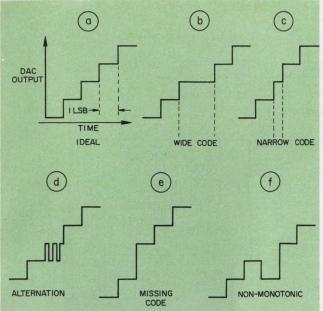
5. Various displays depict uniform excursions of an ideal a/d (a), wide and narrow codes (b and c), alternations (d), missing codes (e) and nonmonotonicity (f).
