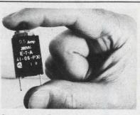
**Overcurrent Protector,** manual reset eliminates fuse replacement. Convenient panel mounting. 15 fractional ratings from 0.1 to 3 amp. Other models up to 400 amp. Tripfree and fool-proof, UL and CSA approved. High quality, low cost \$1.29 ea. in 1000 lots. E-T-A Products Co. of America, 7400 N. Croname Rd., Chicago, III. 60648. Tel: (312) 647-8303. Telex: 253780. CIRCUIT BREAKER <u>616</u>
