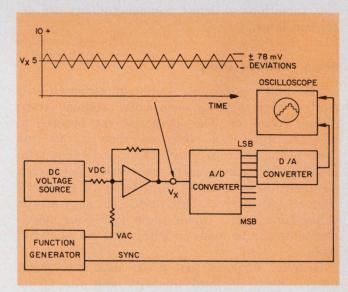
3. With a scope, you can observe and measure the switching points around a major bit, set by  $V_{\rm de}$ . A triangle,  $V_{\rm ae}$ , is added to  $V_{\rm de}$  to exercise the LSBs around the set point. The d/a converter changes the information back to analog for display.
