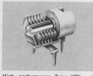
High performance Type "T" subminiature machined-plate capacitors. Rotors and stators machined from solid brass extrusions provide excellent stability and uniformity. High Q, low temp. coefficient (plus  $30 \pm ppm/^{\circ}C$ ). Available in horizontal and vertical tuning for PC and stripline mounts. E. F. Johnson Co., Waseca, MN., (507) 835-5222. TYPE "T" CAPACITOR 606
