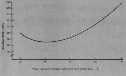
battery-powered equipment, reduces other component costs, because less drive current is required, and significantly lowers the cooling load. Reliability also is improved, because of less thermal stress on the transformer and adjacent components, and smaller parts can often be used.
