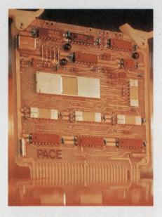
National Semiconductor's Pace microprocessor was the first 16-bit micro on a single chip. It comes in chip form, on a board with some memory (shown here) and also packaged into a prototyping system. such things as working in a harsh environment, very small space or at a very low power.
