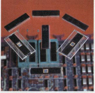
Western Digital produces a chip set that is used by Digital Equipment Corp. as the heart of the board-level microcomputer, the LSI/11. These chips allow Digital Equipment to market a 16-bit PDP-11 minicomputer on a board.
