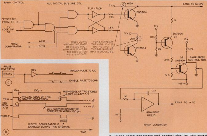
8. **Timing control of the tester** (a) synchronizes the various circuit elements. Timing relationships of the various signals are shown in "b."
