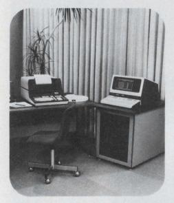
9882A subsystem (right) provides CRT and high speed data entry for 9830A calculator (left). Mass memory, below 9882A, has 4.8M bytes memory.
