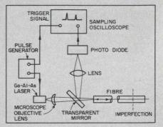
Telefunken researchers use a microscope objective to focus the laser light onto the end of the fiber under test. Between the microscope objective and the fiber, the front surface of a transparent mirror picks up light reflected from the fiber front face, from the fiber imperfection and from the far end of the fiber. This reflected light is focused onto an avalanche photodiode, and the detector output is displayed on a sampling oscilloscope.
