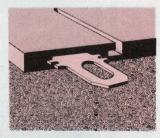
the terminals. It is not necessary to tape the start lead since it comes to the top of the coil through the slot and is thus separated from the winding. Separate lead wires or terminal boards and the extra assembly time to use them are eliminated.
