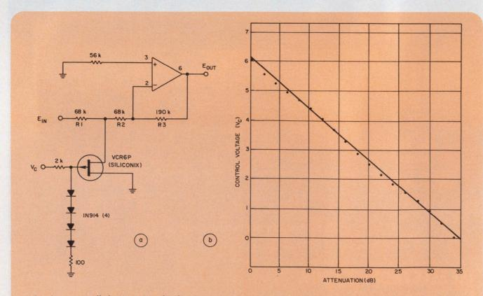
A voltage-controlled attenuator circuit (a) can provide linear dB variations (b) when the nonlinearity
