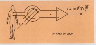
7. Loops in connecting leads should be avoided, since stray fields can couple and induce unwanted voltages into the input. Molded leads avoid the problem.
