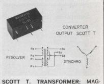
NETICO Synchro driver is 7/8 x 1-5/8 x 11/16 high, rated at 1 volt amp., 2 arc minutes accuracy. P.N. amp., 2 arc minutes accuracy. P.N. 52155 is 5.9 sine and cosine to 11.8 v. L-L Synchro. P.N. 52156 is 5.9 sine and cosine to 90 v. L-L Synchro. MAGNETICO, 182 Morris Avenue, Holtsville, N.Y. 11742— 516-654-1166. 607
