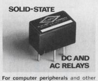
high-speed, high-reliability switching jobs, with either DC or AC loads up to 6 amp, these transformer-coupled Heinemann relays offer highest sensitivity and control-to-output pulse-shape conformity for TTL and other low-level control signals. Heinemann Electric Company Trenton, NJ 08602. 602
