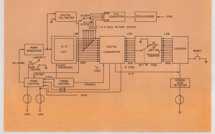
7. The complete a/d converter tester, with all additions and modifications, can determine converter errors in several ways. Code centers are measured with the digital
