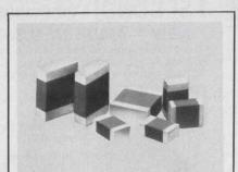
HIGH O MULTILAYER CAPACITORS feature very high quality factors at microwave frequencies. Offered in three standard sizes: .050 x .040, .080 x .050, .125 x .095. Capaci-tance values from 0.1 pf to 1000 pf with close tolerance and voltages to 1000 VDCW. Johanson/Monolithic Dielectrics Div., Box 6456, Burbank, Ca. 91510, (213) 848-4465.
