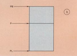
7. A code segment table (CST) keeps track of program segments in main memory (a). The stack simplifies this virtual memory operation, because program and data are separate. Three registers, PB, P and PL, protect and manage the code being executed (b).
