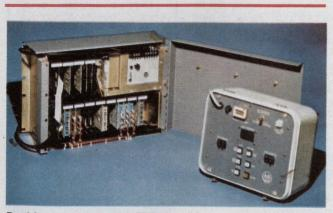
**Pushbutton programming on this programmable controller** made by Allen-Bradley, the Bulletin 1755-Mini-PMC, can sequence 62 input/output functions.
