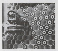
Vast amounts of data can be stored on data cartridges housed in the honeycomb storage compartments of the IBM 3850 mass storage system. Two cartridges can store the same amount of data as one disc pack.
