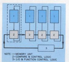
A simple arrangement for a sorting memory is shown above. A segment of the bus is extended to become a memory segment. This consists of a memory unit and the compare and control logic. An additional segment is used as the input-output unit.
