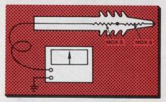
MAXI-MOX resistors have full-load drift less than 1% in 2000 hours of operation, and are available in tolerances of 1, 2, and 5% in values from 10K to 2,500M ohms. A silicone varnish conformal coating provides environmental protection while allowing a maximum hot-spot temperature of 220°C.
