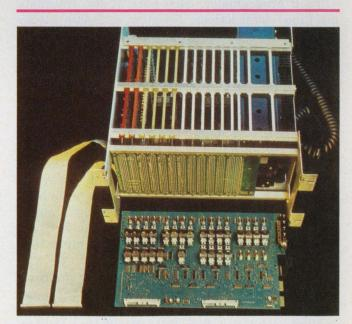
A microprogrammable mini from Interdata employs a push-down—or last-in, first-out—stack architecture to simplify use of high-level language and its compiler.
