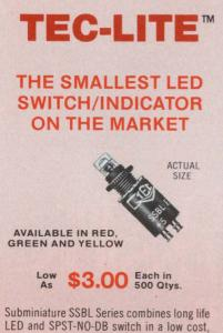
highly reliable unit that fills a variety of display and control functions-especially where space is limited. Projects only 5/8" behind panel with turret lug terminals (as shown) or 1" with .025" square Wire-Wrap terminals. Mounts in 1/4" hole on 3/8" centers.
