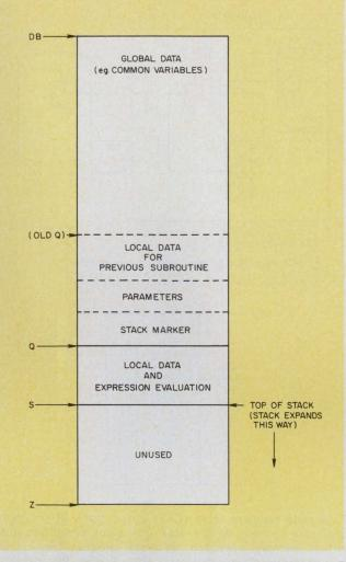
6. Four registers control stack boundaries. DB and Z limit the stack to prevent interference between users. Q indicates the data base for a currently executing routine, and S follows the changing stack size.
