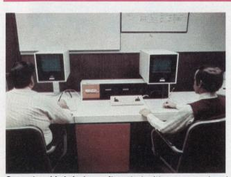
**Computer-aided designs often start** with a spec and end with complete PC board layouts. RCA uses Applicon graphics terminals to master the layout problems associated with complex MSI and LSI components, after CAD programs verify the design.
