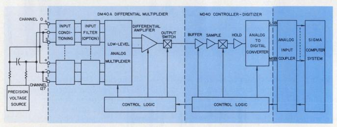
1. To check out a data-acquisition unit, set up a simulated system configuration and apply a precision voltage
