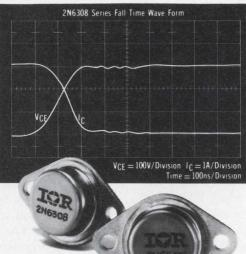
**Glass Passivation – Long Term Reliability** . . . high reliability and long term stability is achieved by hard glass passivation. Also, if you're using chips to make your own circuits, IR's glass passivation gives you the most stable, easy to assemble
