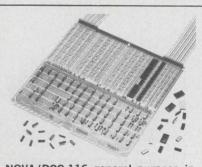
NOVA/DCC-116 general purpose interface board provides: multiple device selection, 4 I/O registers, DMA zero word count detect, 105 socket positions for 14, 16, 24 & 40 PIN IC's. Basic board (all features of data general 4040 plus multiple device select) \$350. MDB Systems, Inc., 981 N. Main St., Orange, CA. (714) 639-7238.
