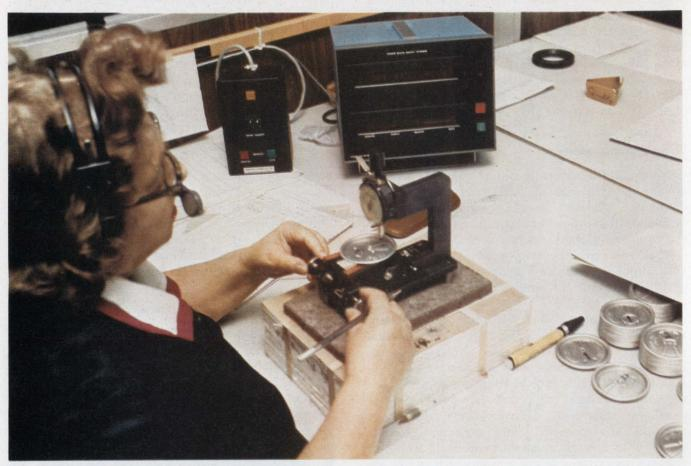
Voice-input systems are being used at Continental Can Co. to enter quality-control data into computers. An inspector makes several measurements on pull-top lids and enters the data by voice into Threshold's VIP 100 system, which prepares punched tapes. A computer then determines if quality control is satisfactory.
