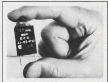
**Overcurrent Protector,** manual reset eliminates fuse replacement. Convenient panel mounting. 15 fractional ratings from 0.1 to 3 amp. Other models up to 400 amp. Tripfree and fool-proof, UL and CSA approved. High quality, low cost \$1.29 ea. in 1000 lots. E-T-A Products Co. of America, 7400 N. Croname Rd., Chicago, III. 60648. Tel: (312) 647-8303. Telex: 253780. INFORMATION RETRIEVAL NUMBER 609
