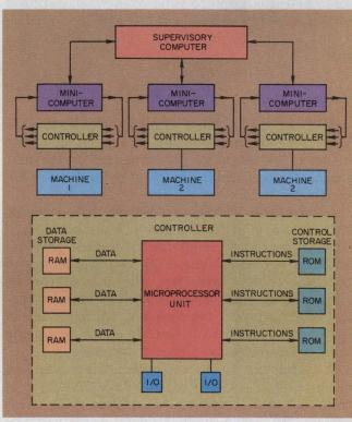
The hierarchy of computers in a fully automated system ranges from a large central unit to local smaller units and microprocessors within controllers.
