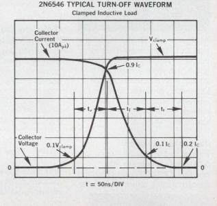
$I_{\text{CEV}}$  are at 100° case. You know  $t_s$  and  $t_F$  performance as a function of collector current and temperature at high inductive energy. You know precisely where you stand with secondary breakdown . . . before it happens. The unknown is known.
