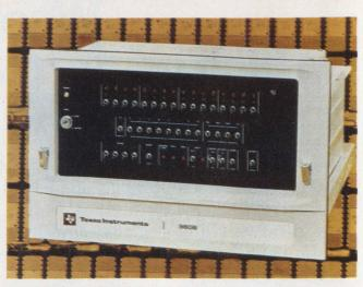
**Incorporating MOS memory elements** with single-bit error correction and multibit error detection, TI's 980B minicomputer allows single-bit manipulation.
