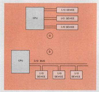
1. I/O bus structures employ several schemes. A radial system is the simplest, but it limits the number of I/O units (a). A party-line system reduces the number of lines needed for a distributed system (b). The latter system also comes in a daisy-chain version, which connects devices serially.
