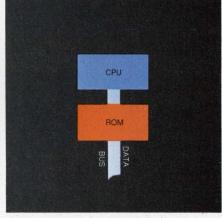
Minimal microprocessor system after the Fairchild F8.
