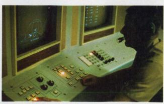
A dogfight flight training system for the Navy pits pilot against pilot in mock air-to-air combat. The computerbased system, by Cubic Corp., provides mission replay.
