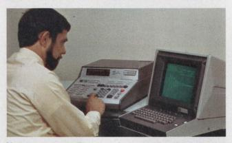
Model 31 (right). The use of graphical peripherals plus programming ease help make calculator systems popular design tools. Graphics tablets can also be used with some of these units.
