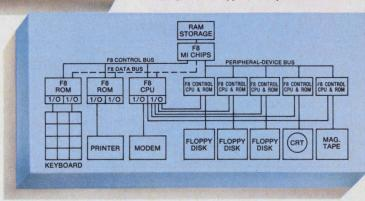
Key-to-floppy-disk. Multiple F8 processors are used in this key-to-floppy-disk system. Each controller consists of a CPU and a ROM. The processors are linked through a multiplexed memory channel provided by a DMA chip. This system illustrates the modular approach to expansion achievable with the F8. Because all controllers can operate simultaneously, total system throughput is increased.
