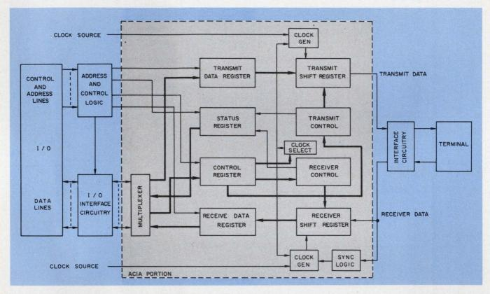
2. A peripheral controller consists of the blocks shown. An ACIA incorporates much of the circuitry needed.
