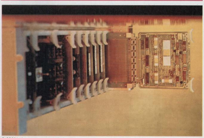
A 16-bit microprocessor on a single chip replaces the 15 to 20 ICs of older multichip versions. National Semi-
