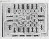
The 5 bit converter constructed on single printed circuit card. Total thruput time 50 n sec, with 20 MHz update rate. Temperature stability over full mil range,  $-55^{\circ}$ C to  $+125^{\circ}$ C with drift less than  $\pm 1$  bit over entire range. M.S. Kennedy Corp; Pickard Dr, Syracuse, NY 13211 (315) 455-7077.
