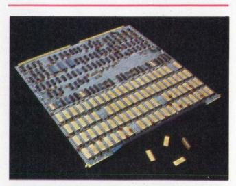
A semiconductor memory module from Data General has correction circuitry that can run without an error, even though four chips have been removed.
