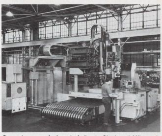
**Computer numerical control** directs Cincinnati Milacron's CIM-Xchanger Series 25HC machine, which carries 90 tools that can be randomly accessed by the program.
