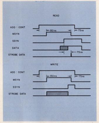
4. The mini establishes these timing requirements for read and write operations.
