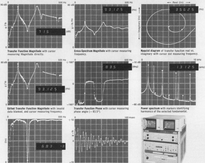
Coherence Function with cursor measuring degree of coherence (6.83 x 10-3).
