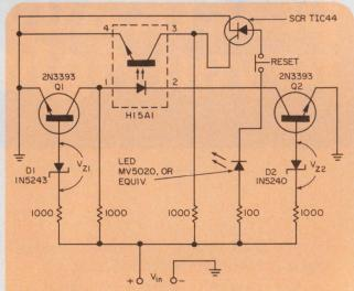
No separate power supply is needed for this voltage-monitor circuit, which has a LED indicator. The monitored voltage must not drop to zero or the event indication will be lost.
