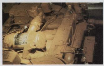
**Microprocessors monitor marine-engine performance** for maintenance and failure prevention. This diesel generator is watched by an Advanced Electronics Development Corp. system using gas, water and oil sensors.
