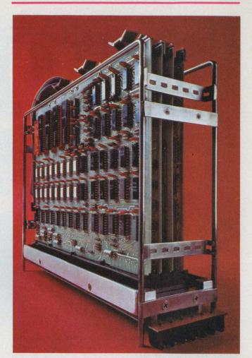
An 8-1/2  $\times$  10-in. board contains the major elements of a mini. The Digital Equipment Corp. LSI-11 board uses a multichip, n-channel microprocessor.
