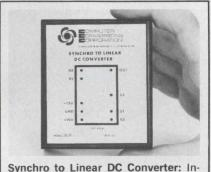
Synchro to Linear DC Converter: Infinite Resolution. Full (±180°) or Limited Angle DC Output (±90°), ±6 or ±15 minute accuracy at input rates up to 1440°/sec., 60 or 400 Hz input. Custom Output scaling available, Module 2.6" x 3.1" x .82" H. Price from \$350 in quantity. Computer Conversions Corp., East Northport, N.Y. 11731—(516) 261-3300. INFORMATION RETRIEVAL NUMBER 611
