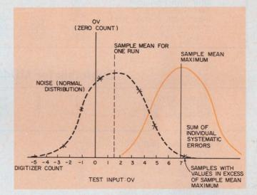
2. Performance capability is bounded by two main factors: cumulative systematic errors and random electrical noise. The computer calculates the mean and standard deviation to compare with calculated values.
