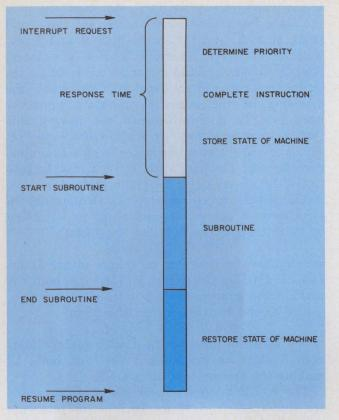
3. An ideal interrupt-service routine automatically saves the state of the microcomputer and then restores it after the interrupt has been handled.
