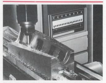
Three-dimensional contour cutting with hyperbolic interpolation is directed by General Automation's Adapt-A-Path and its SPC-16 minicomputer.
