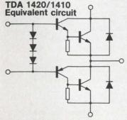
The TDA 1420 integrates a quasi-complementary (NPN/PNP) pair and biasing diodes for perfect electrothermal matching. Applicat this versatile power IC include DC stepping motor drivers, op amp p boosters, audio output stages, etc
