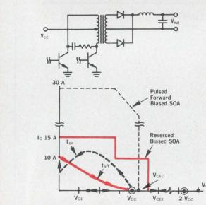
". . . both blocking voltage and sustaining voltage are important in switch-mode applications. The circuit illustrated requires high blocking capability since the transistor is subjected to a substantially higher voltage than  $V_{\rm CC}$  after turn-off . . ."
