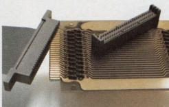
trimming the cable after assembly. Connector units provide positive alignment with precisely spaced conductors in 3M's flat, flexible PVC cable. The connector contacts strip through the insulation, capture the conductor, and provide a gas-tight pressure connection. With cable, connectors and assembly tools from one design and manufacturing source, you have added assurance the connection will be made surely, with no shorts or "opens."
