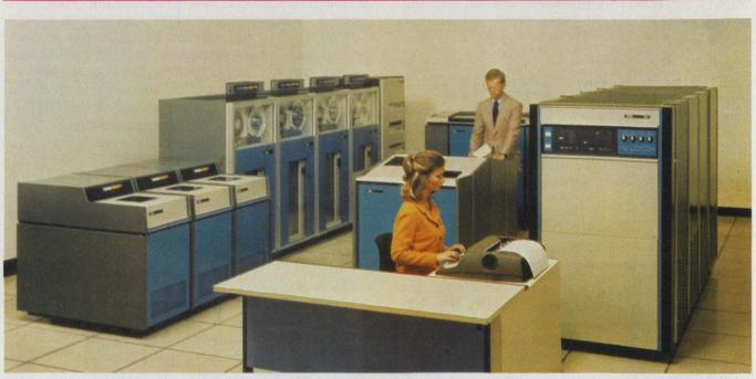
A single system processor controls input/output and arithmetic processors in the hierarchical architecture of the Xerox 560 computer, a 32-bit midi. Independent
