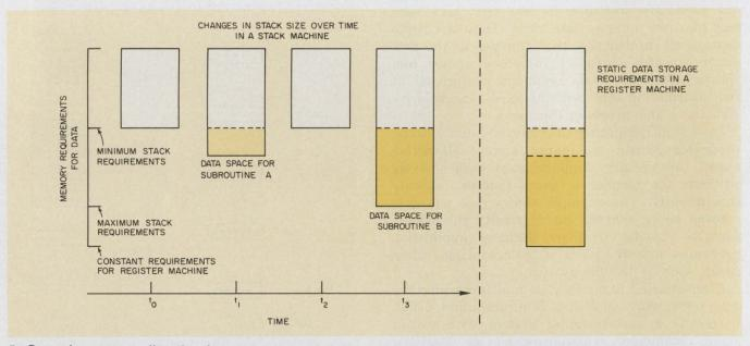
5. Dynamic memory allocation becomes automatic with a stack, since each subroutine uses only the amount of data space needed to perform calculations. In a regis-
