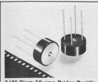
**3/4" Diam 10 amp Bridge Rectifiers** from Tarzian with heat dissipating aluminum base. 240 amp surge rating. Heat dissipation is 25W@10A. Max case temp is 150° C. H-FB Series supplied as standard avalanche, fast recovery or with special terminals. Sarkes Tarzian, Inc., Semiconductor Div., 415 College Ave., Bloomington, Ind. 47401, 812-332-1435.
