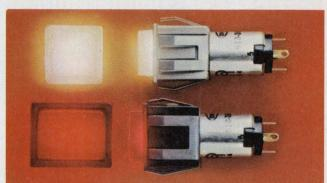
**513 SERIES** With bezel for snap-in panel mounting. Alternate, momentary and snap-action contacts with ratings to 5 amps. N.O., N.C. and two circuit (one N.O., one N.C.). Low level switches also available. Round, square and rectangular bezels in four colors; caps from  $\frac{1}{2''}$  to  $\frac{1}{2''}$  in more than 12 colors. Illuminated caps with or without legends. **UL listed**.
