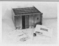
MP12 Small Computer System. Configure your own application system with 4k MP12 CPU with programmed I/O, interrupts, DMA. Interface cards for teletype, modems, floppy disk, paper tape, A/D, printer, card reader, mag. tape. Real-time operating system, full supporting software. Fabri-Tek, Inc. 5901 S. Cnty. Rd. 18, Mpls, MN 55436 (612) 935-8811 INFORMATION RETRIEVAL NUMBER 623
