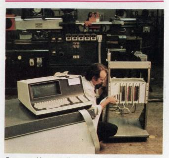
**Programmable controllers,** such as this Eagle-Signal CP600 with solid-state circuitry, are replacing the conventional relay-sequencing controller.
