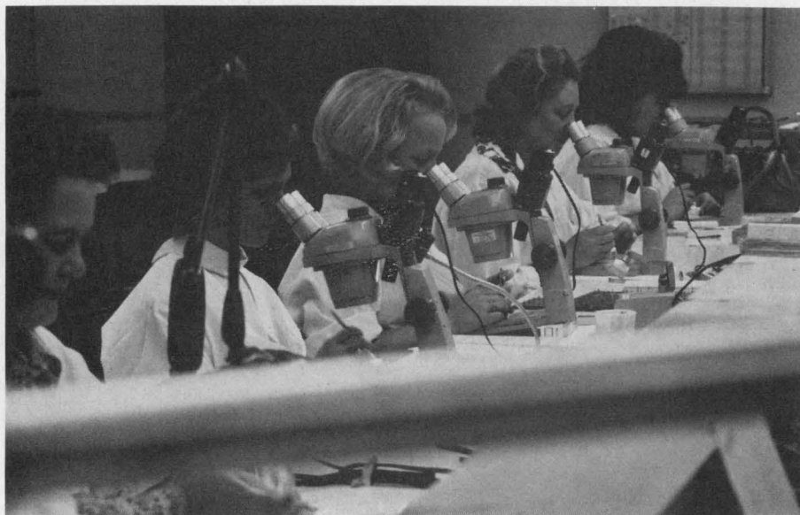
Iron-core microtransformers require detailed hand assembly and fabrication. Joining of heavy leads to wires between 0.001 and 0.0005-in. thick is a critical opera-
