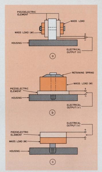
3. The piezoelectric accelerometer can be mounted to produce an output in either the shear (a), compression (b) or bender (c) mode of operation. In any of these operating modes, the accelerometer usually moves less than a thousandth of an inch.
