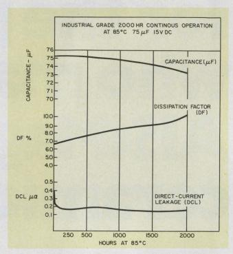
1. Even good grade aluminum electrolytic capacitors lose capacitance and experience an increase in dissipation factor with age.
