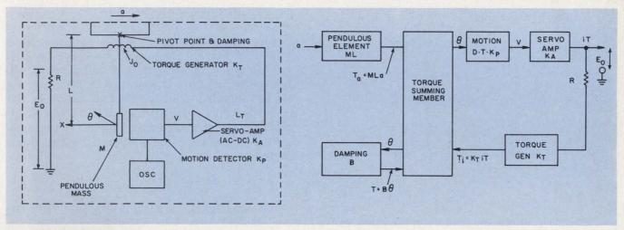
9. Servo accelerometers are closed-loop systems. They use a feedback loop to detect any forces.
