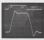
NON-COMPENSATED 10V/V GAIN STABLE INVERTING ONLY
