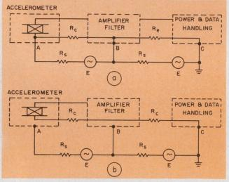
12. Ground-loop problems within a multicircuit measuring system can create many problems (a). If all the circuits use a common ground (b) the various pieces of equipment can work together.
