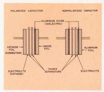
5. If there is any possibility that the circuit's polarity can reverse, only nonpolarized capacitors should be used.
