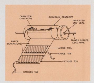
4. In axial-lead aluminum electrolytics, the container shell is usually connected to the cathode via a tab at one end. The anode lead passes through an insulating seal at the other end of the container.
