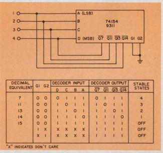
3. This quad-flop is built with a 1-of-16 decoder, as shown by the input-output table. A fifth state (1111) could be extracted with an external decoder, if needed.
