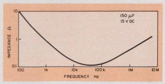
7. An electrolytic capacitor's impedance is equivalent to a series RLC circuit. Minimum impedance, which occurs at resonance, is resistive.
