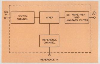
1. Basically the lock-in amplifier detects weak signals by the process of synchronous demodulation. Extraneous signals, which are not synchronized to the reference, are rejected.
