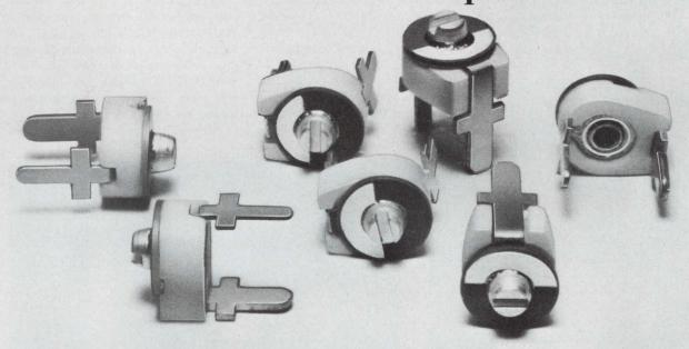
TDK's new dielectric material and improved configuration permits linear temperature characteristic with small-size ceramic trimmer capacitors (5mm in diameter).
