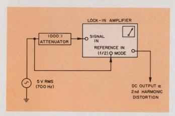
4. To measure the second-harmonic distortion generated in an amplifier (in this case, the lock-in itself), this test setup is used.
