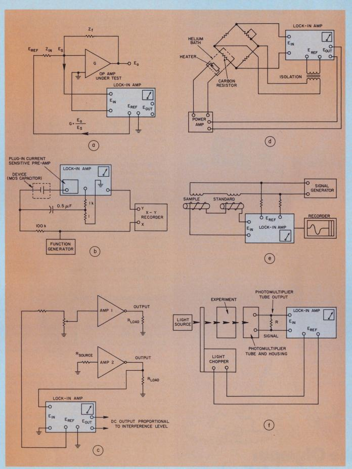
6. In typical applications, the lock-in is used to measure the open-loop gain of an op amp (a); to determine the C-V (capacitance-voltage) characteristics of an MOS semiconductor (b); and to measure amplifier crosstalk
