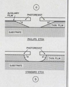
film, the fabricator can control slope of the thin film between 1 and 60 degrees. The Philips process has been fully developed for thin films of gold (to 5  $\mu$ m thick), for Permalloy (to 3  $\mu$ m thick) and silicon dioxide (to 10  $\mu$ m thick).
