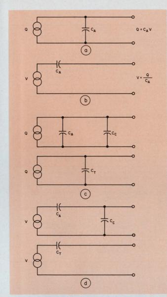
2. The piezoelectric accelerometer can be represented by a charge generator and a shunt capacitance (a) or by a voltage generator and a series capacitance (b). The effect of the cable capacitance can be added into the accelerometer models (c and d).
