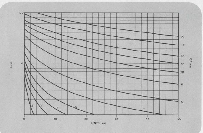
The specific inductance of a small coil can be obtained if you know its length and average diameter.
