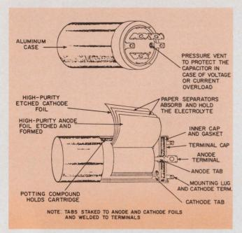
6. Large electrolytic capacitors have a vent to allow escape of any internal build-up of gas or vapor.
