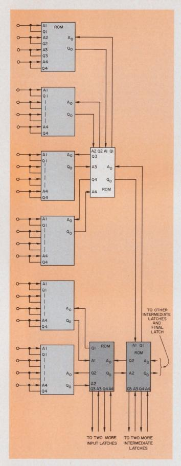
7. ROMs or programmable logic arrays (PLAs) can be the building blocks for large n-flops. Each ROM is a quad-flop. The circuit structure is a tree, and the over-all circuit has a lower package count than one built with decoders.
