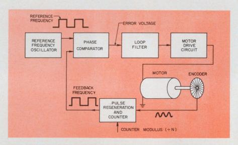
**Digital phase-locked loops** can be used for precision speed control as well as positioning. In this system, from Motorola, a shaft encoder is used to sense motor speed, and a pulse train is fed back to a comparator, to be checked against the reference pulse train. If the motor is not synced to the reference, an error voltage adjusts the motor speed.
