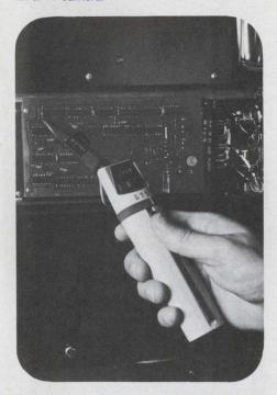
A new RF probe adds 100 kHz to 500 MHz ac measurement range to HP's handheld 970A digital multimeter. Accuracy within this range is greater than 1 dB. The new 97003A RF adapter measures 0.25 to 30 V full scale. Maximum input is 30 V rms, plus 200 Vdc.
