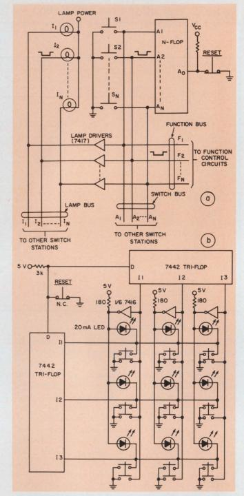
8. These n-flops latch for the most recent button pushed. The first circuit (a) uses single-contact switches. The m  $\times$  m arrangement (b) uses smaller n-flops.
