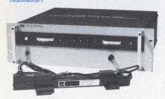
When your application calls for a system or lab power supply in the range of 0-4 kV, HP has six models to fill your need. Three of them are constant voltage/constant current supplies with sufficient output current to power devices such as klystrons, magnetrons, backward-wave oscillators, high-power gas lasers, and electron-beam welding devices. Model 6521A delivers 0-1 1kV at 0-200 mA; model 6522A delivers 0-2 kV at 0-100
