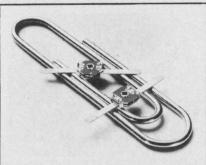
Thin-Trim variable capacitors vide a reliable means of adjusting capacitance without abrasive trimming or interchange of fixed capacitors. Series 9401 has high Q's and a range of capacitance values from 0.2-0.6 pf to 3.0-12.0 pf and 250 WVDC working voltage. Johanson Manufacturing Corporation, Boonton, New Jersey (201) 334-2676.
