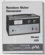
The Model 420 provides a precisely calibrated random noise source with Gaussian amplitude distribution. Spectral density distribution is independent of frequency (white) with lower cut-off approaching D. C. Analog outputs from 0.01 to 1000 µV per root Hertz continuously variable and metered. Response is flat from D.C. to 100 KHz.
