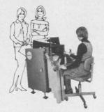
to do the rest: position housing . . . insert terminal to exact depth and lock it in place . . . repeat until the preset number of terminals are inserted . . . then eject the completed connector—all automatically.
