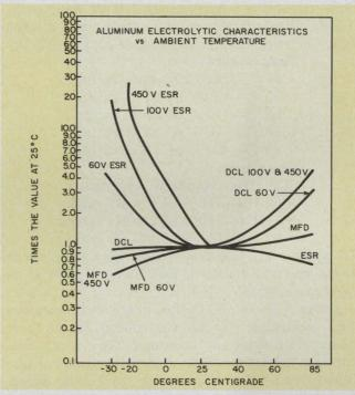
3. The important properties of an electrolytic depend strongly on the unit's temperature. DCL rises steeply but ESR drops with increasing temperature.
