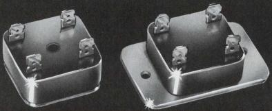
It's the year of the compact and our 25 amp ELF Bridge packs all the power of more bulky encapsulated assemblies. Our double diffused diode is available with ratings up to 1200 PRV. Designed to be an economical bridge, it meets NEMA creepage clearances and Hi-pot standards. Suitable for extreme temperature conditions to -55°C, it is available in single hole (Series EMF) or flange mounting (Series ELF).
