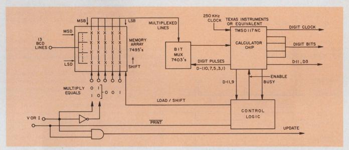
Power is derived by direct multiplication in the calculator chip of the BCD numbers for voltage and cur-
