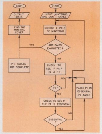
1. Flow chart of CAD program shows how logic functions are simplified. Minterm pairs are checked to find prime implicants in the final minimized function. A minimal cover process selects the fewest prime implicants to contain all minterms in the function. Essential prime implicants are always included.
