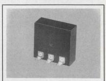
Solid-state timers—TS Series Delay On Make, N.O. or N.C. Operating voltages: 12, 24 - 230 v. Operating temps from -40°C to +60°C. Adjustable delay ranges or factory fixed. Encapsulated circuitry. Transient protected. DC units reverse polarity protected. SSAC PRECISION PROD-UCTS, INC., Box 395, L N.Y. 13088 (315) 457-9610 Liverpool,
