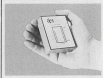
"Synchro to digital converters - 10, 12, or 14 bit output, errorless tracking up to 4 r.p.s., accuracy ±4 min. of arc ±.9LSB, resolution - 1.3 minutes, 60 or 400 Hz input, Module 2.6 x 3.1 x .82" H, Price From \$350 in aty.
