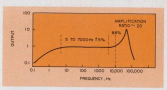
5. Typical output response of a piezoelectric accelerometer is very poor near dc, at input frequencies it is flat and at resonance it increases sharply.
