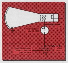
Even though the Corotron operates in the corona mode of discharge, it has no voltage jumps or jitters. Corotrons are not tied to "natural" operating voltages and are adjustable in manufacture from 350 to 30,000 volts.
