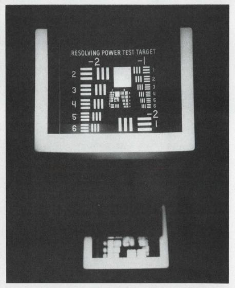
The image of a resolution chart projected by a heads-up display demonstrator and viewed at infinity shows the resolving capability of the unit. The blurred image below is the original resolution chart viewed without the hologram lens.
