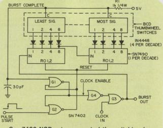
One 7402 NOR gate can control the switching for a large number of thumbwheel-programmed pulses.
