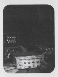
The new 3312A function generator has sine, square, triangle, positive and negative ramps. Accuracy is  $\pm 5\%$  of full scale.
