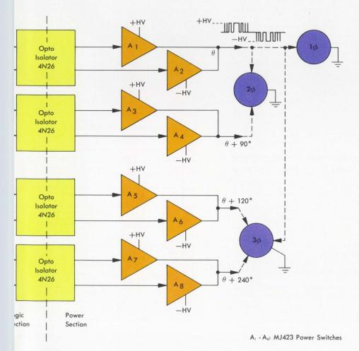
FIGURE (3) — Controller output signal synthesis idealized load current waveforms  $B_0 + B_0 +$
