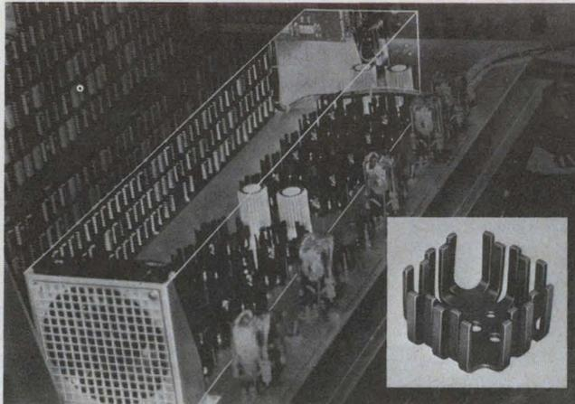
**X-Y plotter designer** put all his hot TO-3 power transistors in one basket to cope with heat problem. Utilizing existing chassis, he mounted devices in UP dissipators, wrapped a shroud around the assembly, and installed a blower. The UP's staggered fingers create turbulence in air stream for maximum efficiency of both the dissipator and air flow, and allowed the designer to meet his design goal of 80°C case rise maximum. He also had room within the shroud to cool his hot resistors.
