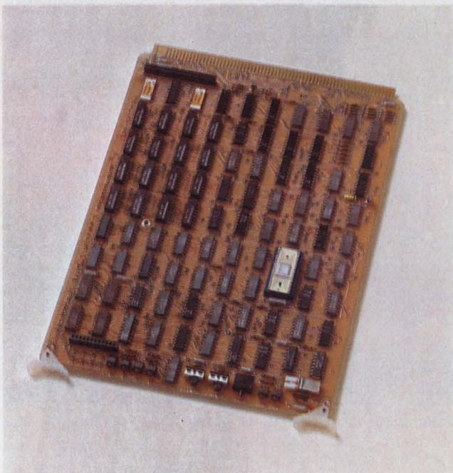
Custom silicon-on-sapphire LSI processors are the basis for General Automation's LSI 12/16, an 8-bit system. The mini maker also uses SOS chips for a 16-bit system, the LSI 16, that is a functional equivalent of the company's SPC-16 mini.
