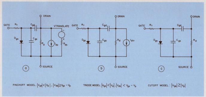
2. Depending on relative values for  $V_{\rm gs}$  and  $V_{\rm ds}$ , the circuit models for the pinchoff (a), triode (b) and cutoff (c) regions of FET operation can be applied. The models are valid for all values of drain current and
