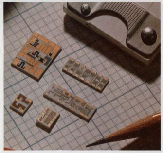
Resistor networks, such as these TRW TanFilm units, are filling industry needs for package-compatible components for hybrid and DIP configured circuits.
