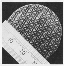
This slice of green-doped galliumphosphide material has been processed to produce seven-segment numerics, each 2.5 mm high.
