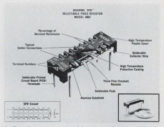
8. For those set-once-and-forget applications, Bourn's SFR selectable, fixed resistors provide a definition of 1% and a resistance range of 33  $\Omega$  to 1.25  $\text{M}\Omega$  with only 15 units.
