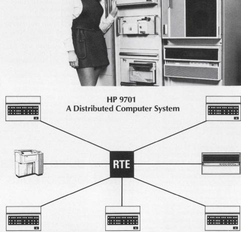
The 9700 distributed system concept involves satellite computers that interface with a central multiprogramming real-time information system. Remote computers can be added in modular fashion.
