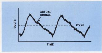
1. A "typical" noise signal consists of a periodic ripple and noise spikes—both superimposed on a dc level. This noise can cause 100% errors.
