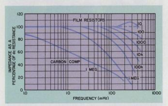
4. The impedance of composition and film resistors generally drops at higher frequencies because of capacitive shunting. Note that only the Mepco  $10 \cdot \Omega$  film resistor shows an inductive effect above 150 MHz. Wound resistors, of course, show the greatest inductive effects and film resistors the lowest capacitive effects.
