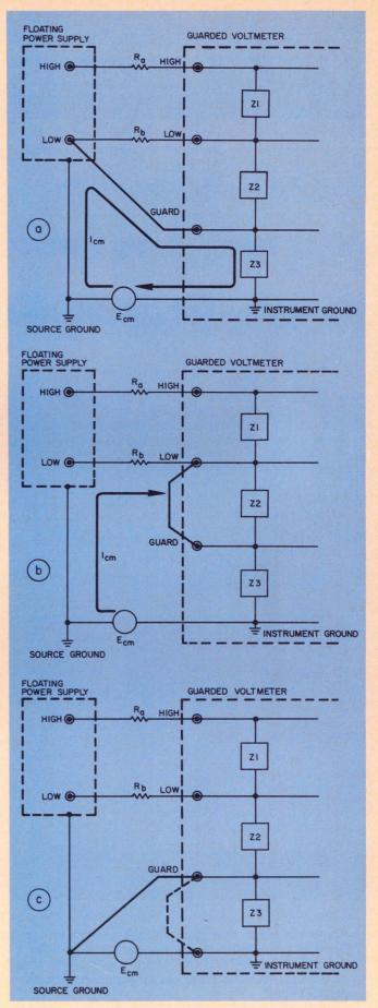
7. A source and guard can be connected in three ways. in the preferred connection (a), no common-mode current flows through  $R_{\rm a}$  or  $R_{\rm b}$ . In the other two connections (b, c), some current may flow in  $R_{\rm b}$ .
