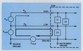
4. Two sources of noise— $E_{\rm em1}$  and  $E_{\rm em2}$ —can appear in a floating measurement, in which neither source terminal is grounded.
