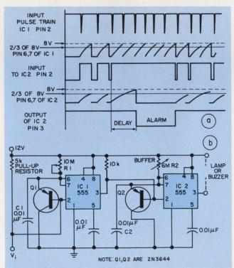
2. A speed warning device senses the car speed by comparing the frequency of pulses generated by the rotating wheel. The generated pulse train (a) is processed by the two timer circuit (b) and activates an alarm signal if the speed is too high.
