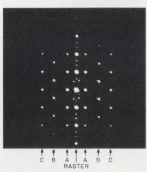
3. **Synthetic gratings formed** by modulating laser with three carriers have a unique white-light pattern.
