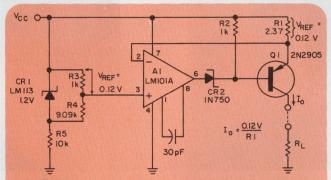
2. Extended compliance circuit uses a resistive divider to lower the apparent zener voltage, thereby permitting the load voltage to go within a few millivolts of  $V_{\rm cc}$ .
