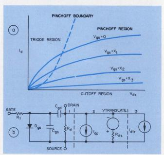
1. The three regions of FET operation, shown in a multicurve plot of  $I_{\rm d}$  vs  $V_{\rm ds}$  (a), can be modeled with the circuit of b. The portions of the circuit labeled 1, 2, and 3 are used as the circuit model for, respectively, for cutoff, pinchoff and triode-region operation.
