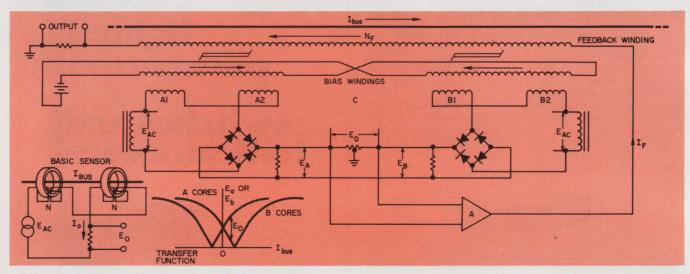
Here's a tough problem: Measure a bipolar dc current of up to 10,000 A without breaking or touching the line and without loading. And do this to within a linearity of 0.015% and with a circuit that's not affected by temperature changes, line-voltage variations, magnetic fields or aging.
