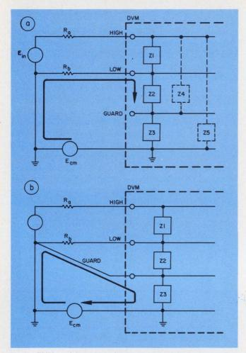
5. In DVMs with a guard, the impedance between low and ground is increased by  $Z_{\rm 3}$  (a). Connecting the guard to the source low terminal shunts unwanted currents (b).
