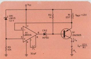
1. High-compliance current source uses a low-voltage zener to minimize the voltage drop across R<sub>1</sub>.
