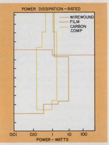
6. Some ranges of tolerance, temperature coefficient and power are dominated by a particular type of resistor, while other ranges can be handled by many different
