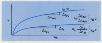
3. Conductance in the pinchoff region is normalized to the  $V_{\rm gs}=0$  curve slope,  $G_{\rm o}.$  This conductance can be interpolated from manufacturers' curves.
