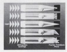
2. Diffraction patterns of gratings can be optically processed to recover impressed information.
