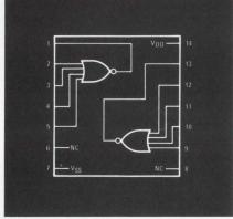
Pin for pin compatible with CD-4002A. 100-999 units -40°C to +85°C \$1.00 \$3.40
