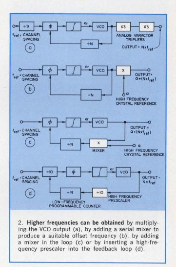
mix down (Fig. 2c). The only difference here is that the VCO now runs at the output frequency. For instance, the VCO could cover the 148-to-172-MHz range, while the 140-MHz offset would reduce the divide-by-N frequency to 8 to 32 MHz. We have exactly the same advantages and disadvantages as when mixing up. However, the VCO design is usually simpler, because the circuit uses smaller components and it operates over a narrower bandwidth.
