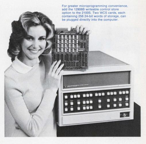
Now, HP offers a minicomputer with built-in "extras" including microprogramming. Extended arithmetic instructions, floating point hardware, dual-channel direct memory access, power fail interrupt, memory parity check, and memory protect—they're all built into the new 2100S computer. A programmable time base generator, communications control channel, and 16K words of 16-bit memory are also standard.
