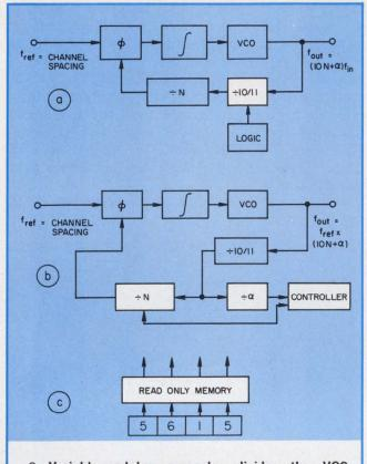
3. Variable-modulus prescaler divides the VCO output either by 11 or 10 (a), as determined by the associated controller IC (b). A ROM look-up table permits the use of simple BCD thumbwheel switches to convert operator-meaningful data into the numbers required by the divide-by-N operation.
