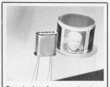
Ceramic low frequency bandpass filters, available from 6 kHZ to 55 kHZ for military and commercial applications. Sealed in HC-6/U crystal cans. Typical parameters are 0.9% minimum 3 dB BDW., 20 dB/3 dB skirt ratio < 13, insertion loss < 5 dB, 30 dB stopband to 100 kHZ. Andex Corporation, Middleburg Hts., Ohio, (216) 842-5339 INFORMATION RETRIEVAL NUMBER 188
