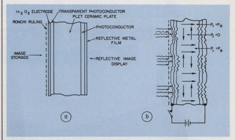
Fericon structure (a) stores images as strain-induced deformations (b) on the surfaces of lead lanthanum zirconate titanate (PLZT) plates.
