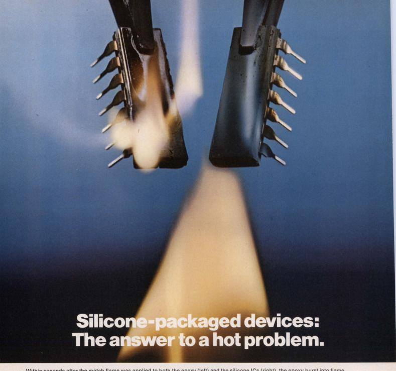
Within seconds after the match flame was applied to both the epoxy (left) and the silicone ICs (right), the epoxy burst into flame.
