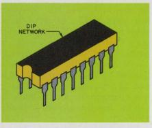
2. For compatibility with popular DIP circuits, passive components are also packaged in DIP form, as in Corning's Cordip line. Custom network designs, and an
