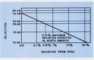
2. Integrating DVM with 1/60-s period of integration exhibits 56-dB of rejection for commonly-encountered line-frequency fluctuations of  $\pm 0.15\%$ .
