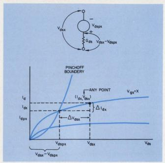
5. The origin of any  $V_{\rm gs}$  curve is set at the pinchoff boundary to maintain the needed continuity along the boundary. Voltage source  $V_{\rm dspx}$  is used to account for the difference between this origin and the actual one.
