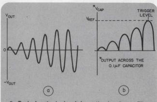
2. Typical output signal from the bandpass filter (a) contains only the desired ultrasonic frequencies. Peak-detector output voltage (b) builds until it reaches  $V_{\rm REF}$ , the trigger level of the comparator.
