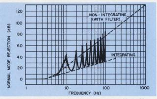
3. A comparison of an integrating and a filtered-input DVM shows that filtering is best for broadband noise, integration for line-related noise.
