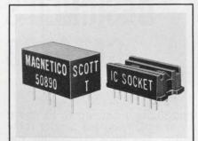
Scott T transformer—dual in line size. In a DIP type size and pin spacing, Scott T No: 50890 converts 400 Hz 11.8V RMS line to line synchro information to 6V RMS Sine and Cosine resolver outputs. Accuracy is 2 arc minutes. Cost is \$25.00 in qty. For any Scott T call: Magnetico, Inc., East Northport, N.Y. 11731. Tel: (516) 261-4502.
