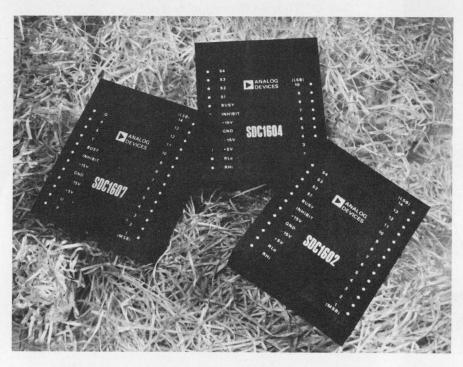
maximum. The outputs are TTL/DTL-compatible, with a fanout of four TTL loads. The seven-ounce 1602 measures 3-1/8 × 2-5/8 × 0.8-in.
