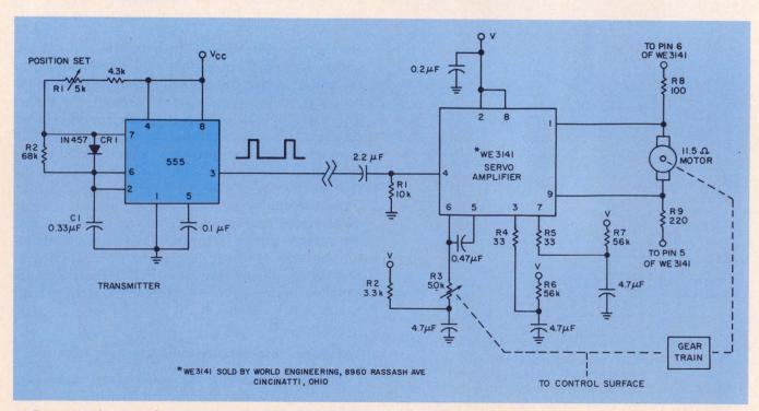
4. To remotely control a servo-motor, the 555 needs only six extra components.
