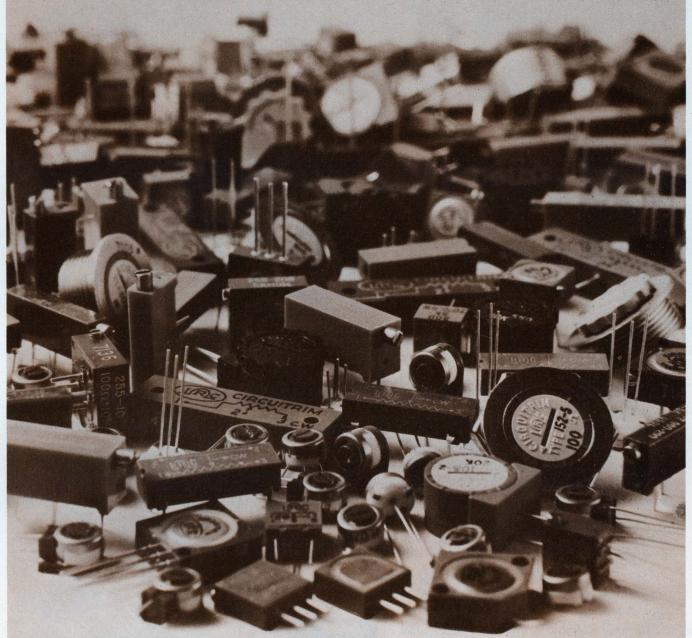
These infinite resolution pots cover the complete size range from ¼" round to 1¼" rectangular in the industry's widest selection of mounting configurations.
