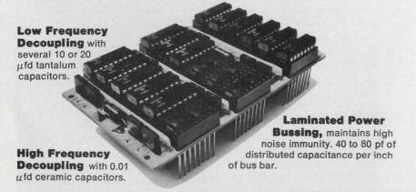
Free Test Data: Get this eye opener! Scope traces of comparable IC logic circuits show convincingly how EECO's power distribution system performs, how you save hours of debugging agony. EECO, 1441 E. Chestnut Ave., Santa Ana, California 92705. For fast answers up-front, call Electronic Packaging Products. (714) 547-5651.
