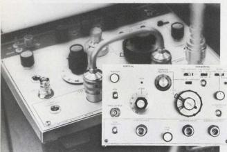
The 1818A time domain reflectometer is easy to use and extremely practical for field measurements
