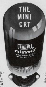
BOOM...big information in a small package. nimo®, a 1.5" MINI-CRT requiring no internal or external focusing or deflection.
