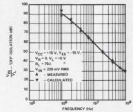
Switch OFF Isolation vs Frequency - DG181
