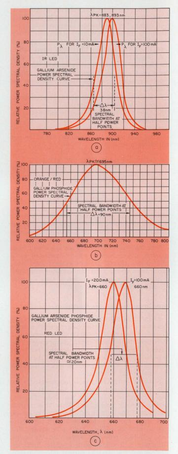
7. Relative power spectral density curves give LED emission as a function of wavelength. Infrared LEDs give peak emission at about 890 nm (a), orange/reds peak at 695 nm (b) and red LEDs peak at 660 nm (c).
