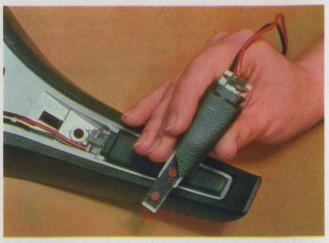
**Pressing a new conductive elastomer** in this steeringwheel button causes the horn to sound. The material, Pressex, has positive switching characteristics.
