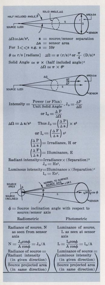
1. Relative geometry of point source and sensor (top and center) determine light intensity at the sensor. Area of extended source (bottom) affects intensity. propriate unit of luminance.
