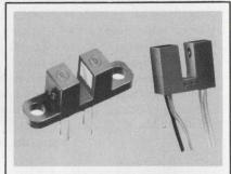
Hermetically sealed optical switch: Contains discrete matched hermetic LED/photo transistors. DTL/TTL compatible output. SSOS-700 straight package. SSOS-800 package with flange. Gap dimension between photo transistor & LED is .110". Solar Systems, Inc., 8124 Central Park, Skokie, III. 60076. Phone: (312) 676-2040.
