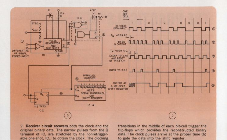
10-bit, serial-in, and parallel-out register is provided by the nonretriggerable one-shot,  $IC_3$ . The output pulse width from  $IC_3$  must be at least half-bit-cell wide, and it also is calculated with Eq. 1. The clocking transitions in the middle of each bit cell trigger the flip-flop at the end of each one-shot pulse. This insures that sufficient setup and hold time is provided for data input to the shift register for each clocking transition.
