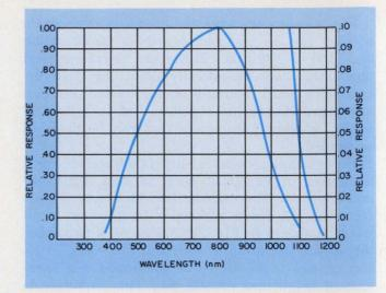
6. Silicon sensor (PIN 10D) calibration curve shows relative spectral response. Responsivity of cell at 800 nm (peak  $\lambda$ ) is 0.379 A/(W/cm<sup>2</sup>).
