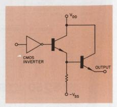
**Each of seven output stages** has an npn Darlington transistor network for higher drive currents.
