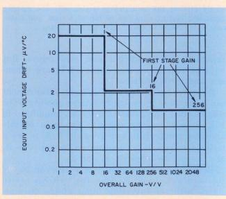
8. First-stage gain has a substantial effect on the amplifier's voltage drift.
