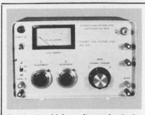
**Electronic high voltage load** for static and dynamic testing of high voltage sources to 30 kV at 2 mA. Switches two independently adjustable load levels from dc to 100 kHz. Provides for ripple, regulation, and recovery time in a single display. Advanced High Voltage Co., 14532 Arminta St., Van Nuys, CA 91402. (213) 997-7222.
