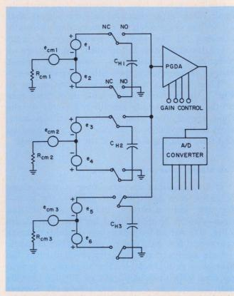
11. A flying-capacitor multiplexing system can maintain a high common-mode rejection ratio and handle large common-mode input voltages.
