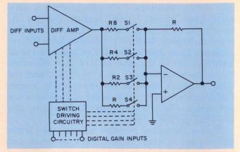
6. This two-stage programmable-gain system offers the combined advantages of differential input, high input impedance, and course and fine gain-controlled ranges.
