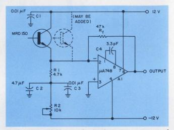
1. Op amp  $\mu$ A748 extends the frequency response of the phototransistor by maintaining the device's output at an effective ac ground. Feedback resistor R<sub>f</sub> adjusts gain, and potentiometer R<sub>2</sub> balances out the quiescent current of the phototransistor.
