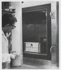
HP cesium beam standards undergo extensive environmental testing. Here, one is being tested at high altitude and high and low temperatures. HP's new digital magnetic tape drive can handle virtually any recording problem—200, 556 or 800 cpi NRZI; any speed from 25 to 45 ips; or 1600 cpi phase-encoded recording that is ANSI/IBM compatible. You get 7 and 9 track, multi-density, NRZI and PE capability—*all* in one read-only tape drive, model 7970E.
