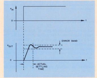
7. Settling time is particularly important when specifying a programmable-gain amplifier.
