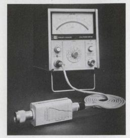
For microwave power measurement, this system has high accuracy with wide dynamic range and broad frequency coverage.
