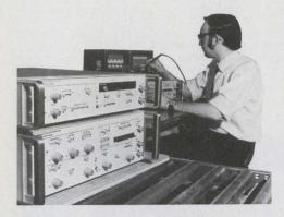
Besides testing PCM equipment, the 3760A/3761A tests computer memories, disc storage, digital recorders, and high-speed logic circuits.
