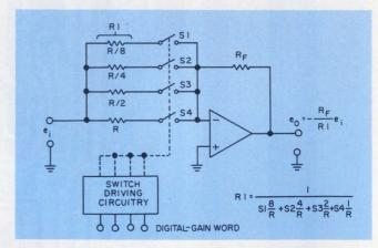
2. A programmable-gain amplifier is basically an op amp whose feedback network is switched to accurately control the closed-loop gain of the configuration.
