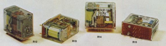
These new solid state time delays each designed to solve different design problems—are built around our compact, widely accepted R10 relay. Each is available in 2 or 4 Form C contact arrangements and may be mounted directly to a chassis, printed circuit board, special mounting strip or in sockets having solder or printed circuit terminals.
