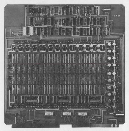
At left is a REAL 72,000-bit semiconductor memory built with Intel 1103's, the 1024-bit silicongate MOS RAM that's winning the price performance competition in main frame memories.
