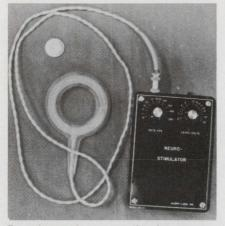
**Experimental neuro-stimulator** consists of a transmitter with a coiled loop antenna. The antenna is placed over an implanted receiver.
