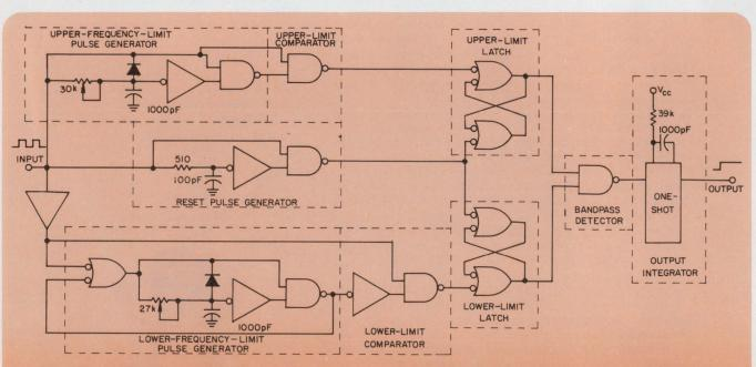
The output of this tone detector is a sharp, narrow, square pulse that is produced when the input frequency is within the preset passband. The upper and lower limits are individually tunable; thus both the center frequency and passband are adjustable. An integrator, in the form of a retriggerable oneshot, can be added for applications requiring a continuous true output.
