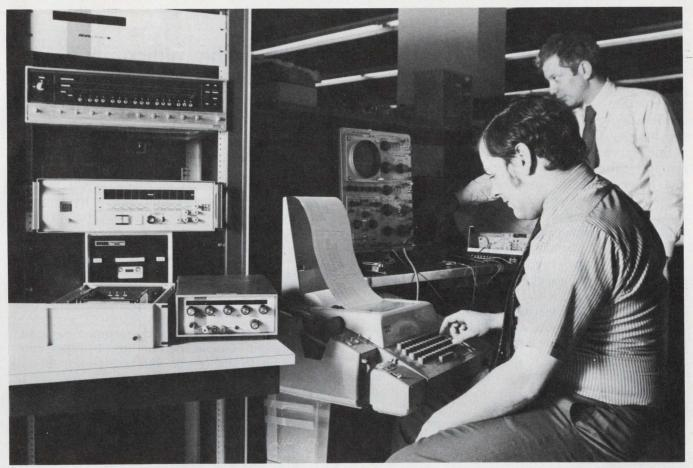
A computer-controlled system for testing analog-todigital converters at Analogic Corp., Wakefield, Mass., employs a Data General Nova computer and a Compu-Systems programmable voltage standard to automatical-
