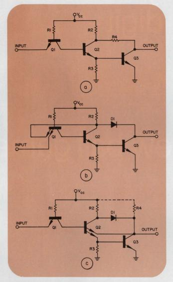
3. Clamping techniques enhance gate switching speed. Essentially the transistors are kept from saturating and the voltage excursions are reduced. A resistor clamp (a), a phase-splitter clamp (b) or an emitter clamp (c) can be used. The dashed lines in (c) show an alternate pull-up technique for the emitter clamp.
