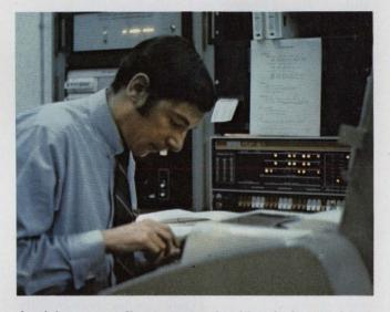
A minicomputer directs tests, classifies devices and logs data in the sophisticated J283 IC test system made by Teradyne of Boston. Here Norman Turner, software development engineer, works on a new job program which fixes pin and source assignments, source values and reject criteria.
