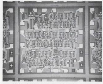
This CMOS eight-stage static shift register, selling for \$4.35, is one of RCA's new, low-cost series. Power dissipations for these MSI circuits are typically 10  $\mu$ W, while that for a gate package is 10 nW.
