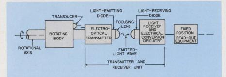
**Transducer picks up vibration data** from rotating object and feeds it into an electro-optical transmitter. The transmitter's modulated beam is received by diodes, converted back to the vibration rate and presented on a display.
