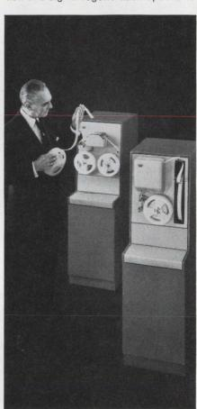
**Telespeed™ equipment:** A line of high-speed tape-to-tape terminals capable of sending and receiving at speeds of 750, 1050 (shown above), or 1200 words per minute.
