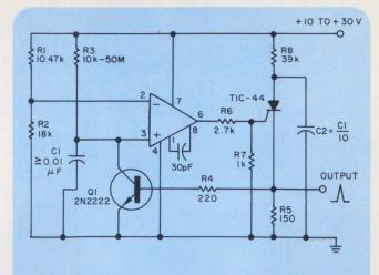
Vary the timing cycle of this pulse generator from 1 ms to 1000 s by simply tweaking some of the passive-component values. High accuracy and temperature stability are main features.
