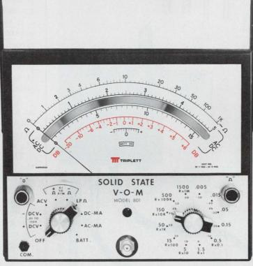
Lower power ohms — 8 ranges with 35 mV power source and 1 ohm center scale.
