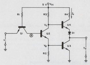
A popular TTL output gate employs an active pullup. A current spike,  $I_r$ , occurs when the gate switches from logic ZERO to logic ONE, because a stored charge in  $Q_2$  delays its true turn-off.
