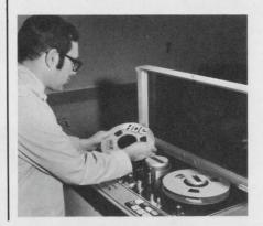
"High Energy" tape being New placed on video helical recorder is treated with a cobalt-modified ferric oxide formulation that creates a 4-dB increase in both rf output and signalto-noise ratio. The 3M Co. will use the new material on video tapes. sound cassettes, and instrumentation and computer tapes. Above are the oscilloscope readings of rf output of standard tape (left) compared with almost double the output (right) of the tape backed with the new oxide.
