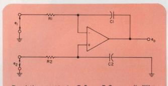
Equal time constants,  $\mathbf{R}_1\mathbf{C}_1 = \mathbf{R}_2\mathbf{C}_2$ , permit differential integration with a single amplifier. The circuit output is the true integral of the input difference voltage. Capacitor  $\mathbf{C}_2$  replaces an op amp.
