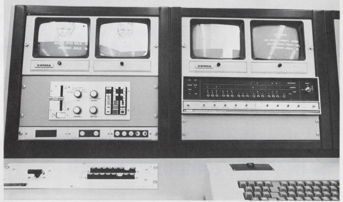
The heart of the Ampex PYRAMID educational system is the NOVA minicomputer. The system, a set of modular subsystems which function as peripherals, allows each student to start, stop, replay, hold, or discontinue his
