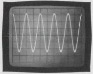
Conventional scope display of 5 MHz signal appears undistorted  $\longrightarrow$
