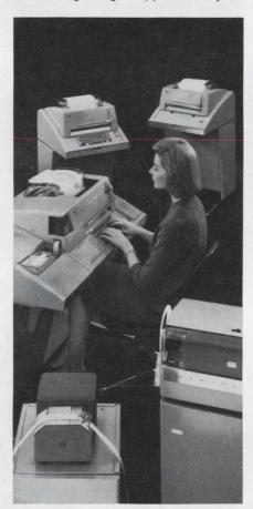
*model 35 series:* A rugged, heavy-duty line of 100 wpm terminals. Uses ASCII. Units in foreground are self-contained paper tape punch and paper tape reader.
