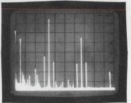
but spectrum analyzer identifies parasitic oscillations.
