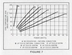
more than four times more power at the same case temperature. In a forced air environment of only 200 FPM, 28 watts can be dissipated — more than nine times the power at the same case temperature. With 1000 FPM, the remarkable light weight UP will allow 50 watts of dissipation from the transistor — seventeen times more power at the same case temperature.
