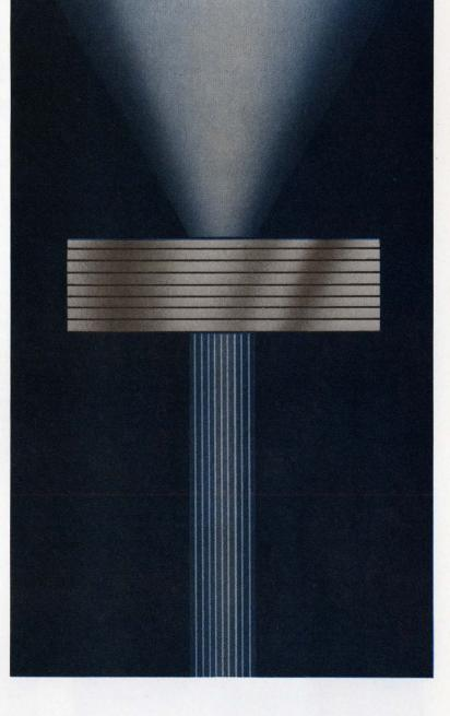
Until now, no one has been able to produce holes in thick metal at anything smaller than a one-to-one ratio. We put our world leading technology in photomechanical reproduction to work and came up with a way to laminate sheets of etched metal in perfect register. We can produce sharply cornered holes of any design in metal much thicker than the width of the hole.
