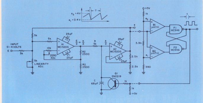
Ramp generator (left) can be converted to a sawtooth VCO by addition of comparators and a flip-
