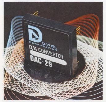
Modular eight-bit digital-to-analog converter gives an overall full-scale accuracy of  $\pm 0.2\%$  for only \$29. Its output settling time is 20  $\mu$ s to  $\pm 0.2\%$ .
