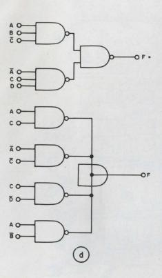
Mr. Pappa's point on serviceability is well taken. The wired-OR does present a problem when the output, F, is at a permanent ground. Granted that all DTL outputs must be removed to find the defective gate, we really are only interested in determining which IC package is bad.
