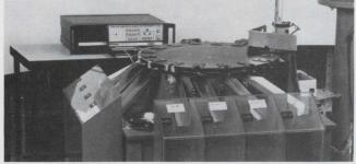
thorough testing. Lots are first sampletested dynamically. Once a lot passes these tests, DEC puts every IC in that lot through a full battery of functional and dc parametric tests. And it manages these dc and functional tests with an instrument that isn't much bigger than a breadbox and that costs less than a Cadillac. The instrument is a Teradyne J133.
