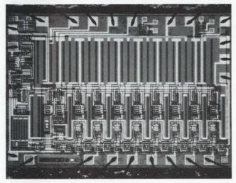
Do we mean "guaranteed?" You bet we do. The RI-1080 has its own thin-film resistor ladder network built right on the same IC chip as the bipolar switches. Without that, any guarantee would be meaningless. With it, the RI-1080 is the only D/A converter that has a guaranteed 8-bit performance over the entire military range from  $-55^{\circ}$  to  $+125^{\circ}$  C.
