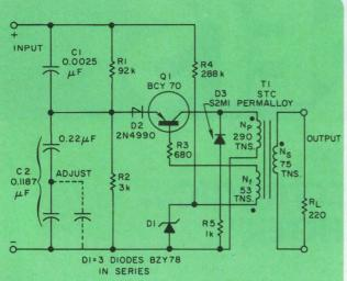
A pulse train appears at the output as long as the input voltage remains above a preset value. Series zeners  $(D_1)$  provide a stable dc reference voltage.
