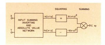
1. An analog multiplier can be based on a squaring circuit. One type of squaring circuit makes use of a parabolic or square-law function derived from harmonically related triangular waves.
