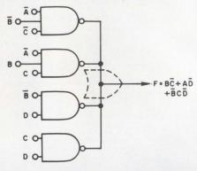
(Incidentally, this circuit is the correct wired-OR implementation for F, as shown on p. 90 of the article.)
