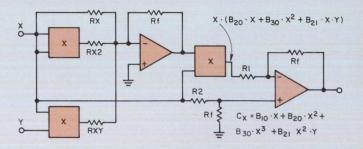
3. After the equation for the proper deflection is obtained, the circuit can be designed. This is the block diagram of a network for the X deflection for the equation shown.
