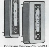
Compare the new Clare HGJ Relays with any other mercury-wetted contact relays. You'll get more speed, less noise, and less jitter—in less space than any other! Take your choice: 0.340" profile for true halfinch pcb spacing, 0.400" profile for higher sensitivity. Single-pole HGJM, two-pole HGJ2MT. Both are capable of switching low level to 2 amp max, 500 v max (100 va max, ac or dc).
