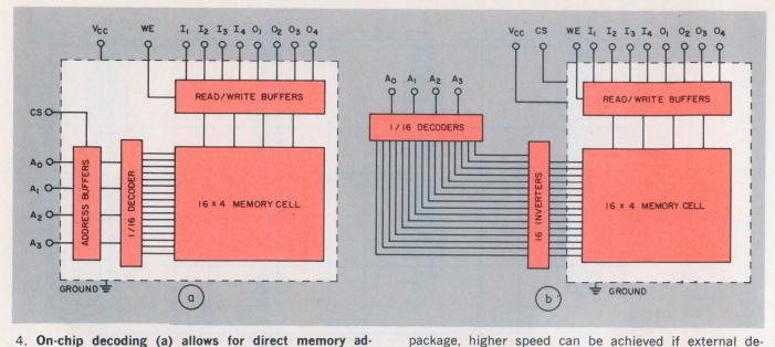
4. On-chip decoding (a) allows for direct memory address in binary form. Although this results in a smaller
