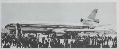
Santa Monica, Calif. With advanced guidance for automatic landings in zero-visibility weather, an on-board computer and a color CRT cockpit display among its electronic highlights, the first McDonnell Douglas DC-10 is undergoing taxiing tests prior to making it maiden flight.
