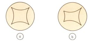
1. A square trace is distorted by a single gun CRT into the pincushion of "a." An off-axis gun, as found in a multigun tube, causes additional keystone distortion (b).
