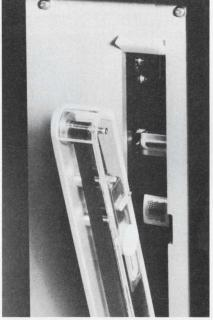
A new data storage system called Comfile provides the data access and organization styles of discs and drums at the low costs associated with magnetic-tape cartridge systems. At the heart of the new system is a 30-inch-long magnetictape loop capable of storing up to 72,000 characters of data. This stored data is accessible within an average time of 315 ms.
