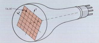
2. The first step in compensating for distortion is to divide the CRT face into a grid. The X and Y deflection voltages for each point determine the correcting network.
