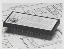
**Standard MOS/LSI devices,** such as this data communicator developed by Larse Corp., may eventually replace pneumatic equipment now used for control functions in factories. and weather-data collection.
