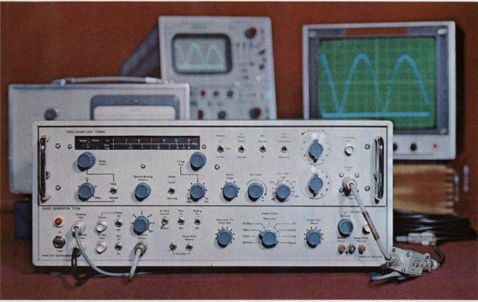
With a detected system flatness within  $\pm 0.05 \, dB$  over the full video range, and a battery of features to aid precise measurement, the new TF 2361 provides a standard of accuracy not usually associated with general purpose sweep generators.
