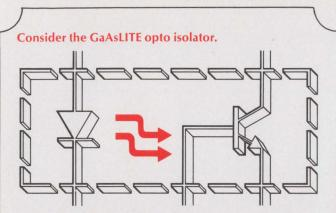
Couple a GaAsLITE to a silicon detector, and you get almost perfect isolation between input and output; 100,000, 000,000 ohms. Our opto isolators listed here do just that, and more. They give high performance at great speeds for very low cost. Scan the details. Each is packaged for mass production handling, and each is priced to suit quantity applications.
