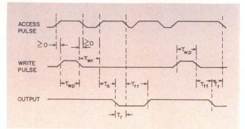
5. The cycle times for all possible memory operations can be determined from the switching characteristics. For example, the WRITE to READ cycle time is the sum of WRITE pulse width  $(T_{wp})$  and the recovery time  $(T_{wr})$ .
