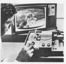
Conventional Super-8 movies can now be transmitted to any number of black-and-white television screens by a new system that resembles an ordinary tape recorder. The equipment consists of a projector and a small video camera which picks up the image for transmission to the TV screen. Either spools or cassettes of film can be used, and sound can be recorded on pre-striped film through the equipment. The manufacturer is Vidicord Holdings Ltd., Condon, England.
