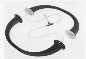
3. Military version of aircraft navigation antenna by Granger Associates withstands supersonic speeds. It is installed during plane construction.
