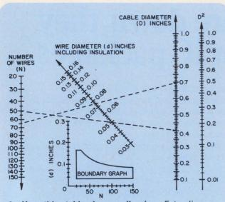
1. Use this table for small wire. Extending a straight line between known wire diameter d and quantity N determines the minimum cable diameter upon intersection with D.
