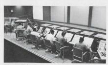
Three 7-by-7-foot translucent screens present in six colors the positions and tracks of ships, aircraft and drones on the sea ranges to the north and south of Puerto Rico. The information is fed both through a computer and manually by operators at consoles. Projection is from the rear of the screen.
