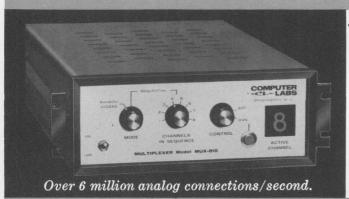
The Computer Labs Model MUX-810 Multiplexer will connect eight analog inputs to a single output at a rate of 6.6 million connections every second. Channels can be connected sequentially, with any number in the sequence; random access; or manually, with a front panel push button. Equivalent "ON" resistance is 0.2 ohm, making the Model MUX-810 an ideal choice for switching 100-ohm lines. Price includes one-year warranty and manual.
