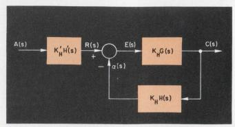
1. The distortion in signal R(s) is corrected by the inverse filter at the right. The feedback transfer function of the filter is a replica of the tranducer's.
