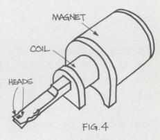
The unit in figure 4 is an application of the magnetic circuit in figure 3 above. It positions magnetic heads in computer disk drive systems. Both electrical and optical position sensing are employed to achieve extremely high resolution.
