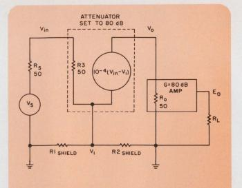
1. Gain equals attenuator setting when  $V_{\rm in}=E_{\rm o}$  in this standard test setup. The attenuator is shown in equivalent circuit form.
