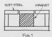
Figure 1 shows the magnetic circuit with highest efficiency. The magnet forms the center pole with a soft steel plate on the gap end. Leakage is 1.5 to 1.8. Operating density of the
