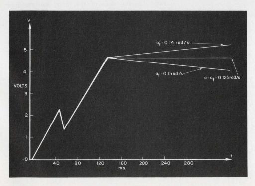
3. Incorrect choice of low-frequency breakpoint in the filter has this effect on signal restoration: The top curve shows the error resulting from too high and and the bottom curve from too low a choice. The correct curve is in the center.
