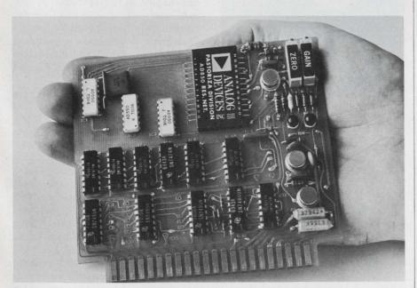
**Precision 12-bit analog-to-digital converter** offers a relative accuracy of 0.0125%. The unit uses monolithic weighted switches and a thin-film resistor network in its d/a section to achieve ultra-stable performance.
