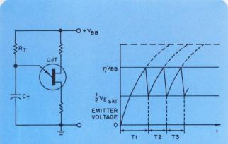
1. Basic UJT oscillator never fully discharges timing capacitor  $C_{\rm T}$  during each cycle. This allows the first period after turn-on to be longer than all others.
