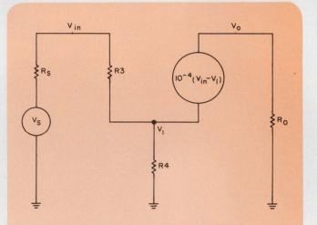
2. Parallel cable shield resistances are redrawn as  $\rm R_4$  to simplify circuit analysis. An  $\rm R_4$  of only 0.001  $\Omega$  can cause a 1.6-dB error when measuring 80 dB.
