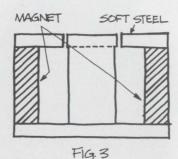
The circuit in figure 3 provides long coil excursion, high gap density —
