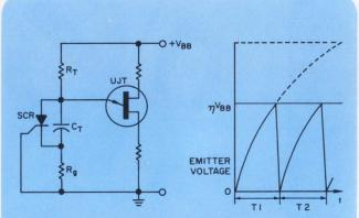
2. Improved UJT oscillator uses an SCR to completely discharge  $C_{\rm T}$  during every cycle. All periods are now of equal duration.
