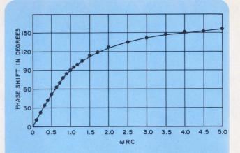
2. Linear phase shift exists over the first 60° of phase adjustment. A wideband transformer allows operation from 1 MHz to 100 MHz.
