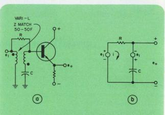
1. Constant-amplitude phase lag is provided by this hookup (a). Interchanging R and C provides phase lead. Equivalent circuit is shown in (b).
