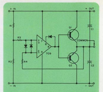
These dual outputs track with both source and load variations. This is an advantage over the typical dual configuration where reference voltage is derived from the positive supply only.
