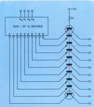
Common base buffer provides an output interface for the one-of-ten decoder.
