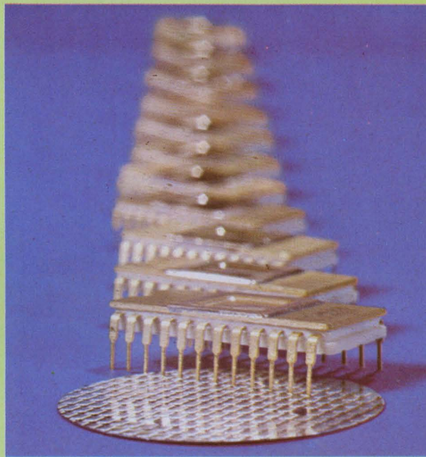
Read-only memories are customized by final metalization. (National Semiconductor Corp. photo)
