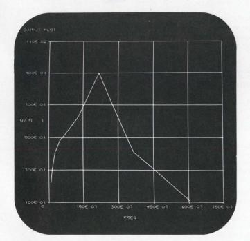
17. Here L=80  $\mu$ H, and the resonance is more pronounced. Note that, although the frequencies to be plotted are logarithmically related, the frequency scale is linear. ECAP does not plot frequencies on a log scale.
