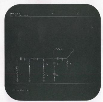
9. Branches 7 through 11 are added in a similar fashion. Branches 4, 5, 7, 8, 9, and 11 represent the equivalent circuit of the transistor without showing the gain as yet. The hybrid-pi transistor equivalent is used.
