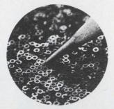
Five new memory cores for your next stack or system. All are medium or high drive, all coincident current, and all are fast switching for your high speed applications. Four new cores available in 18 mil, 20 mil, and two types of 30 mil sizes for use from 0° to 70°C. Also, a new wide temperature range 18 mil core for severe environments of —55° to +100°C.
