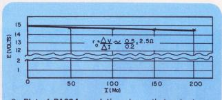
2. Plot of PA234 regulation shows that output resistance is several ohms.
