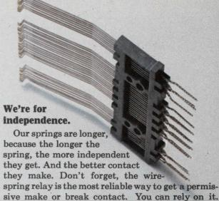
The middle contact springs have to be stationary. To make sure they stay that way forever, we actually mold them between two thick pieces of DAP on both ends. Just try to move one.
