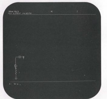
7. The next branch begins at the upper node of the first branch, and after selection of a 5  $\mu$ F capacitor the display looks like this.
