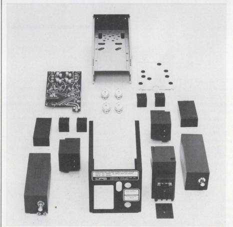
**Dynamic-focus CRT supply** can modulate high voltages from dc to 100 kHz. This compact unit delivers an output of 1 to 5 kV at 2 mA. It is constructed of interlocking epoxy blocks with no soldered connections.
