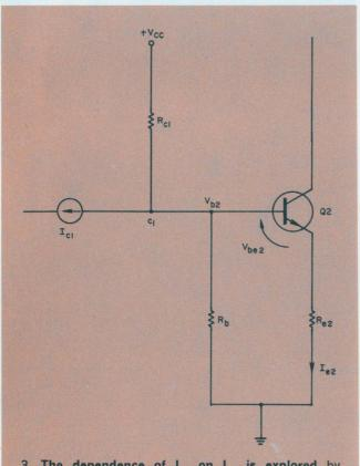
3. The dependence of  $l_{\rm c1}$  on  $l_{\rm c2}$  is explored by means of this circuit model. The expression for  $l_{\rm c2}$  as a function of  $V_{\rm be1}$  and  $V_{\rm be2}$  is differentiated with respect to  $V_{\rm be1}$  and  $V_{\rm be2}$  to yield the stability factors  $\delta_{\rm c}/\delta_{\rm be1}$  and  $\delta_{\rm c}/\delta V_{\rm be2}.$
