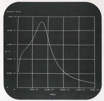
18. The frequency response is repeated here with a frequency multiplier of 1.08, which gives about 100 frequency steps. L=80  $\mu$ H. Compare this with Fig. 17.
