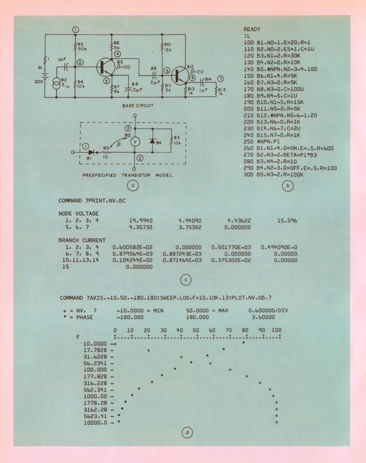
2. RECAL'S modeling capability includes the use of diodes. (a) shows a circuit with a transistor model that uses diodes. (b) is the input data for this circuit. (c) is a print output of the dc node voltages and branch currents. (d) is an output plot of the voltage at node 7,
