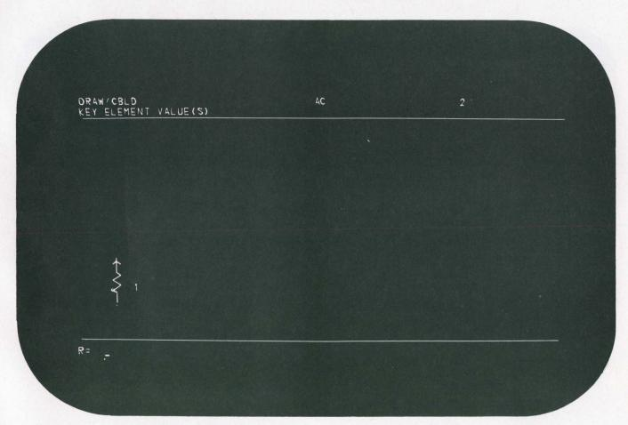
3. After a resistor is selected for branch 1, the display looks like this. The terminal requests a value for the resistor, and the user enters the value using the keyboard.
