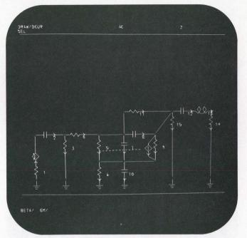
11. A dependent current link can now be inserted. By detecting FINISH ROUTINES on the previous display, we are asked to SEL FROM BRANCH (select the "FROM" branch), whereupon the user detects branch 5, and SEL TO BRANCH (select the "TO" branch), whereupon he detects branch 9. A dependent current now appears across branch 9 with a dotted line to branch 5. A menu choice is given between BETA and GM for expressing the dependence of branch 9.
