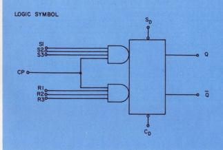
2. Two AOI gates form a gated latch. From the sequence table we note that the latch may be set when the S inputs are ONE ( $C_{\rm P}$  may be considered an S input) or reset when the R inputs are ONE, and that direct inputs  $C_{\rm D}$  and  $S_{\rm D}$  operate with logic ZERO levels. The truth table and logic symbol are derived from the sequence table. The gated latch is useful for general storage applications, where a full master-slave flip-flop is not required.
