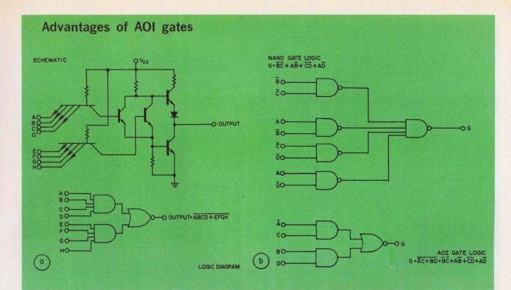
The AND-OR-INVERT (AOI) gate has three very important advantages over the NAND gate in TTL arrays. An LSI logic array of AOI gates typically uses 20 to 30% less silicon area, has 30% lower delay, and uses 20% less power than the equivalent function using NAND logic.
