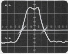
features: a tangential sensitivity of -85 dBm, frequency range of 400 kHz to 130 MHz, direct readout in dBm, and a calibrated reference line for swept operation.
