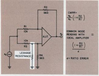
2. This CMRR test circuit requires careful matching of resistor ratios  $R_1/R_2$  and  $R_3/R_4$ , but leakage effects make close matching difficult. Matching error must be less than 0.01% for the circuit to be practical.
