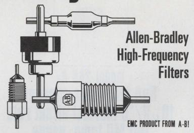
These miniature low-pass filters have been specifically designed for use in demanding EMC applications, where the necessary attenuation of undesired high frequencies cannot be obtained with conventional feed-thru capacitors. Attenuations of 75 db or more can be obtained in the frequency range of 50 MHz to 10,000 MHz.
