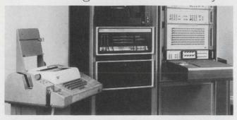
Picker uses its J259 to test circuit boards going into x-ray generators. The J259 whips through the 70 or 80 tests required on a board in a split second, automatically typing out the results of any test that is failed. Test data on a rejected board then accompanies the board to trouble-shooting, where a technician refers to his copy of the test program and keys the failed test to the bad component or connection.
