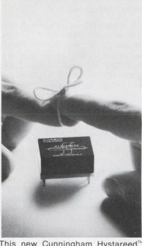
This new Cunningham Hystareed™ Magnetic Latching Relay operates without permanent biasing magnets or holding currents. Latches and stays latched. Won't change its programmed state because of vibration, shock, power interruptions or transients. Needs no adjustment or calibration. Available with up to six form A's, or four form C's in a single assembly. Operates as standard relay for scanning.
