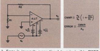
3. Error is inversely proportional to gain in this CMRR test circuit, which limits its usefulness to op amps with comparatively high gain  $(1\times10^6)$  and low CMRR  $(1\times10^5)$ .
