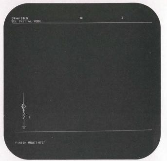
6. By detecting the bottom node with the light pen, and then GROUND from a new series of menu items (not shown here) a ground symbol appears. NEW BRANCH is then detected from the menu items, and this display then appears where the instruction, SEL INITIAL NODE at the top, calls for the initiation of a new branch.
