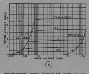
Optoelectronic control element LD<sub>1</sub> holds the output of the agc amplifier (a) at a constant level over a 74-dB input voltage range (b).
