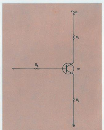
4. The stability of  $l_{\rm e2}$  over temperature is indicated quantitatively by Eq. 21. It describes this simplified input stage in which all circuitry is reduced to Thevenin equivalents connected to the input transistor.
