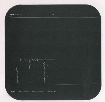
8. The circuit is built up to this point, branch by branch. Here wire extensions that make the diagram more legible are shown at either node of branch 5. The menu items at the bottom of the display are the passive element choices available, and when detected by the light pen are next to appear on the CRT.
