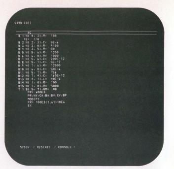
14. A display of the input data is now asked for. The computer replies with conventional ECAP language listing as shown here. The results of the print (PR) statement will not be shown. The originally chosen frequency (FR-600E3) is changed by the MODIFY statement to cover the range 100E3 to 10E6.
