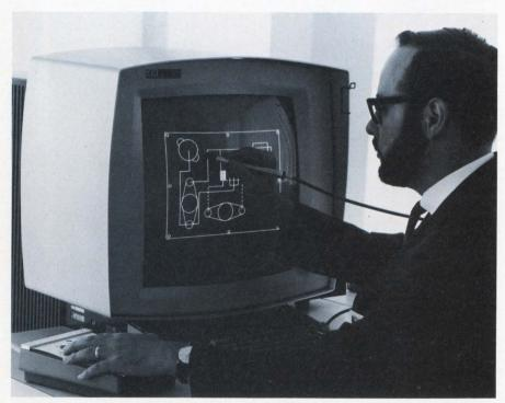
**Circuit-board layout** is checked out with a light-pen-actuated graphic console by Norman Schweitzer, a staff engineer at TRW Systems.
