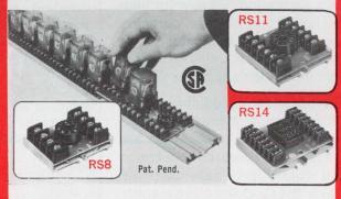
Octal socket assembly for 8 pin 2 P.D.T. relays. Assembly 2" long. Rated: 10 amps, 250 volts.
