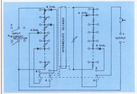
By using the same voltage divider resistor ladder for both A and B measurements, the potentiometer achieves an accuracy of 1 part in 100 million since deviations of the ladder's accuracy are kept common to both A and B.
