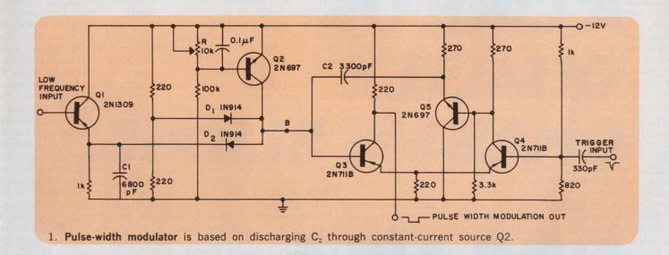
ly until it becomes negative enough to make Q3 conduct again. This marks the end of the output pulse, and the multivibrator returns to its stable state.
