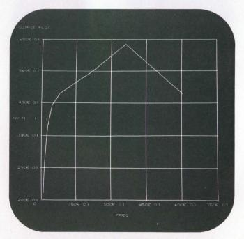
15. The computer plot of the voltage across branch 14 has approximately 14 frequency steps as a result of the choice of the frequency multiplier=1.67. The inductor of branch 13 is used as a parameter to vary the peaked frequency response. Here L=  $20~\mu\text{H}$ . The computer automatically selects the vertical and horizontal scales so the curve fills the screen.
