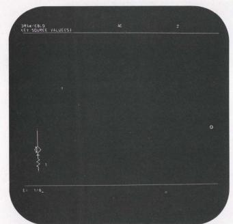
5. The computer requests the value of the voltage source, and the user keys in 1.0 V at zero phase.
