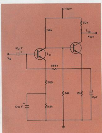
5. A current-feedback pair amplifier using a 2N2060B dual transistor has an Ic2 drift of about 88 nA/°C, only a 4.5% change from the 250  $\mu\text{A}$  collector current from 25°C to 150°C. The kHz voltage gain is 76 dB.
