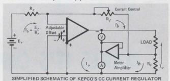
Dynamically, CC regulators are unrestrained by the usual large shunt output capacitor of conventional voltage sources. This means that a change in load resistance will produce an immediate response in the load voltage without waiting for a capacitor to charge! It also means that when you short the output (the proper way to idle a current source), you no longer need worry about a current surge from the output capacitor. No capacitor, no surge.
