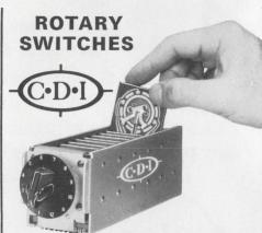
For critical reliability applications. Meet MIL-S-22710. Removable wafers permit quick changing of programs, configurations, circuits. CDI patented switches with dust covers available in sizes 2" x 2", 3" x 3" and 4" x 4" with lengths to accommodate up to 36 wafers. Operation may be manual, motor or solenoid.
