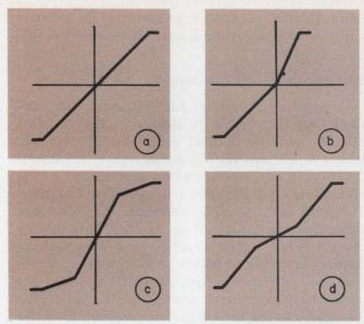
1. The dc transfer characteristics of op amps are seldom ideal, as in the linear transfer curve (a). Practical op amps have asymmetrical positive and negative gain (b), a decrease in gain near their output swing limits (c), a decrease in gain near zero output level (d), or a combination of these.
