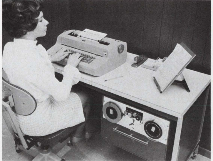
Typewriter-to-magnetic-tape recording system can be operated by non-EDP personnel, see p. 120.
