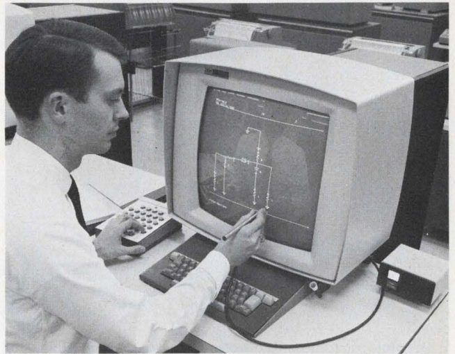
4. Designer uses light pen to select components from a list of options shown at the lower area of the screen.
