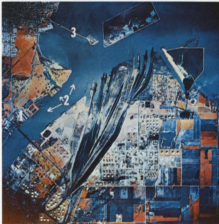
Solar infrared color aerial photograph shows distribution of pollutants in Maumee Bay, Lake Erie. The sewage plant (1) discharges effluent (2) into Maumee Bay, which is trapped behind the recently built breakwater (3). (Photo courtesy of NASA).
