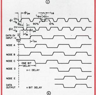
2. The dynamic shift-register cell contains six MOS transistors. Information is shifted within the cells when  $\Phi 1$  goes negative (turning on devices Q3, etc.) and is shifted between cells when  $\Phi 2$  goes negative (a). The data is clocked out of the register during the  $\Phi 1$  clock time, n-clock-periods after data entry, where n is the size of the register in bits (b).
