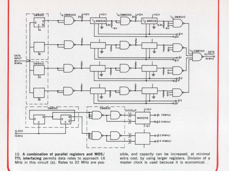
The maximum data rate that can be achieved by paralleling registers is about 32 MHz at present. The limit is imposed by the speed with which TTL circuits can detect and reassemble the outputs of the parallel registers. Today's TTL circuits can commutate data down to easily acceptable MOS register clock rates.
