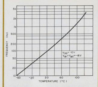
4. The minimum operating frequency of a dynamic register depends on its operating temperature. The dynamic cell does not have a feedback latch and must depend on charge-storage for retention of data. Leakage resistance, directly proportional to temperature, limits the storage time—and hence imposes a minimum operating frequency.
