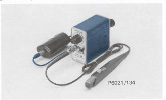
The P6021 AC Current Probe and Type 134 Amplifier provide the facility for accurate current measurements over the wide range of 12 Hz to 40 MHz without breaking the circuit under test. Used with any plug-in unit having a deflection factor of 50 mV/div, the P6021/134 provides deflection factors from 1 mA/div to 1 A/div.
