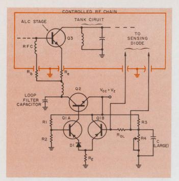
6. A wide dynamic range is achieved with only a single-polarity power supply by using an npn transistor for Q2 and a pnp pair for Q1. Diode D1, in the emitter leg of Q1A, provides linear temperature compensation for the control circuit, and  $R_{\rm e}$  sets the bias level of the alc stage.
