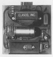
The LIC5-1A power supply is designed for mounting either on a chassis or in a 5½" IC Basket. As many as 9 units can be mounted in a standard Elasco basket.
