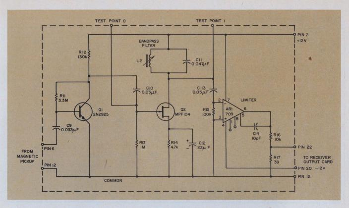
3. The receiver input circuit provides noise rejection and limiting of the tie signals received on the telephone lines.
