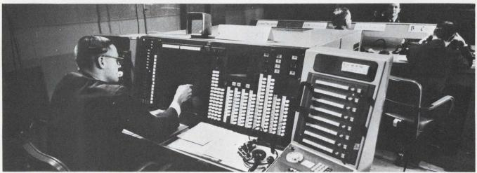
Display for Back-Up Interceptor Center (Buic III), which would replace a bombed-out Sage air defense network, shows twice as much
