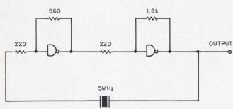
Highly accurate clock can be built from two linearized gates and a crystal.
