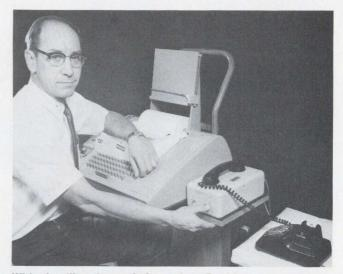
With the flip of a switch, author Roubique converts his teletypewriter into a time-shared terminal that operates over conventional telephone lines.
