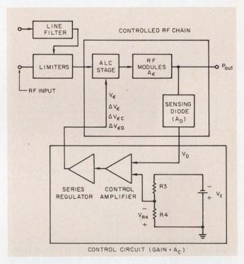
2. Automatic level control is provided by a saturated rf amplifier whose output is controlled by varying its supply voltage.
