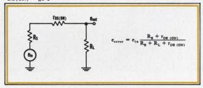
OFF CONDITION: Static OFF error voltage is extremely small due to low drain leakage current, ID(OFF). AC feedthrough is low since drain-to-source capacitance, Cds, is always less than 0.4 pF.
