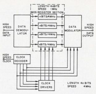
9. Clock rates can be multiplied by paralleling registers and using data modulators and demodulators. Data can enter and leave this line at 4 MHz, while individual registers are clocked at only 1 MHz. This system can be expanded.
