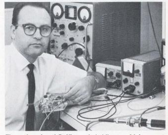
The author, Arpad D. Vincze, is holding a  $\times 24$  frequency multiplier/rf amplifier chain.
