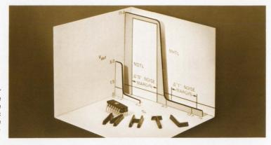
The transfer curves on the right illustrate the large logic swing available from MHTL compared with MDTL.
