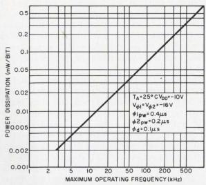
5. Power dissipation increases with operating frequency in a dynamic register, because a current path between supply and ground exists only during the time that one of the clock phases is in the negative state. Since the clock pulse width is held constant, the clock duty-cycle—hence power dissipation—increases with frequency.
