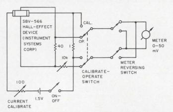
Hall-effect device produces an output voltage that is proportional to the strength of the magnetic field it is measuring.
