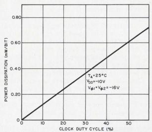
6. The dynamic register-cell dissipates power only when the load resistor is clocked ON. If the clock-pulse duty-cycle is lowered, power dissipation is decreased, so the narrowest possible clock should be used. A typical cell will dissipate the same power at 100 kHz with 1.0  $\mu$ s clock pulses as it will at 10 kHz with 10.0  $\mu$ s clock pulse.
