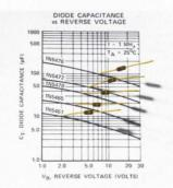
The slopes of capacitance change vs.voltage are the same for all types in the 1N5461 Epicap tuning diode series.
