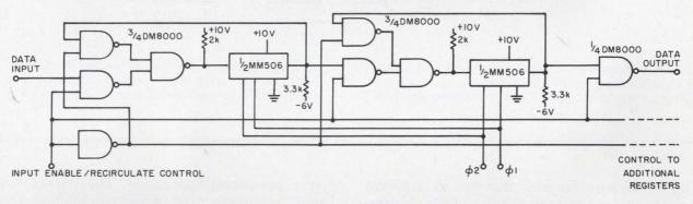
8. TTL interfaces lower register loading and improve output detection, allowing higher register
