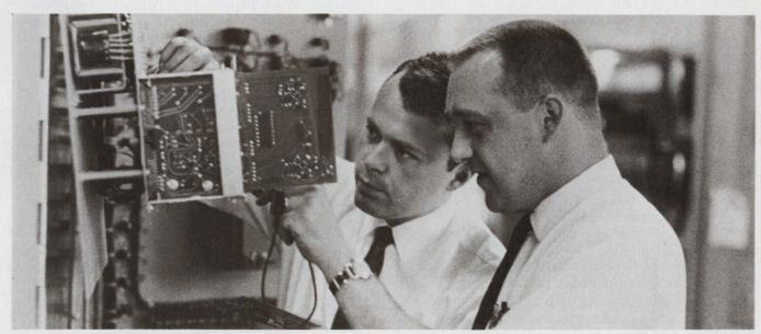
Authors Randall (left) and Ritchey check the control circuitry in an SCR static power rectifier.
