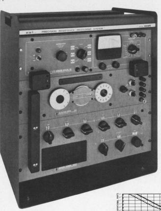
The 242C is simple enough for batch testing on a GO-NO-GO basis (meter deflection without bridge adjustment). Or if you prefer to read percent deviation from nominal value, you do so with a one-dial adjustment. Then when the perfectionist has a need, he can resolve actual value of a resistor to 10 places (with 8 decades plus a vernier). And when calibrated against ESI standards, comparisons can be made to 0.1 ppm with accuracy directly traceable to the National Bureau of Standards.
