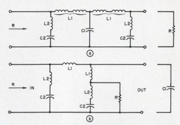
A low-pass T-section with m-derived terminations makes up the low-pass filter network (a). Rearrangement of the network shows the input and output terminals (b).
