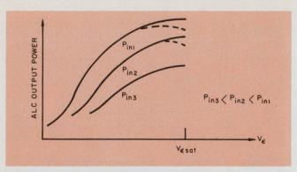
3. The alc stage transfer characteristics are plotted for different values of input power. Note that as the supply voltage gets high enough to pull the amplifier out of saturation, the output power may dip (dashed lines) if the amplifier Q is too high.
