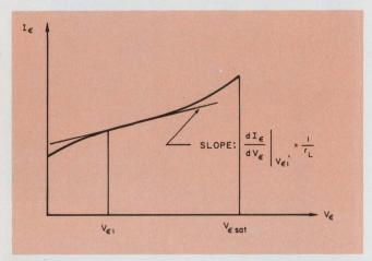
5. The incremental input resistance of the alc stage can be found from this plot of  $l_{\epsilon}$  vs  $V_{\epsilon}$ . The resistance is the reciprocal of the slope of the curve.
