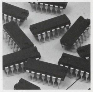
Two up/down counter chips, binary and decimal, rep to 30 MHz, p. 108.
