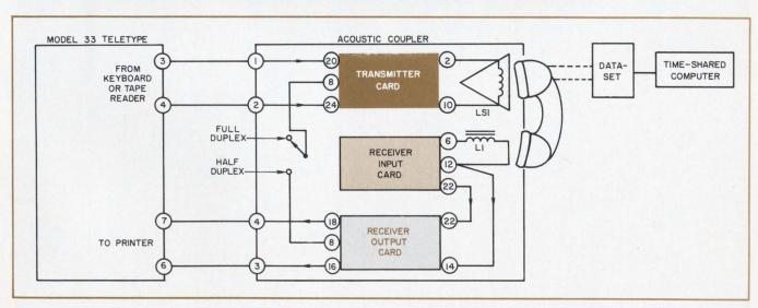
1. Acoustic coupler converts a teletypewriter into a timeshared computer terminal. The transmitter portion of the coupler converts the dc signals from the teletypewriter
