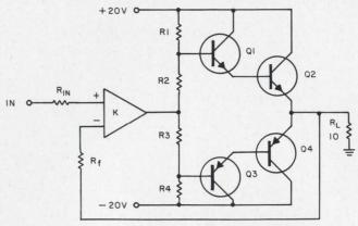
2. Q1 through Q4 are complementary Darlington pairs. They can boost the output of a low-current operational amplifier to well over 1 A.
