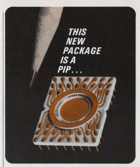
It's a 40-pin Plug-in-Package (PIP) from the Cermetron Division of National Beryllia—30% lighter, and with 8 to 10 times the thermal conductivity of similar packages using other materials, because it is made from BERLOX—Beryllium Oxide.
