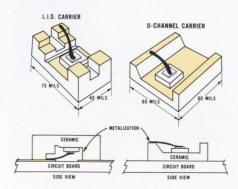
Zener diode "chips" can be supplied on metalized ceramic U-channel and L.I.D. carriers (as well as unmounted), to satisfy most any Hybrid thick or thin-film circuit mounting and fabrication requirement.
