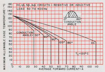
1. Power dissipation in an SCR, and therefore the allowable case temperature, is dependent on the conduction angle. The curves shown are for the G.E. series C52 SCRs, and are based on a sinusoidal current waveform.
