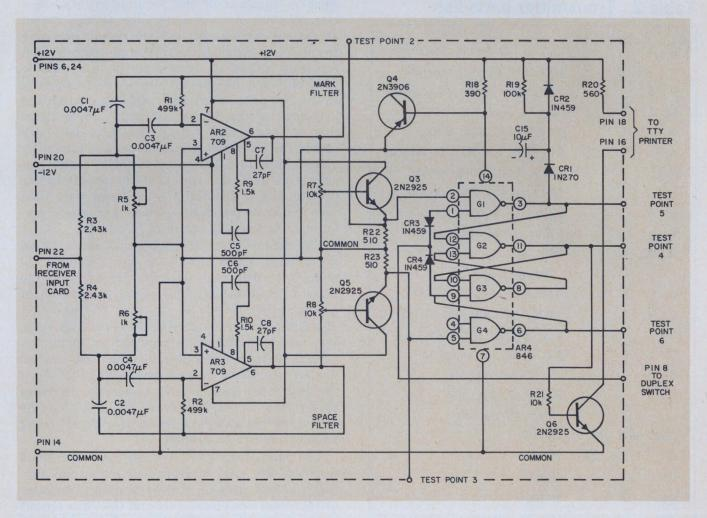
4. The receiver output circuit converts the frequencyshift tone signal into the ON-OFF dc currents required by a teletypewriter. The circuit uses two IC operational amplifiers and one digital IC.
