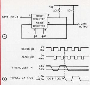
1. A dual dynamic register is series-connected to make a simple 100-bit delay line (a). Data clocked to the register input appears 100-clock-pulses later (b) at the output.
