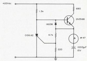
Flashing occurs each time the capacitor discharges through the turned-on SCR. When the discharge current falls below the SCR holding current, the SCR turns off, and the capacitor begins charging for another cycle.
