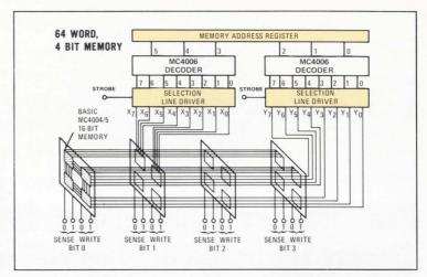
Decoders and 16 MC4004/5's are needed to form a complex, yet compact system such as this 64-Word, 4-Bit Memory.
