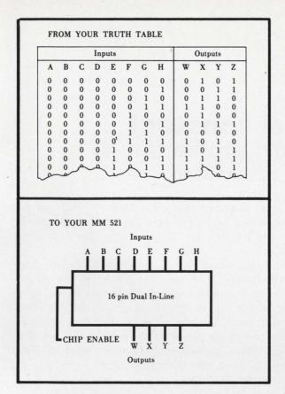
Use the logic easily programmed into our ROM (Read Only Memory) elements. With a minimum of time (typically four weeks), we can set up the simple interconnection metalization pattern your needs dictate and start shipments. Costs about a thousand dollars.
