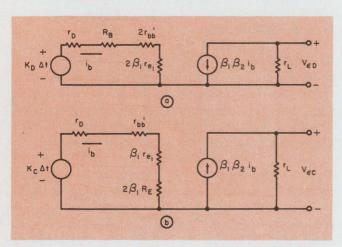
8. The linear drift behavior of the control circuitry is analyzed with these equivalent circuits. Separate models are needed for differential-mode drift (a) and common-mode drift (b).  $R_{\rm B}$  is the equivalent parallel resistance of  $R_{\rm 1}$  and  $R_{\rm 2}$  of Fig. 6.
