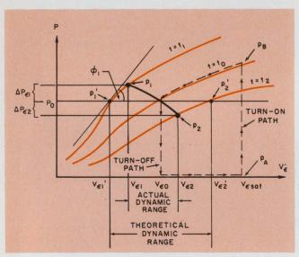
4. The effect of temperature on the output of the rf chain can easily be seen in this plot of output power vs error voltage for three different temperatures. The reference temperature is  $t_{\rm o}$ ;  $t_{\rm 1}$  is below  $t_{\rm o}$ , and  $t_{\rm 2}$  is above it. The dashed line shows the turn-on/turn-off locus. The solid black line is the locus of normal operation.
