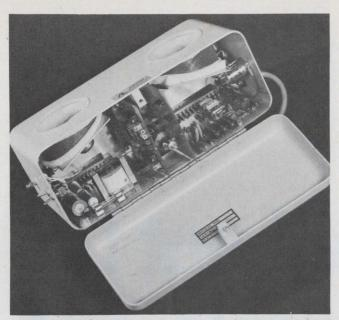
Compact packaging is easy due to the relative simplicity of the coupler circuitry. The two receiving boards are mounted vertically in the center, while the transmitting board is at the lower right. The power supply, which must provide a +12 V and a -12 V at a current of 100 mA, is at the lower left.
