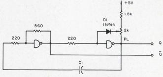
4. Square-wave generator with complementary outputs can be varied in frequency over a wide range.
