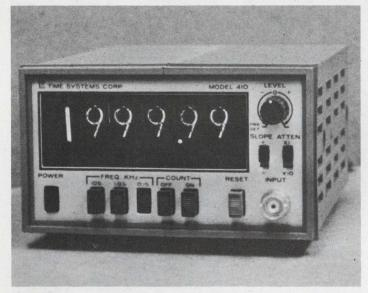
**Low-frequency counters** in 3 by 4.9 by 6-3/4-in. package can be remotely programed, p. 118.
