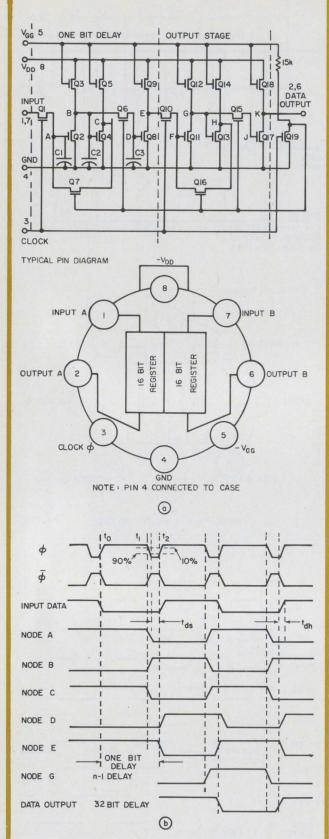
3. Each static shift-register cell contains nine transistors in an Eccles-Jordan feedback-latch configuration (a), with Q6 and Q7 acting as cross-coupling resistors. Information is transferred between cells on the clock pulses via Q1 and Q10 (b), and is transferred within cells on the complementary clock pulses  $(\bar{\Phi})$ , which are generated internally. The static register will store bits indefinitely, even if the clock is interrupted.
