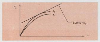
7. Stay away from the flat portion of these sensing diode curves. The flattening is caused by reverse breakdown of the diode. The curves are shown for two temperatures,  $t_{\rm o}>t_{\rm l}$ .
