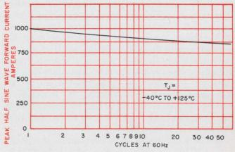
2. The peak forward surge current,  $I_{\rm fm}$ , of an SCR must be derated if the peak current is to be conducted for more than one half-cycle.
