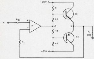
1. Push-pull emitter followers Q1 and Q2 boost the output current from the operational amplifier. The circuit can deliver  $15\ V$  to a 100-ohm load.
