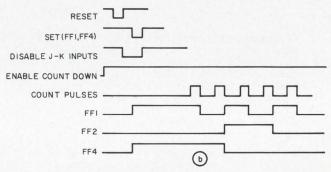
of standard logic blocks. Timing waveforms are shown for counting down from binary 101 (b).
