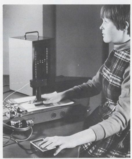
To use the Bliss-Linvill portable tactile reading aid, the operator moves the probe along the line of print and feels a bundle of stimulator pins vibrating in the shape of the letters. The light display box is used for visual trouble-shooting.
