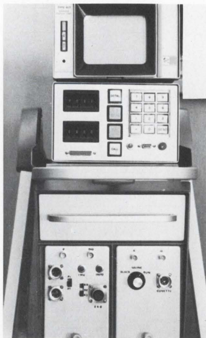
The remote terminal unit used in the Utah network. Note the compactness of the unit and the simplicity of the controls.
