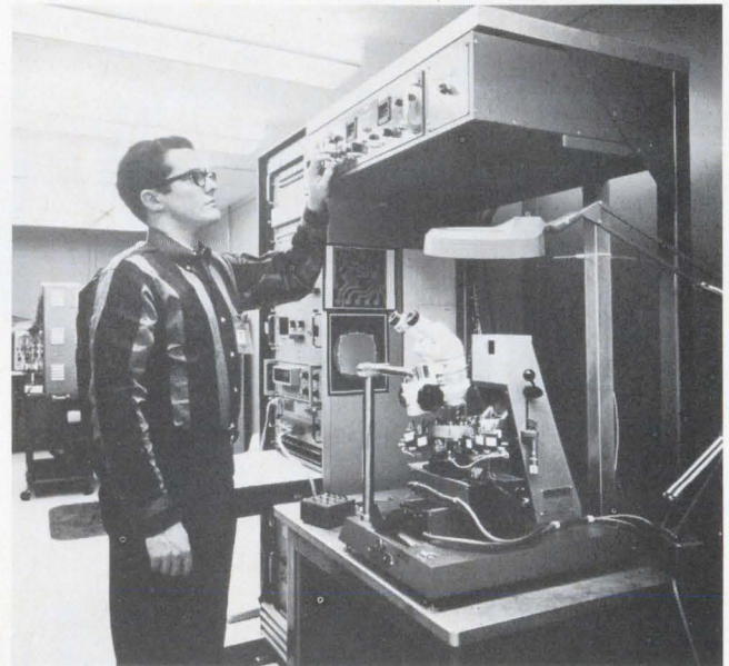
6. The automatic probe-test equipment rapidly and accurately determines which circuits on a slice are good and which are defective. The data are fed to a probe processing program.
