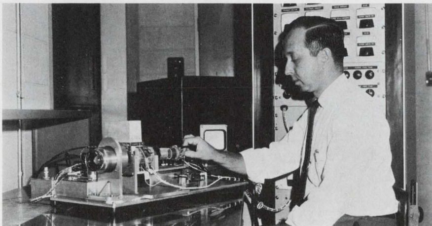
GE's TV camera system, designed with a Focus, Projection, Scan Vidicon, has a resolution of 2200 TV lines per inch. The goal is 10,000 lines.
