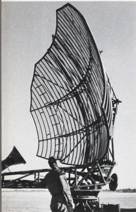
Antenna of the AN/TPS-44 search radar collapses, making the lightweight system air transportable in two neat modules.
