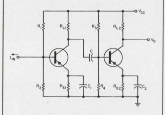
The combined cascaded network derived in connection with Fig. 6 can be applied to the analysis of this amplifier circuit. The transistor is a 2N1925, a pnp germanium, general-purpose, medium-power device. The *h* parameters obtained from the data sheet and typical values are:
