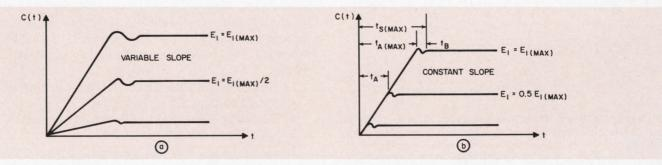
4. Both positioning time,  $t_A$ , and settling time,  $t_s$ , are functions of the yoke voltage  $E_1$ . Ideal deflection ampli-
