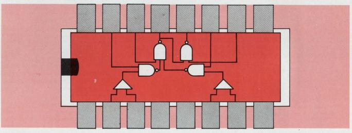
Six IC sense amplifiers designed to operate with TTL or DTL circuitry, detect bipolar dif-
