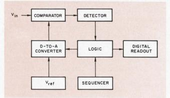
2. Successive approximation is faster, but still noisy. The system performs a "forced null balance" by a continued series of comparisons and detections.
