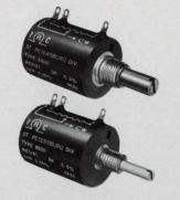
High performance and long life at lowest cost. 10 turns,  $\frac{7}{6}$ " diameter with only  $1\frac{1}{6}$ " behind the panel. 2 watts @ 25°C., derates to zero @ 105°C. 100 $\Omega$  to 100K, with all popular intermediate values.  $\pm 5\%$  tolerance and  $\pm 0.25\%$  linearity. Side terminals accept to #14 wire. Model 8400 has  $\frac{3}{6}$ "-32 bushing,  $\frac{1}{4}$ " shaft. Model 8500 has  $\frac{1}{4}$ "-32 bushing,  $\frac{1}{6}$ " shaft.
