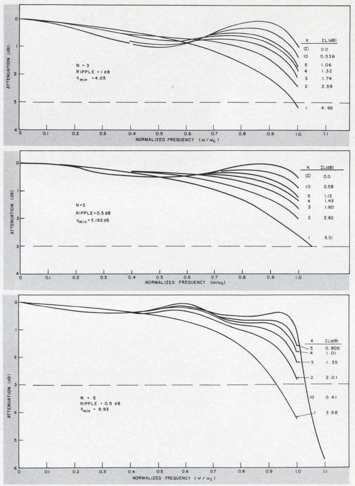
9. Curves for Chebyshev filters show attenuation for third- and fifth-order types and several ripple factors as
