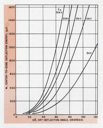
2. **Deflection energy** required for the display CRT can be determined from this plot, once deflection angle and the CRT anode voltage are known.
