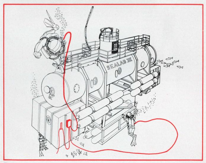
The Navy Sealab III base will be placed on the sea floor 600 feet down. Aquanauts will be tethered with a cable
