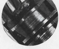
Brush assembly of conventional synchro after 1000 hours
