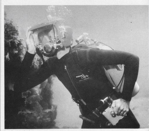
**Bendix AN/PQC-2** acoustic phone for Sealab III can transmit voice, code or homing signals more than 1500 feet. An 8.5-to-11-kHz modulated carrier is sent and received by a piezoelectric ceramic transducer on the underside of his belt-mounted case. Aquanauts will wear similar fiberglass helmets.
