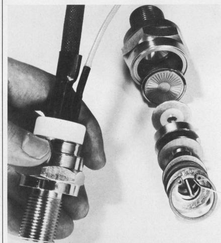
**Compression-bonded encapsulation** is what holds this transistor's junction in place. This technique eliminates soldering and uses spring pressure.
