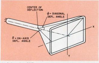
1. Only a few CRT parameters are required to calculate the over-all display system components.
