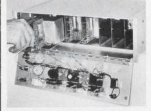
Seven plug-in circuit boards make up the diffusion furnace controller.
