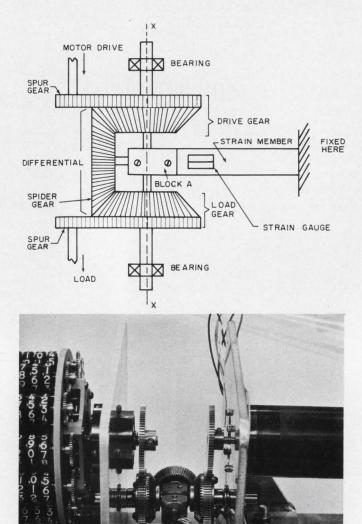
Simple and accurate torque sensor is built with a differential and a stationary strain member. An actual test set up is shown in the photo.
