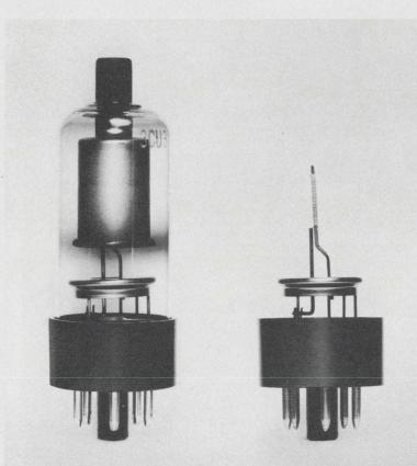
New Sylvania 3CU3, above, contrasted with our 3A3A high-voltage rectifier with cathodetype construction. Note simplicity and ruggedness of posted filament design in 3CU3.
