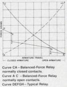
method of getting rid of a bounce condition is to balance the armature forces exactly. This is achieved in the
