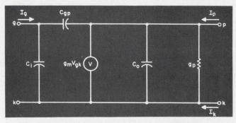
3. Equivalent circuit of a pentode helps establish the appropriate floating admittance matrix. One matrix is sufficient to describe all modes of operation.
