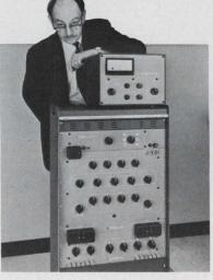
ESI makes available a family of standards and transfer standards to complete the System, including our proven 10k resistance standard. Although optional if you already have satisfactory standards for comparison and transfer, our Model 104 Transportable Resistance Standard (instead of a Thomas 1-ohm) is a keystone to achieving full performance with the 123 Comparison System. Circle No. 163 on your reader card.
