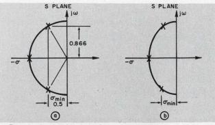
1. Roots of transfer functions for Butterworth filters lie on a unit circle (a) in the S-plane. For Chebyshev types, they are on an ellipse (b). The minimum Q of a low-pass filter is the reciprocal of  $\sigma_{min}$  for both types, which is the real part of the root nearest the j $\omega$  axis.
