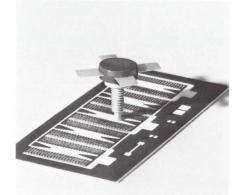
The Balanced Emitter Technology (BET) protects against the development of "hot spots" by providing nichrome resistors in series with each emitter, to facilitate an even current distribution throughout the entire transistor structure.
