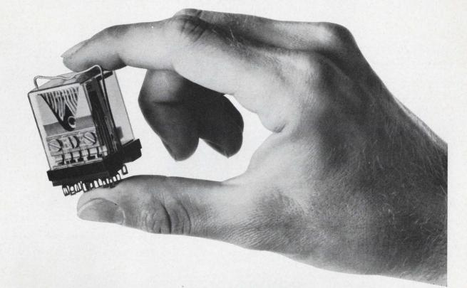
The Class H relay is small in size—just about a 1.3 inch cube. It's a versatile "telephone-type" component that offers better than average quality at a low price.
