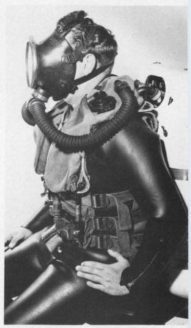
Navy diver wears semi-closed circuit breathing apparatus. Umbilical cable attaches to fitting on his right side. No communication or telemetry equipment is shown. signal and sends it to a waterproof encapsulated bone-conduction phone that is fitted under the diver's neoprene helmet.
