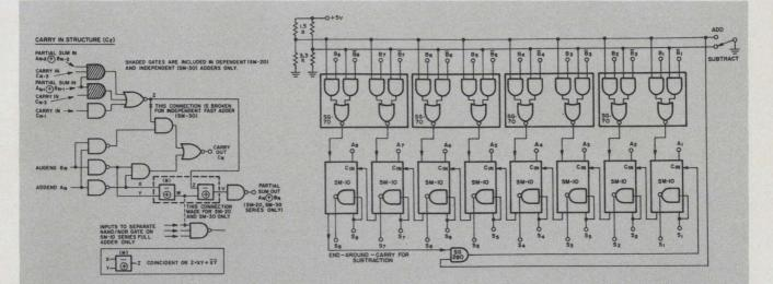
Figure 1. Logic diagram for a single parallel adder stage
