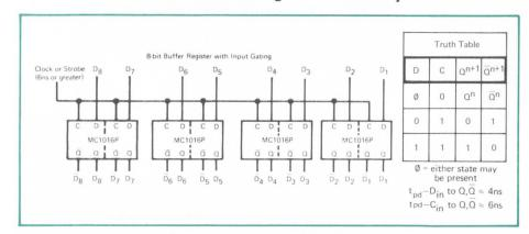
Here's an easier, less-complex and less-expensive way to construct an 8-Bit Buffer Register *using just four dualfunction MC1016P MECL II integrated circuits!* These new dual R-S flip-flops reduce can-count (and system cost) by doubling the number of functions per package.
