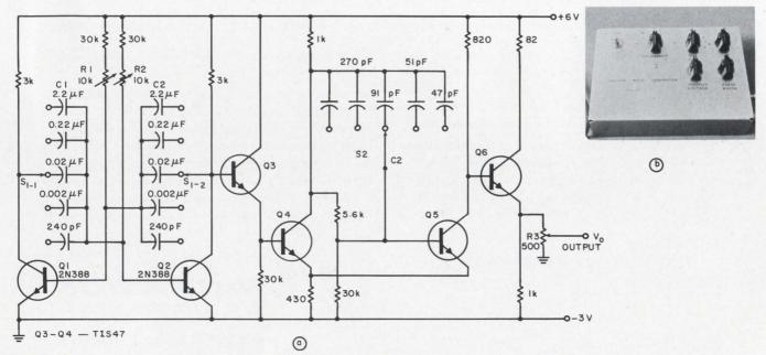
**Rise times down to 20 ns** are obtained from the square wave generator (a). It can be housed in a small, inexpensive aluminum chassis (b). It can be operated either on batteries or off an external power supply.
