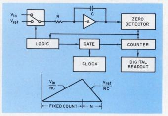
6. Dual-slope integration is accurate, fast, and quiet. Long-term accuracy is high, since shifts in C are compensated for by shifts in  $V_{\rm ref}/RC$ . Even if the clock frequency varies, the reading will remain correct.
