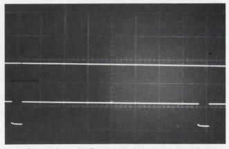
**Long-duty-cycle multivibrator** (top) uses only one discrete component, C<sub>T</sub>. Upper trace (bottom) is the set pulse, lower trace is the output pulse. Horizontal scale is 500  $\mu$ /cm, vertical is 5 V/cm.
