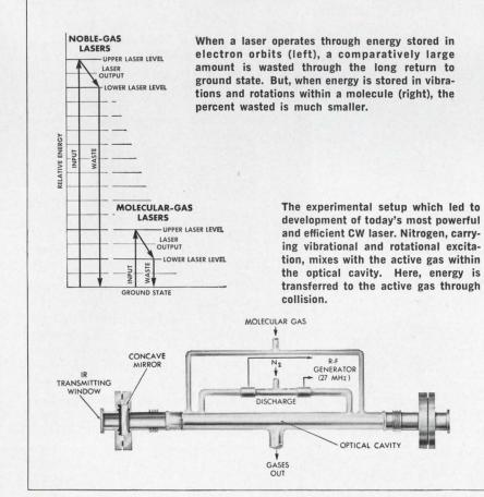
To produce a photon in a gas laser, an atom or molecule reduces its energy by dropping from the "upper laser level" to the "lower laser level" (graph). From the lower level, the energy usually decreases to absolute minimum— "ground state"—before the atom or molecule can emit another useful photon. This second drop is waste: incoherent light and heat.
