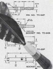
of giving you very high density puck ing of contacts on .050" centers. (That's up to 420 contacts per square inch.) We've been able to do this by removing the standard contact spring member and replacing it with a breathing helical spring.
