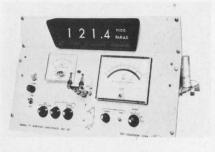
25-kW dummy load weighs 11 pounds
