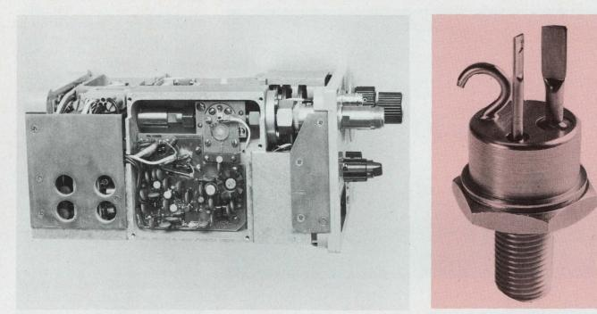
**Transfer oscillator plug-in** has a frequency range of from 50 Hz to 18 GHz with a sensitivity of -4 dBm. Page 128
