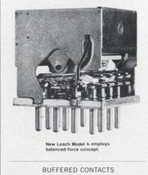
The moving contacts are mounted to an armature, which is held firmly at the end of each stroke by high magnetic forces. Since the armature can't move during shock
