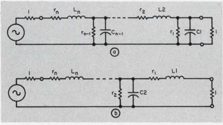
2. Two standard low-pass filter configurations are used in most designs. For even-order types, (a) is used as the standard circuit, and for odd-order ones, (b) is the usual circuit. The resistances  $r_n$  compensate for copper and core losses.
