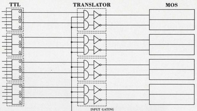
New DM7501 dual JK flip flop used as a TTL shift register for an 8-bit word.
