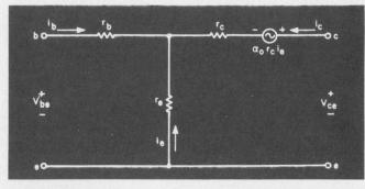
5. Deletion of the appropriate row and column from the floating matrix, based on Fig. 4, establishes the commonemitter configuration.
