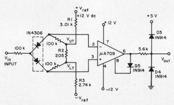
High-impedance window discriminator is built with a single  $\mu$ A709 and a few precision resistors.
