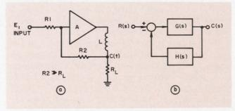
3. Ideal deflection amplifier (a) and its servo model (b) required to drive the yoke. L is the yoke inductance,  $R_{\rm L}$  is the yoke resistance.
