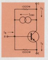
6. The eight-parameter transistor model is described by considering the transistor as two diode junctions. Npn is shown; for pnp the direction of the currents is reversed.
