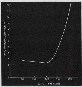
5. Total harmonic distortion at 1 kHz is less than 3% over the design power output range (300 mW). The gain of the amplifier under these conditions is 44 dB and the input impedance is  $3 \text{ k}\Omega$ .
