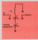
8. In a varactor-tuned cavity, where the diode may be in series with the line, the cavity consists of a capacity-loaded open-circuit line. The varactor and its associated inductance terminates the other end of the line. Inductive input and output couplings are used.
