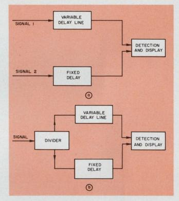
6. **Typical applications** of variable delay lines occur in crosscorrelators (a) and autocorrelators (b). There the major requirement is wide bandwidth.
