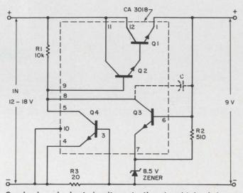
**Overload and short-circuit protection** is obtained in a simple voltage regulator by using Q4 and  $R_3$  to limit the output current to just under 30 mA.
