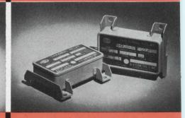
The PT Series relays provide the most precise performance available in thermal relays. Meet the exacting military requirements for reliability under extreme operating environments. Features:  $\pm 5\%$  tolerance over a temp. range of  $-55^{\circ}$ C to  $+125^{\circ}$ C; 2000 Hz vibration; 50g shock; time delays, 3 to 180 sec.; heater voltages, 6.3, 28 and 115V. AC or DC.
