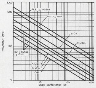
4. The diode's frequency limits depend on the type of package and lead length. The limit is determined by a 10% decrease of  $Q_A$ . Parallel resonant tuning, where the inductance degrades the Q by more than 10%, is not recommended.
