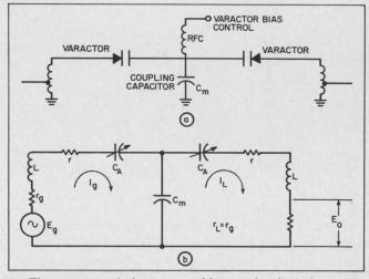
7. The varactor inductance adds to circuit inductance, hence response of circuit is not degraded. The coupling capacitor,  $C_{\rm e}$ , can be replaced by a varactor for wider tuning range (a). In its equivalent circuit (b), it is assumed that the circuit coupling is adjusted for  $r_{\rm L}=r_{\rm g}$ , and is otherwise symmetrical.
