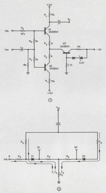
1. **Transformerless chopper (a)** uses a differential amplifier (Q1, Q2) and a constant-current source (Q3). The circuit action is explained in (b).
