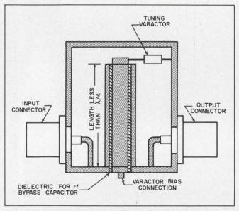
5. In a varactor-tuned coaxial cavity, the cavity length should be less than  $\lambda/4$ , so that the cavity impedance is inductive at the varactor terminals. The diode's capacitance resonates with the inductance at the mean frequency.
