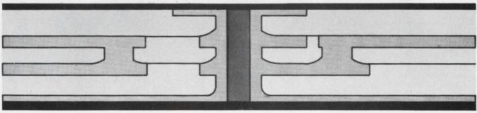
A wiring board in multilayer form uses a solid post technique that will allow dual-in-line ICs to be surface mounted. Holes may also be drilled through the posts. Page 148
