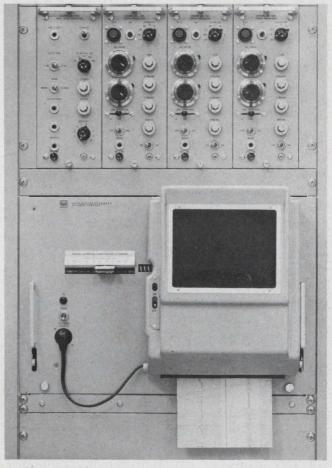
2. Photographic-paper processing can be sped up with a rapid-developing adapter. Such recordings exhibit very high contrasts and lend themselves well to duplication by any standard method.
