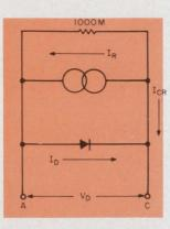
4. Simple models are used by CIRC. The diode model has three parameters and is easily specified from the manufacturer,s data. The shunt resistor is needed for CIRC mechanization.
