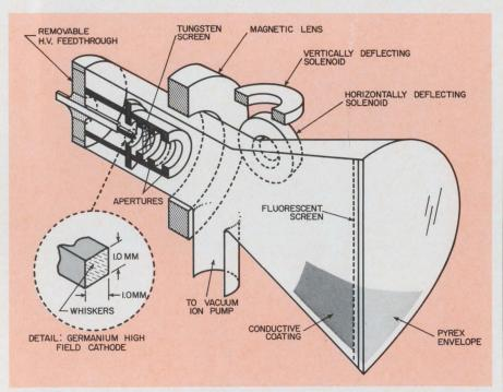
**High field cathode** in demonstration cathode-ray tube needs no heater. Cornell University device gives 1 A/cm<sup>2</sup> electron emission density from novel whiskered cathode in the parallel plane diode structure.
