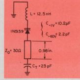
9. Equivalent circuit of a varactor-tuned cavity covering from 470 MHz to 890 MHz uses the values calculated in the text. The given values for  $C_{\rm T}$ ,  $Z_0$  and L, and a Smith chart permit calculation of the 1N5139 capacity values:  $C_{\rm max} = 11.1$  pF and  $C_{\rm min} = 2.35$  pF.
