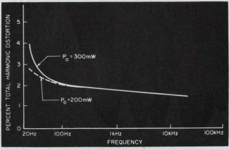
6. Total harmonic distortion as a function of frequency for two values of output power is under 4% at 25 kHz and 300 mW.
