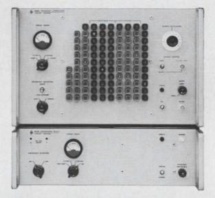
The new Hewlett-Packard 5105A Frequency Synthesizer generates spectrally pure frequencies from 0.1 MHz to 500 MHz in 0.1 Hz steps—a frequency range 10 times higher than previously available by direct synthesis.
