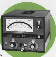
RMS responding • Built-in rechargeable battery (optional model for line only) • Isolated signal ground • DC output of 0.1 - 1.0 V for each 10 dB range for application to recorder or DVM where output is proportional to mean square of input ac voltage. • PRICES: Model 323 (Battery/line) \$520; Model 323-01 (line only) \$485.
