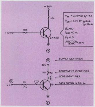
1. At the starting point of a CIRC analysis the engineer takes his circuit design (a) and numbers each element and node (b). This simple example has two nodes but CIRC can handle fifty.
