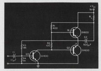
1. **Generalized complementary-symmetry amplifier** schematic includes three transistors. In this case Q1 and Q3 are a matched complementary pair of silicon epoxy transistors (GI 600) and Q3, the driver, is an epoxy GI 400. Note that each output transistor sees only a maximum of one-half the supply voltage. All values are computed in the design example.
