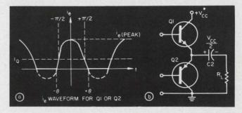
4. **Transistor power dissipation** is computed by means of an equivalent circuit (b) and its current wave (a).
