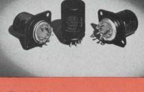
The LT Series relays provide hi-level performance in a subminiature hermetically sealed housing — space saving without loss of performance. Meets military standards. Features: height above mounting panel 40% of standard relays (7 pin flange mount); time delays, 2 to 75 sec.; operating temp.,  $-65^{\circ}$ C to  $\pm 85^{\circ}$ C; operating voltages, 6.3 to 115V. AC or DC.
