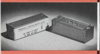
The JT Series is the only thermal relay designed to mount directly on pc boards without need for adapters or sockets. This design conserves space, reduces weight, allows greater packaging densities for pcb's. **Features:** time delays,-2 to 180 sec.; contacts, SPST, NO or NC; heater voltages, 6.3 to 230V. AC or DC; temperature compensated; operates in any position.
