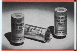
Metal enclosed thermal time delay is dust proof and shatter proof — designed for industrial applications requiring reliable operation and long life. **Features:** temp. compensated; time delays, 2 to 180 sec.; heater voltages, 6.3, 26, and 115V. AC or DC; contacts, SPST, NO or NC. Recognized Under The Components Program Of Underwriter's Laboratories, Inc.
