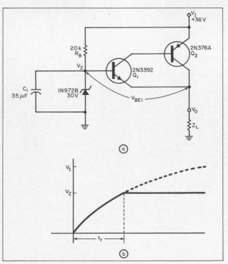
**Slow build-up** of output voltage is obtained (a). The delay time is about 2 seconds (b).
