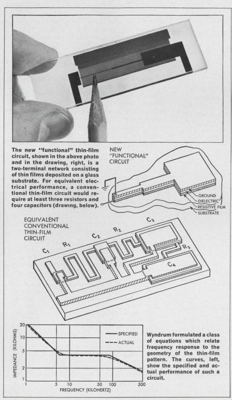
As electronic systems have grown in size and complexity, tantalum integrated circuits have reduced costs while increasing reliability and performance. To obtain even further integration of circuit functions, however, engineers at Bell Telephone Laboratories have used tantalum technology to build single thin-film components equivalent to networks of thin-film resistors and capacitors.
