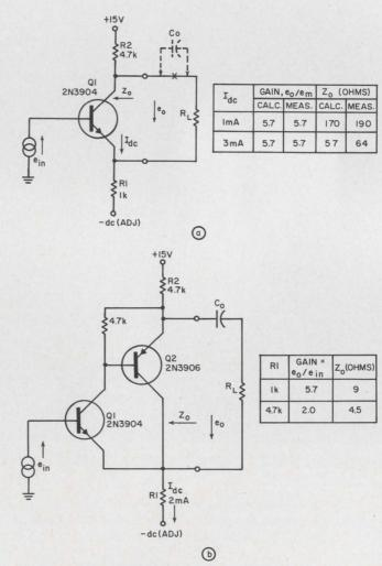
1. Low output impedance is obtained in circuit (a) when  $R_{\rm L}$  is connected across the transistor. Note effect of operating current  $I_{\rm dc}$  on the  $Z_{\rm o}.$  Two-transistor version (b) has much lower  $Z_{\rm o}.$  Note the effect of gain.
