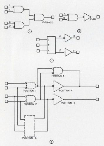
1. One printed-circuit board (d) can be used for three logic functions (a, b, c) by placing ICs in proper positions. Function (a) is obtained by leaving positions 4, 5 and 6 empty; (b) by leaving positions 3 and 6 empty; (c) by leaving 1, 2 and 3 empty.
