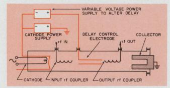
4. **Traveling-wave delay lines** are basically modified TWTs. As a delay line, the TWT circuit is severed and has a drift space that changes the beam velocity. The delay depends on the potential and the length of the drift region in the tube.
