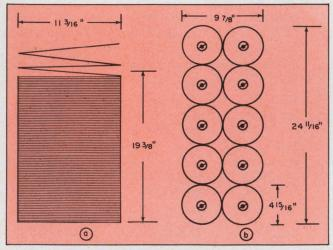
1. **Z-fold paper saves space.** Five thousand feet of Z-fold (a) stand 19-3/8-inches tall; a comparable amount of roll-fed paper (b) takes over 40% more space. Z-fold records are easily accessable; roll-fed is unraveled foot by foot.
