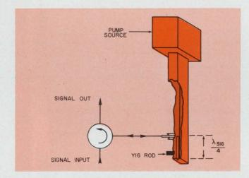
3. Parametrically pumped solid-state delay line needs large rf pump powers: typically greater than 20 watts in S band. They offer large variations in delay times: up to 20  $\mu$ s was reported.
