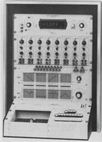
**Dc analysis of ICs** with up to 40 pins can be handled by this tester. Dynamic testing with a sampling scope is available as an option.
