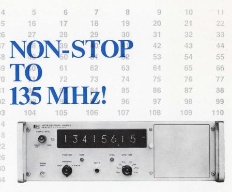
PLUS—ultra-stable, fast warm-up time base PLUS—plug-in measurements to 18 GHz PLUS—versatility as a frequency standard PLUS—100 mV to 10V input range without adjustment
