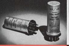
Instant reset during or after timing is available by combining G-V's unique instant reset timing element with a magnetic relay. Widely used in communication systems and data processing equipment. **Features:** delay time, 2 sec. to 5 min.; ambient operating temp., 32°F to 185°F.
