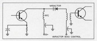
6. Series resonant tuning permits the varactor inductance to be added to tank circuit inductance, thereby raising the possible operation frequency.
