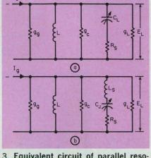
3. Equivalent circuit of parallel resonant tank circuit may omit the varactor's inductance (a). Its inclusion (b) leads to a more accurate analysis.
