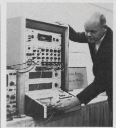
**Dynamic testing** is performed by Computer Test Corp. tester by connecting a sampling oscilloscope to an internal pulse generator.
